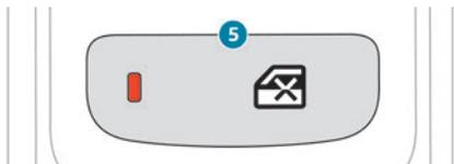
For your children's safety, press control **5** to deactivate the controls for the rear electric windows, irrespective of their positions. The red indicator lamp in the button comes on and a confirmation message is displayed. The lamp will remain lit until the controls are reactivated.
