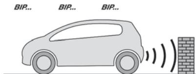
The system signals the presence of obstacles within the sensors' detection zone.
