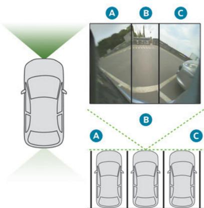
The 180° view assists with exiting from a parking space in forward gear, making it possible to see the approach of vehicles, pedestrians and cyclists.
