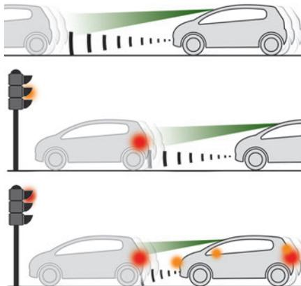
This function, also called automatic emergency braking, intervenes following the alerts if the driver does not react quickly enough and does not operate the vehicle's brakes.
