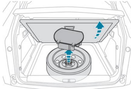
The spare wheel is stored in the boot, under the floor.
