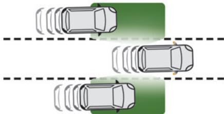
This system warns the driver of a potential danger posed by the presence of another vehicle
