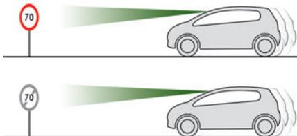
This system displays the maximum speed authorised locally on the instrument panel, using:
