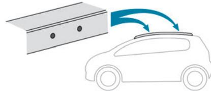
The transverse bars must be fixed at the markings located on the longitudinal bars.
