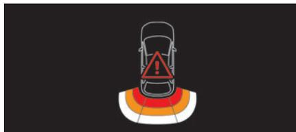
This supplements the audible signal by displaying bars on the screen that represent the distance between the obstacle and the vehicle
