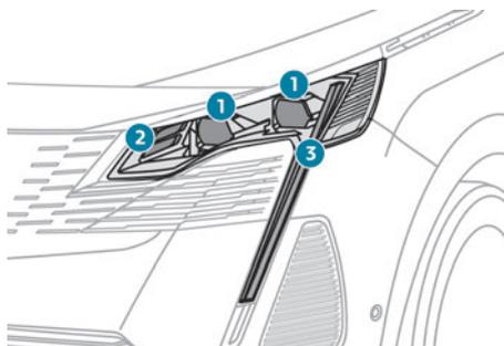
1. Dipped beam headlamps/Main beam headlamps
