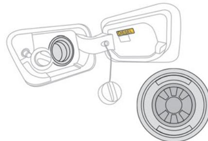
When a petrol filler nozzle is introduced into the fuel filler neck of a Diesel vehicle, it comes into contact with the flap. The system remains closed and prevents filling.
