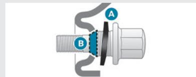
If the vehicle is fitted with alloy wheels, the washers **A** do not make contact with the steel or "space-saver" type spare wheel. The wheel is held in place by the conical contact surface **B** of each bolt.
