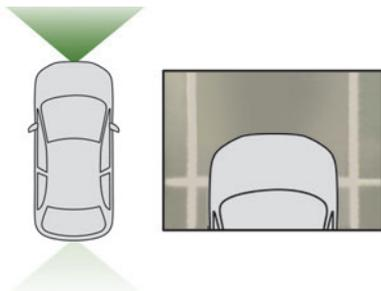
The camera records the vehicle's surroundings during the manoeuvre in order to create a view from above the front of the vehicle in its near surroundings, allowing the vehicle to be manoeuvred around obstacles nearby. This view is available with AUTO mode or in the view selection menu.
