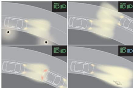
**!** This system is a driving aid. The driver remains responsible for the vehicle's lighting, its correct use in the prevailing light, visibility and traffic conditions, and for compliance with driving and vehicle regulations.
