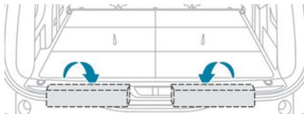
Some of the tools are stored beneath the floor against the boot sill.
