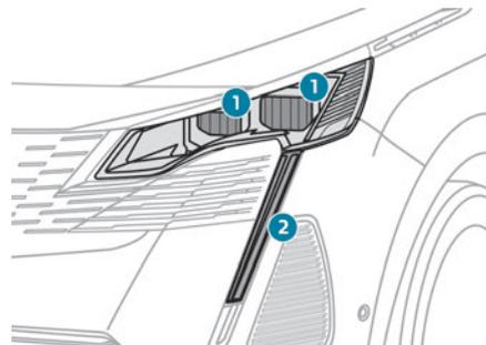
1. Dipped beam headlamps/Main beam headlamps
