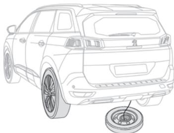
The spare wheel is held by a winch system underneath the rear of the vehicle.
