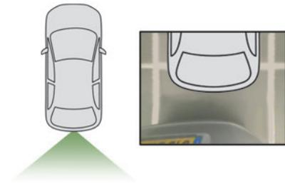
The camera records the vehicle's surroundings during the manoeuvre in order to create a view from above the rear of the vehicle in its near surroundings, allowing the vehicle to be manoeuvred around nearby obstacles. This view is available with AUTO mode or in the view selection menu.
