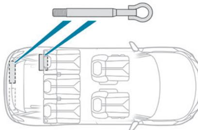
Depending on version, the towing eye is stored either in the interior trim of the boot sill, left-hand side, or in a bag behind the left-hand rear seat.
