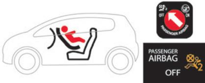
! The front passenger airbag must be deactivated before installing a rearward facing child seat. Otherwise, **the child risks being seriously injured or killed if the airbag is deployed.**
