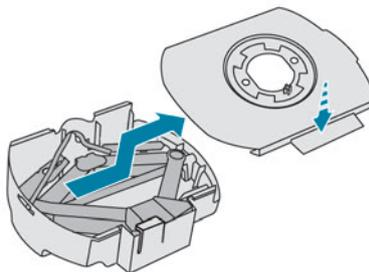
The tool box is installed at the centre of the spare wheel beneath the vehicle. It contains the jack and the wheel bolt cover removal tool.
