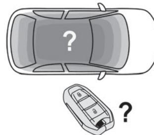
If the electronic key is not detected or is no longer in the recognition zone, a message appears in the instrument panel when closing a door or trying to switch off the engine.
