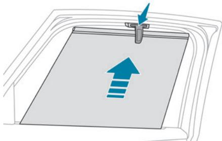
Fitted to the second row windows, they protect the passenger compartment from the sun's rays.
