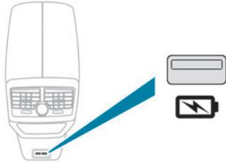
Each USB socket is used only to power or recharge a portable device.
