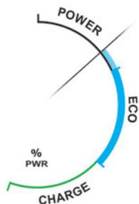
**POWER** High power demand, using the combined capabilities of the petrol engine and the electric motor(s) (depending on version).
