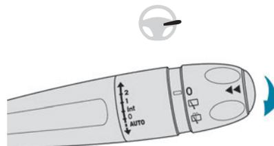
► To select the wiping speed: raise or lower the stalk to the desired position.
