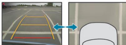
This mode is activated by default. Using sensors in the front bumper, the automatic view changes from the front view (standard) to the view from above (zoom) as an obstacle is approached during a manoeuvre.
