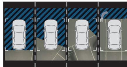
Using one or two cameras, the close surroundings of the vehicle are recorded whilst manoeuvring at low speed.
