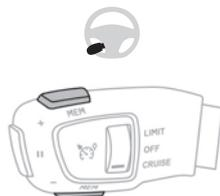
With this button, you can select a memorised speed setting to use with the speed limiter or the programmable cruise control.
