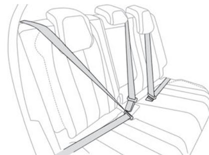
Each of the rear seats has a three-point seat belt with inertia reel.
