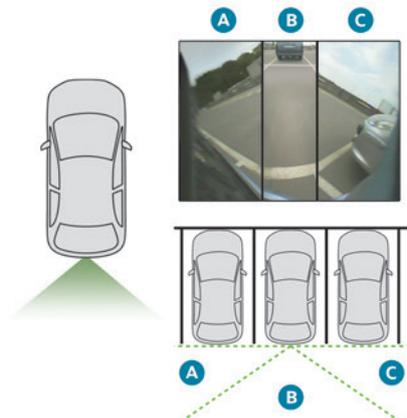
The 180° view facilitates reversing out of a parking space, making it possible to see the approach of vehicles, pedestrians and cyclists. This view is not recommended for carrying out a complete manoeuvre.
