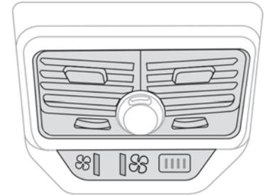
When this function is activated, the rear air vents blower starts up. In this case, the rear passengers can control the air flow from these air vents independently of the air conditioning air flow control for the front air vents.
