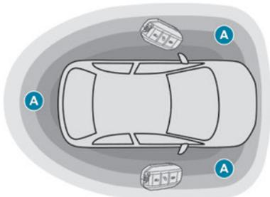
This system allows the unlocking, locking and starting of the vehicle, while carrying the
