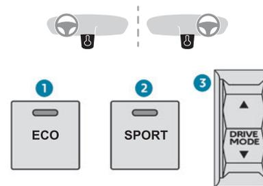
1. Pressing the control activates **Eco** mode. The indicator lamp comes on.
