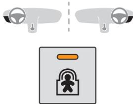
► With the ignition on, press this button to activate/deactivate the child lock.
