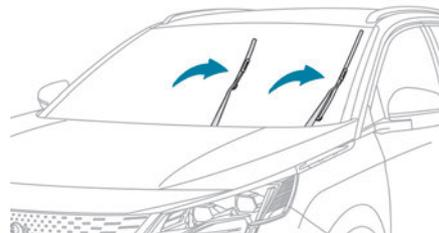
Operating the wiper control stalk within one minute after switching off the ignition will place the wiper blades in a vertical position.
