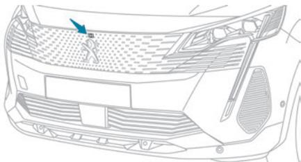
This system identifies and signals the presence of pedestrians and animals in the driver's field of vision, in low exterior light conditions, using an infrared camera located at the front of the vehicle.
