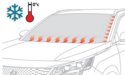
In cold weather, this system heats the bottom of the windscreen, as well as the area alongside the left-hand windscreen pillar.
