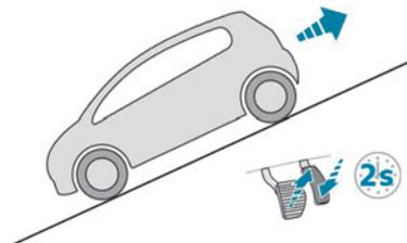
**Facing downhill, with the vehicle stationary and reverse gear engaged, the vehicle is held for a short time when the driver releases the brake pedal.**
