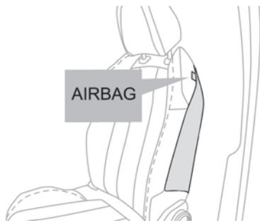
In the event of a serious side impact, this system protects the driver and front passenger to mitigate the risk of injury to the chest, between the hip and the shoulder.
