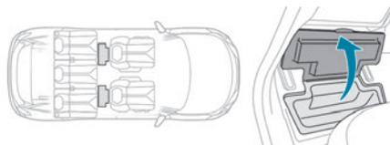
Depending on version, the storage boxes are fitted in the floor, at the foot of the side seats on the second row.
