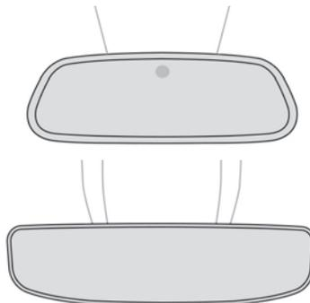
The electrochromic system uses a sensor that detects the level of exterior brightness and that coming from the rear of the vehicle, in order to automatically and gradually switch between day and night usage.
