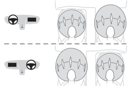
System that protects the driver and front passenger in the event of a serious front impact, limiting the risk of head and chest injury. The driver's airbag is fitted in the centre of the steering wheel; the front passenger airbag is fitted in the dashboard above the glove box.
