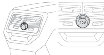
▶ To connect a 12 V accessory (maximum power: 120 W), lift the cover and plug in a suitable adaptor.
