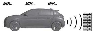
The system signals the presence of obstacles which are both within the sensors' detection zone and in the vehicle path defined by the direction of the steering wheel.
