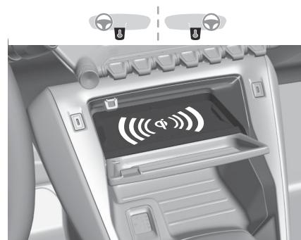
This system allows wireless charging of a portable device such as a smartphone, using the magnetic induction principle, in accordance with the Qi.
