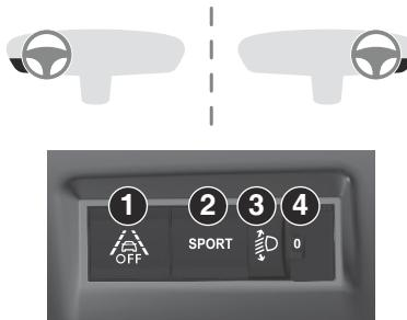
1. LED technology headlights beam height adjustment
