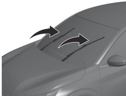
Operating the wiper control stalk immediately after switching off the ignition will place the wiper blades in a vertical position.
