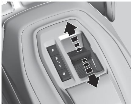
The drive selector is a pulse selector with a regenerative braking function.
