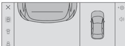
The front or rear camera records the surroundings during the manoeuvre to create a front or rear view from above the vehicle in its close surroundings, making it possible to manoeuvre the vehicle around the surrounding obstacles.
