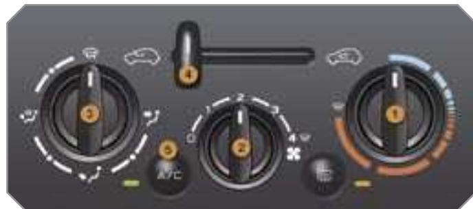
Control panel with manual control
