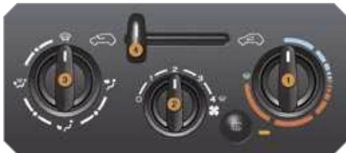
Control panel with manual control
