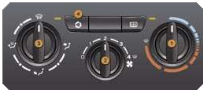
Control panel with electric control
