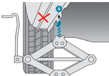
► Extend jack **6** until its head comes into contact with jacking point **A** or **B**; contact area **A** or **B** on the vehicle must be properly inserted into the central part of the head of the jack.
