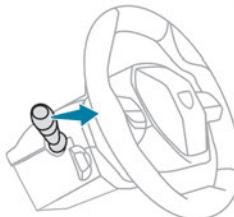
► With the ignition off, pull the lighting control stalk toward you ("headlamp flash") to activate/deactivate the function.
