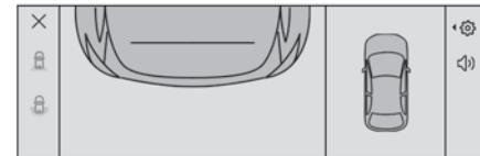
The rear camera records the vehicle's surroundings during the manoeuvre in order to create a view from above the rear of the vehicle in its close surroundings, allowing the vehicle to be manoeuvred around nearby obstacles.
