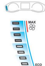
The gauge shows the consumption of the traction battery's electrical energy by the thermal comfort devices in the passenger compartment. With a digital instrument panel, the gauge only appears in "Personal" mode.
