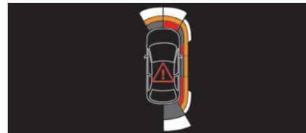
Using four additional sensors located on the sides of the bumpers, the system records the position of obstacles during the manoeuvre and indicates them when they are located alongside the vehicle.
