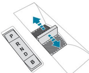
The drive selector is a pulse selector with a regenerative braking function.
