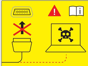
As a safety measure, access to the **diagnostic socket**, used for the vehicle's electronic systems, is reserved strictly for PEUGEOT dealers or qualified workshops, equipped with the special tools required (risk of malfunctions of the vehicle's electronic systems that could cause breakdowns or serious accidents). The Manufacturer cannot be held responsible if this advice is not followed.
