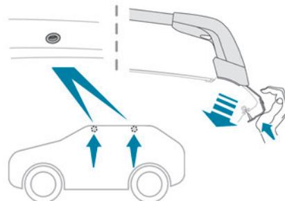
The transverse bars must only be fixed at the four anchorage points located on the roof frame. These points are concealed by the vehicle doors when the doors are closed.
