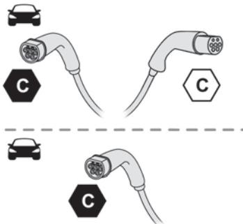
Identification labels **C** on the charging connector (vehicle side) and on the socket (charger side).
