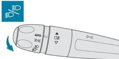
► Pull the lighting control stalk to switch between dipped and main beam headlamps. In lamps off or "AUTO" modes, depending on version, and in sidelamps mode, pull the lighting control stalk to switch the main beam headlamps on directly ("headlamp flash").
