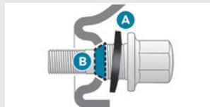
If the vehicle is fitted with alloy wheels, the washers **A** do not make contact with the steel or "space-saver" type spare wheel. The wheel is held in place by the conical contact surface **B** of each bolt.
