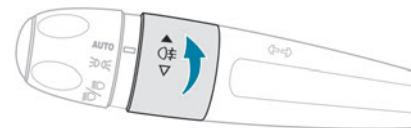
► Rotate the ring forwards/backwards to turn it on/off.
