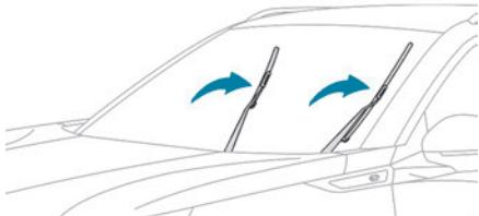
Operating the wiper control stalk immediately after switching off the ignition will place the wiper blades in a vertical position.
