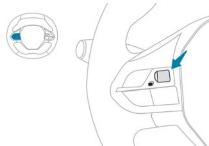
► Turn the thumbwheel on the left of the steering wheel to display and scroll through the various pages on the instrument panel.
