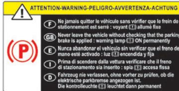
! Before leaving the vehicle, check that the parking brake is applied: the parking brake indicator lamps on the instrument panel and the control must be on fixed.
