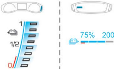
The traction battery's actual charge level and the remaining range are displayed continuously when the vehicle is started.
