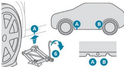
► Place the foot of jack **6** on the ground and ensure that it is directly below the front **A** or rear **B** jacking point on the underbody, whichever is closest to the wheel to be changed.
