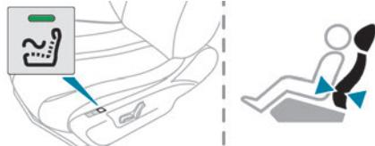
This function provides lumbar massage; it only operates when the engine is running as well as in STOP mode of the Stop & Start system.
