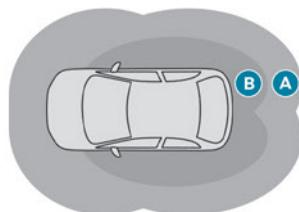
**Zone A:** automatic locking on moving away from the vehicle (about 2 metres from the vehicle).
