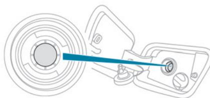
When a petrol filler nozzle is introduced into the fuel filler neck of a Diesel vehicle, it comes into contact with the flap. The system remains closed and prevents filling.
