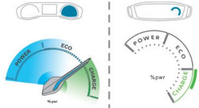
**CHARGE** Traction battery charging during deceleration and braking.
