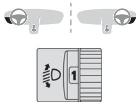
To avoid dazzling other road users, the height of the headlamp beams must be adjusted according to the load in the vehicle.
