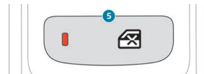
For your children's safety, ignition on or engine on, press control **5** to deactivate the controls for the rear electric windows, irrespective of their positions.
