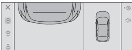
The front or rear camera records the surroundings during the manoeuvre to create a front or rear view from above the vehicle in its close surroundings, making it possible to manoeuvre the vehicle around the surrounding obstacles.
