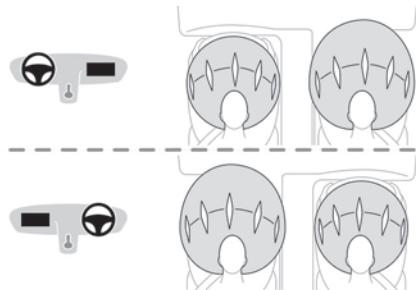
This system protects the driver and front passenger in the event of a serious front impact, limiting the risk of head and chest injury. The driver's airbag is fitted in the centre of the steering wheel; the front passenger airbag is fitted in the dashboard above the glove box.
