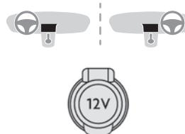
► Plug in a 12 V accessory (with a maximum rated power of 120 W) using a suitable adapter.
