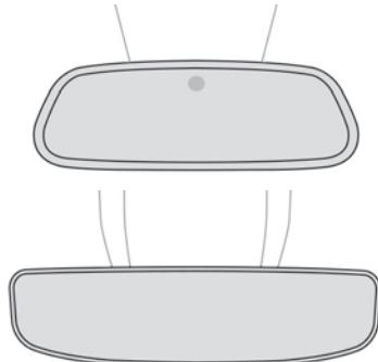
The electrochrome system uses a sensor that detects the level of exterior brightness and that coming from the rear of the vehicle, in order to automatically and gradually switch between day and night usage.
