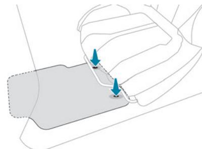
When fitting it on the driver's side, only use the mountings present on the carpet (a "click" indicates proper locking).
