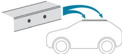
The transverse bars must be fixed at the markings located on the longitudinal bars.
