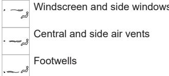
A symbol is activated to display the presence of blown air in the direction indicated.
