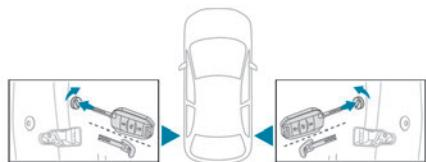
► To activate the child lock, turn the built-in key in the **red** control as far as possible:
