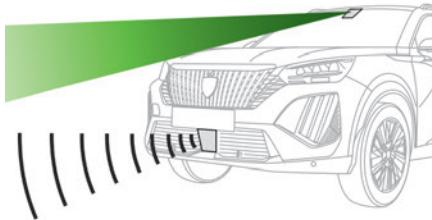
The vehicle has a multifunction camera located at the top of the windscreen and, depending on version, a radar located in the front bumper.
