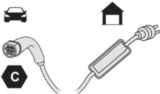
Identification label **C** on the charging connector (vehicle side).
