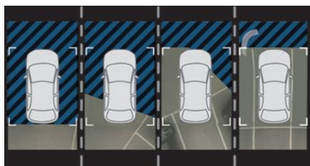
Using the camera, the vehicle's close surroundings are recorded during low speed manoeuvres.
