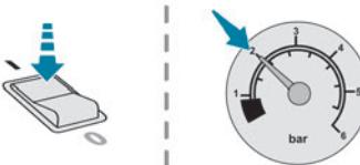
▶ Switch on the compressor by moving the switch to position "I" until the tyre pressure reaches 2 bar. The sealant product is injected under pressure into the tyre; do not disconnect the pipe from the valve during this operation (risk of blowback).
