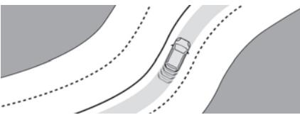
The system identifies the edges of the traffic lane and steers the vehicle to keep it inside this lane and maintain the lateral position chosen by the driver.
