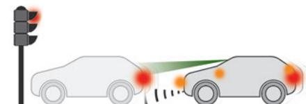
This function, also called "automatic emergency braking", intervenes after the acoustic alert if the driver does not operate the brake pedal quickly enough.
