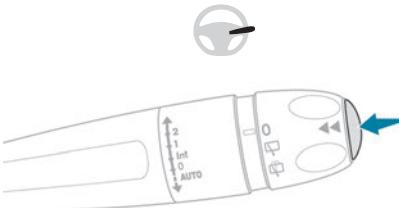
► Pressing the button located on the end of the wiper control stalk displays the following tabs in turn:
