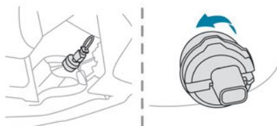
This bulb is replaced from outside the rear bumper.
