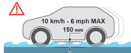
If the vehicle absolutely must drive through a flooded section of road:
