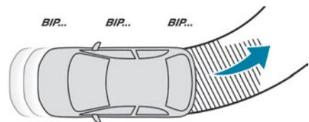
Depending on version, in the example shown, only the obstacles present in the shaded area will be signalled by the audible assistance. The proximity information is given by an intermittent audible signal, the frequency of
