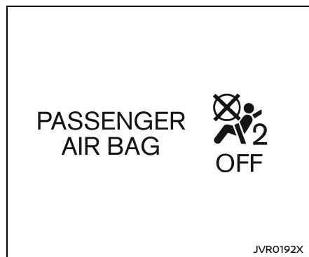
Front passenger air bag status light
