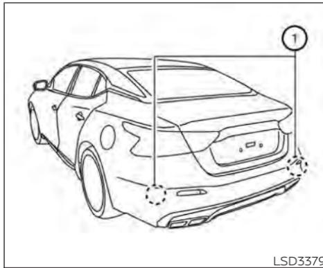
The RCTA system uses radar sensors ① installed on both sides near the rear bumper to detect an approaching vehicle.
