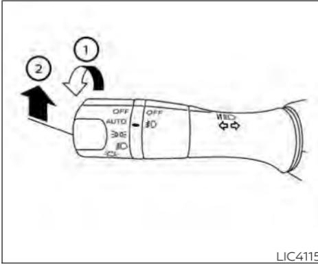
When the vehicle speed lowers to less than approximately 16 mph (25 km/h), the headlight uses the low beam.
