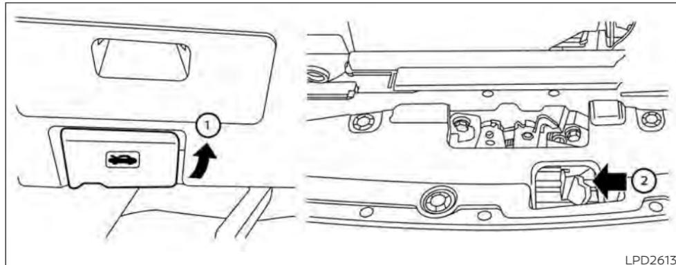
① Pull the hood lock release handle located below the driver side instrument panel. The hood will spring up slightly.
