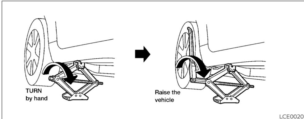
Always refer to the illustrations for the correct placement and jack-up points for your specific vehicle model and jack type.
