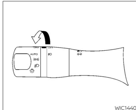
The headlights must be on and the low beams selected for the fog lights to operate. The fog lights automatically turn off when the high beam headlights are selected.
