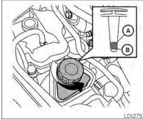
Check the fluid level in the reservoir.
