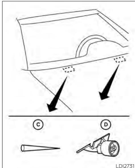
If you wax the surface of the hood, be careful not to let wax get into the washer nozzle **D**. This may cause clogging or improper windshield-washer operation. If wax gets into the nozzle, remove it with a needle or small pin **C**.
