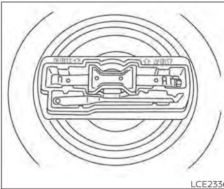
Remove the tool box from the spare tire.
