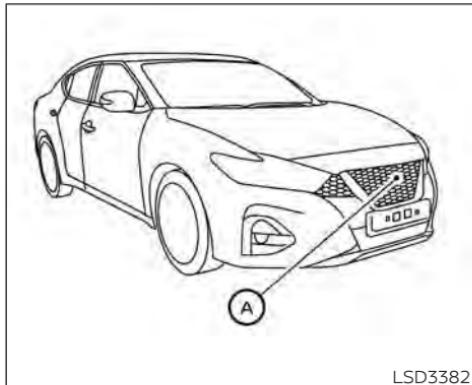
The I-FCW system uses a radar sensor Ⓐ located on the front of the vehicle to measure the distance to the vehicle ahead in the same lane.
