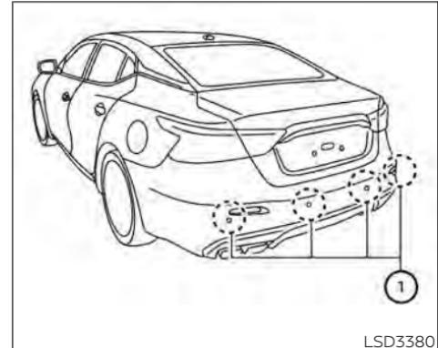
The RAB system detects obstacles behind the vehicle using the parking sensors ① located on the rear bumper.
