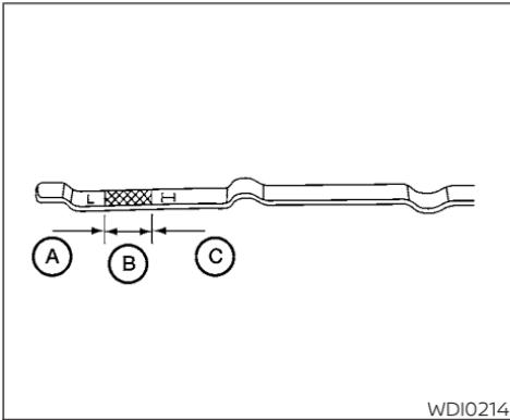
5. Remove the dipstick again and check the oil level. It should be between the H (High) and L (Low) marks ④. This is the normal operating oil level range. If the oil level is below the L (Low) mark ④, remove the oil filler cap and pour recommended oil through the opening. **Do not overfill ④.**
