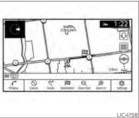
The icon will not move across the screen if the vehicle is moving over speeds of 4 mph (7 km/h), yet the information will still transfer to the vehicle information display.
