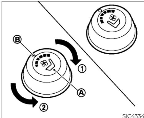
The climate-controlled seat warms up or cools down the front seat by a built-in heater or ventilates air into the seat. The climate control switch is located on the center console.
