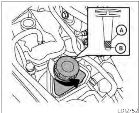
Check the fluid level in the reservoir.
