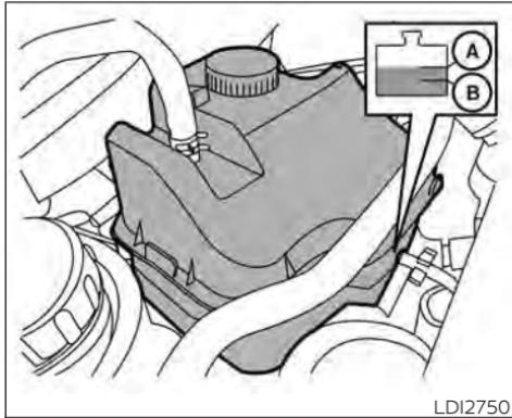
This vehicle contains Genuine NISSAN Long Life Antifreeze/Coolant (blue). The life expectancy of the factory-fill coolant is 105,000 miles (168,000 km) or 7 years. Mixing any other type of coolant or the use of non-distilled water will reduce the life expectancy of the factory-fill coolant. For additional information, see the "Maintenance and schedules" section of this manual.
