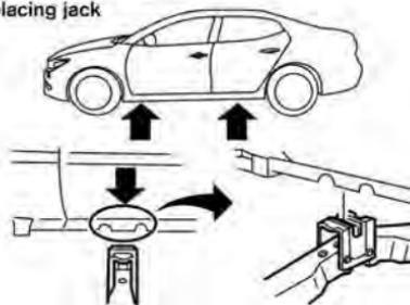
Jacking up vehicle and removing the damaged tire
