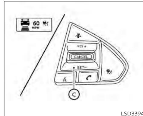
**To set cruising speed**, accelerate your vehicle to the desired speed, push the SET-switch **(C)** and release it. The ICC system set indicator (green), vehicle ahead detection indicator, set distance indicator and set vehicle speed indicator **(B)** will come on. Take your foot off the accelerator pedal. Your vehicle will maintain the set speed.
