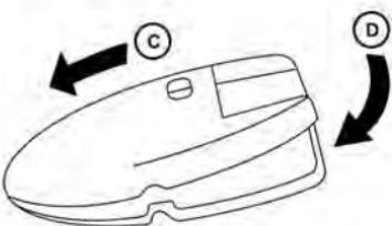
3. Replace the battery with a new one.
