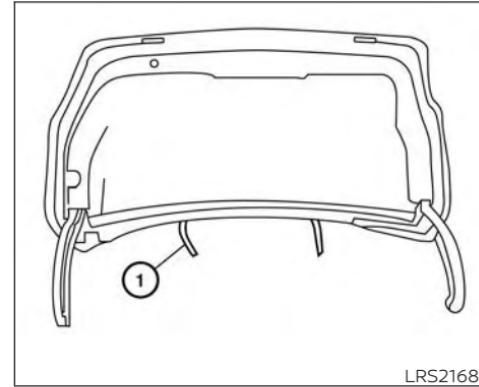
To fold down either side of the rear seat, open the trunk and pull on the strap ①.
