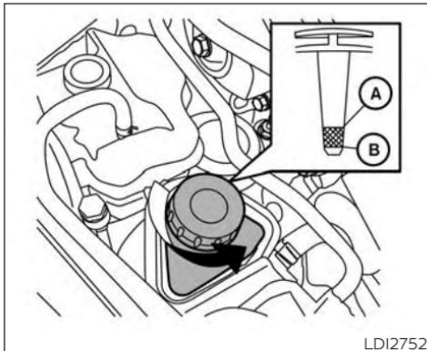
Check the fluid level in the reservoir.
