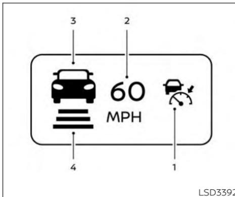
Vehicle-to-vehicle distance control mode display and indicators
