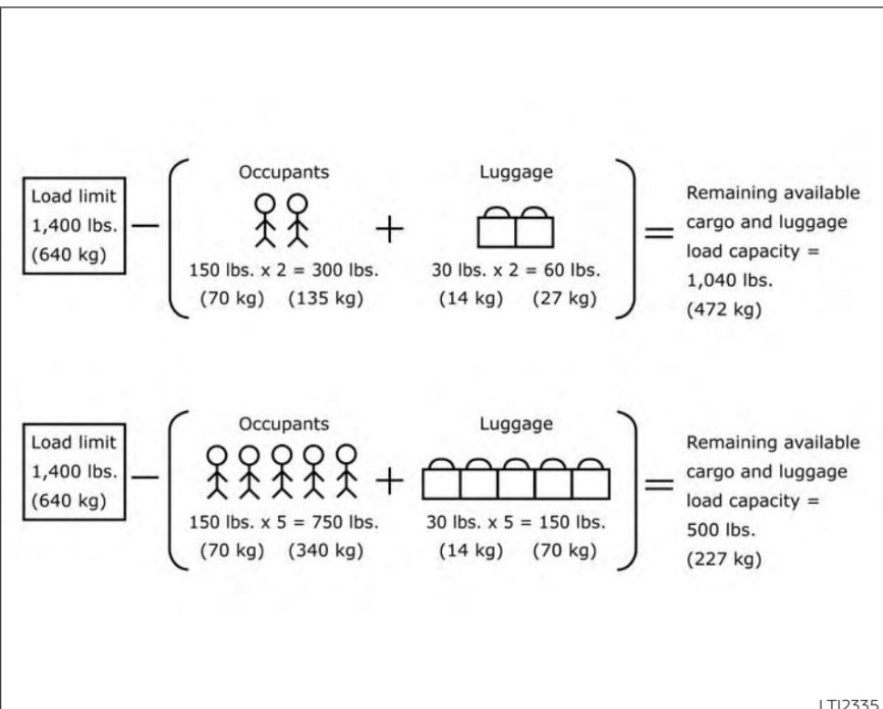
Steps for determining correct load limit
