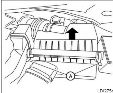
The air cleaner filter should not be cleaned and reused. Replace it according to the maintenance log shown in the "Maintenance and schedules" section of this manual. When replacing the filter, wipe the inside of the air cleaner filter housing and the cover with a damp cloth.
