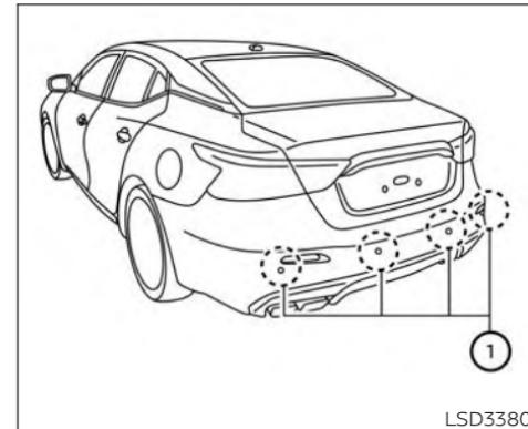
The RAB system detects obstacles behind the vehicle using the parking sensors ① located on the rear bumper.
