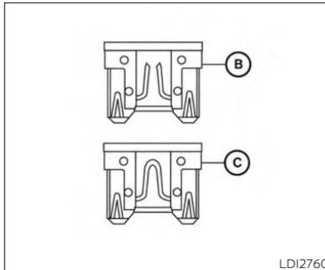
4. If the fuse is open **B**, replace it with an equivalent good fuse **C**.
