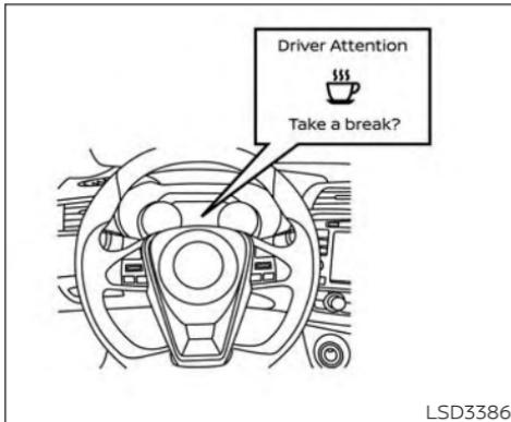
The system resets and starts reassessing driving style and steering behavior when the ignition switch is cycled from ON to OFF and back on.
