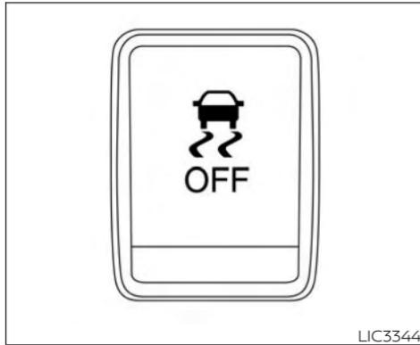
Push the VDC OFF switch again or restart the engine to turn on the system. For additional information, refer to "Vehicle Dynamic Control (VDC) system" in the "Starting and driving" section of this manual.
