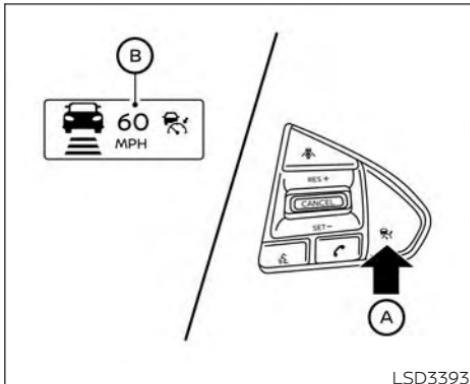
This message will disappear after about 6 seconds, or can be dismissed by pushing the OK button. Cruise control status will continue to display in the upper right corner of the vehicle information display while the system is on.
