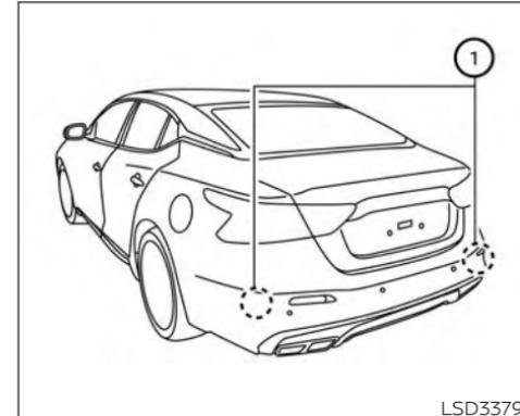
The BSW system uses radar sensors ① installed near the rear bumper to detect other vehicles in an adjacent lane.
