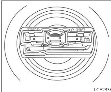
Remove the tool box from the spare tire.
