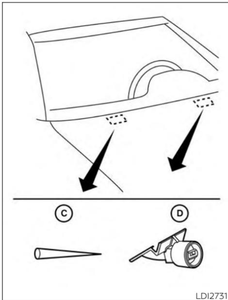
If you wax the surface of the hood, be careful not to let wax get into the washer nozzle **D**. This may cause clogging or improper windshield-washer operation. If wax gets into the nozzle, remove it with a needle or small pin **C**.
