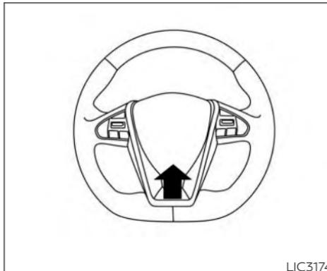
To sound the horn, push near the center pad of the steering wheel.
