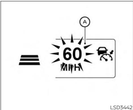
**When passing another vehicle**, the set speed indicator **(A)** will flash when the vehicle speed exceeds the set speed. The vehicle detect indicator will turn off when the area ahead of the vehicle is open. When the pedal is released, the vehicle will return to the previously set speed.
