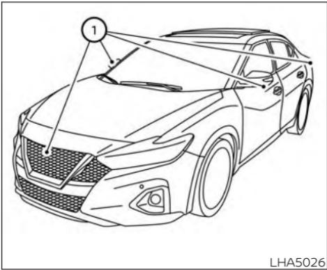
If dirt, rain or snow accumulates on any of the cameras ①, the Intelligent Around View Monitor may not display objects clearly. Clean the camera by wiping with a cloth dampened with a diluted mild cleaning agent and then wiping with a dry cloth.
