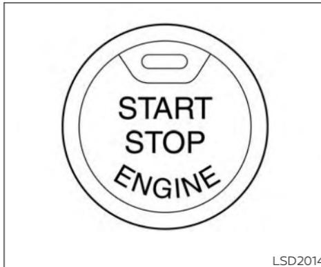
**If the battery of the vehicle is discharged, the push-button ignition switch cannot be moved from the LOCK position.**
