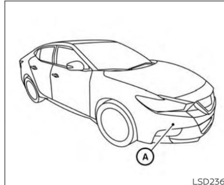
The I-FCW system uses a radar sensor **A** located behind the lower grille of the front bumper to measure the distance to the vehicle ahead in the same lane.
