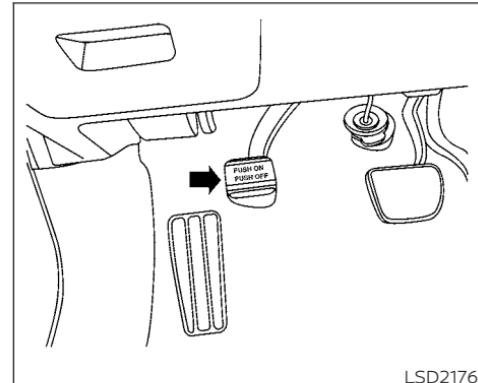
**To engage:** Firmly depress the parking brake.
