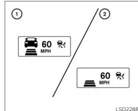
**When passing another vehicle,** the set speed indicator ② will flash when the vehicle speed exceeds the set speed. The vehicle detect indicator will turn off when the area ahead of the vehicle is open. When the pedal is released, the vehicle will return to the previously set speed.
