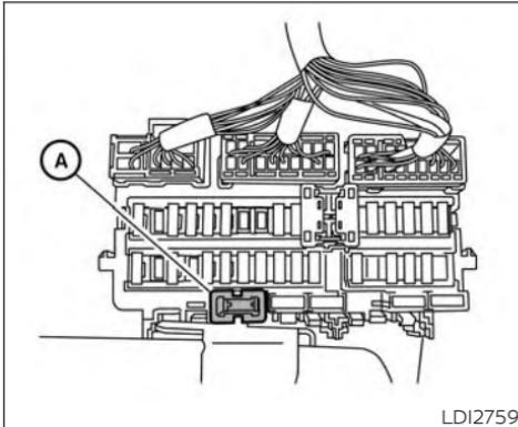
3. Remove the fuse with the fuse puller **A**.
