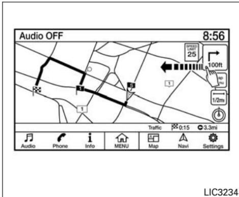
The icon will not move across the screen if the vehicle is moving over speeds of 7 kph (4 mph), yet the information will still transfer to the vehicle information display.
