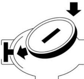
3. Replace the battery with a new one.
