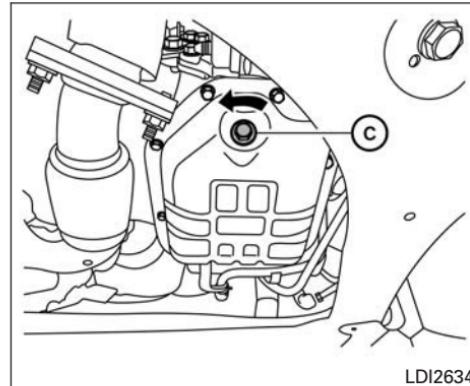
5. Place a large drain pan under the drain plug **C**.
