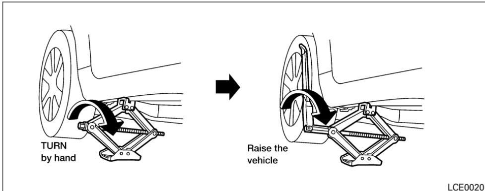
Always refer to the proper illustrations for the correct placement and jack-up points for your specific vehicle model and jack type.
