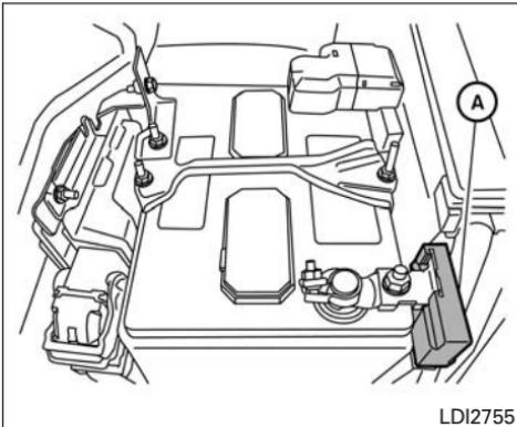
The current sensor **A** is located near the battery along the negative battery cable. If you add electrical accessories to your vehicle, be sure to ground them to a suitable body ground such as the frame or engine block area.
