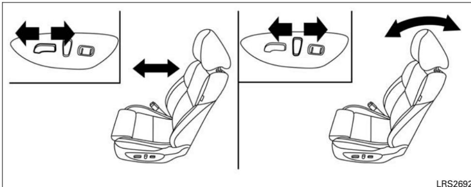
The reclining feature allows adjustment of the seatback for occupants of different sizes for added comfort and to help obtain proper seat belt fit. For additional information, refer to "Precautions on seat belt usage" in this section. Also, the seatback can be reclined to allow occupants to rest when the vehicle is stopped and the shift lever is in P (Park).
