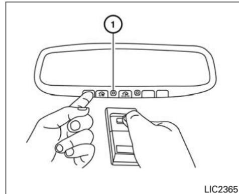
2. Using both hands, simultaneously press and hold the desired HomeLink® button and handheld transmitter button. DO NOT release until the HomeLink® indicator light (1) flashes slowly and then rapidly. When the indicator light (1) flashes rapidly, both buttons may be released. (The rapid flashing indicates successful programming.)
