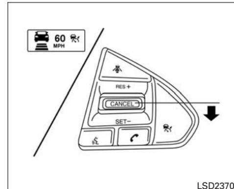
**To set cruising speed:** accelerate your vehicle to the desired speed, push the SET- switch and release it. The ICC system set indicator (green), vehicle ahead detection indicator, set distance indicator and set vehicle speed indicator **Ⓑ** will come on. Take your foot off the accelerator pedal. Your vehicle will maintain the set speed.
