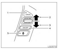
VEHICLE-TO-VEHICLE DISTANCE **CONTROL MODE SWITCHES**
