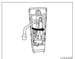
3. Collapse the jack to remove it from the storage location by inserting the wheel nut wrench into the jack screw at the top of the jack as shown. Turn the wheel-nut wrench counterclockwise as shown until the jack screw becomes loose. Then loosen the jack with your fingers until it becomes free
