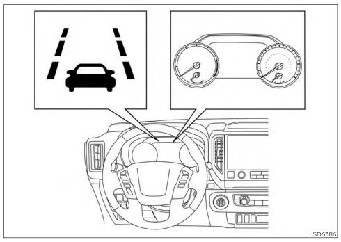
The LDW system provides a lane departure warning function when the vehicle is driven at speeds of approximately 37 mph (60 km/h) and above and the lane markings are clear. When the vehicle approaches either the left or the right side of the traveling lane, the steering wheel will vibrate and the LDW indicator on the instrument panel will blink to alert the driver.
