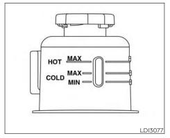
Check the power steering fluid level when the engine is stopped.
