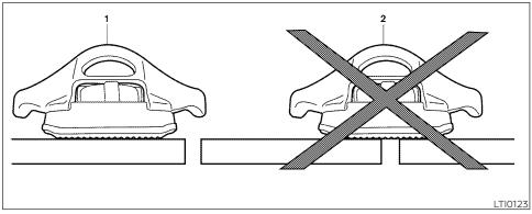
1 correct installation, 2 incorrect installation
