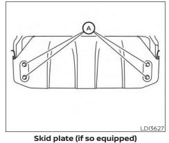
Removal of under-engine protectors
