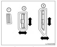
Adjust air flow direction for the driver and front passenger side vents 2 or center vents 3 by moving the vent slide and/or vent assemblies. The defrost vents (1) located above the driver and front passenger side vents cannot be adjusted or closed.
