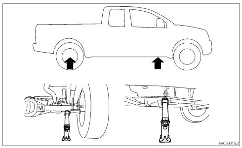
Always refer to the illustration for the correct placement and jack-up points for your specific vehicle model and jack type.
