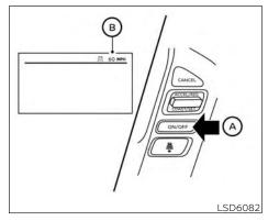
Operating vehicle-to-vehicle distance control mode
