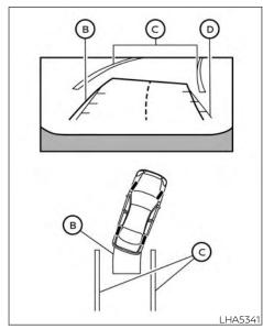
3. Slowly back up the vehicle adjusting the steering wheel so that the predicted course lines (B) enter the parking space
