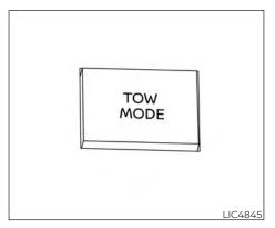
Tow mode should be used when pulling a heavy trailer or hauling a heavy load. Driving the vehicle in the tow mode with no trailer/load or light trailer/light load will not cause any damage. However, fuel economy may be reduced, and the transmission/engine driving characteristics may feel unusual.
