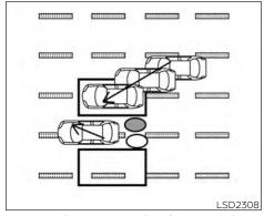
Illustration 6 - Entering from the side **Illustration 6:** If the driver activates the turn signal while another vehicle is in the detection zone, then the system chimes (twice) and the side BSW/RCTA indicator light and the BSW indicator (yellow) flash.
