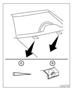
Be careful not to let anything get into the washer nozzle ②. This may cause clogging or improper windshield-washer operation. If something gets into the nozzle, remove it with a needle or small pin ③.
