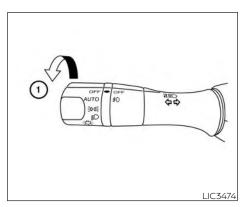
1. For USA: Turn the headlight switch to the AUTO position (1)
