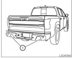
The RCTA system uses radar sensors (1) installed on both sides near the rear bumper to detect an approaching vehicle.
