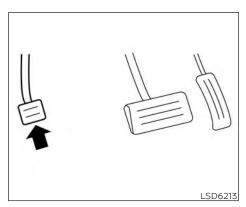
To engage: Firmly depress the parking brake.
