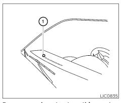
Be sure you do not put anything on top of the autolight sensor (1) located in the top side of the instrument panel. The autolight sensor controls the autolight; if it is covered, the autolight sensor reacts as if it is dark out and the headlights will illuminate. If this occurs while parked with the engine off and the switch in the ON position, your vehicle's battery could become discharged.
