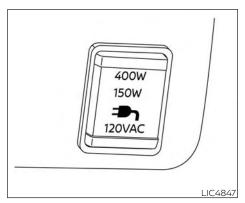
To use the outlets for devices that require up to 120v power, the vehicle must be running and the power inverter switch must be on.
