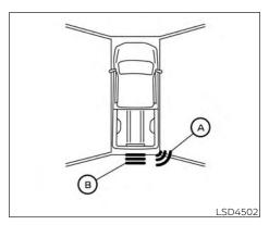
When the corner of the vehicle moves closer to an object, the corner sonar indicator  $\ensuremath{\Theta}$  appears. When the center of the vehicle moves close to an object, the center sonar indicator (B) appears.
