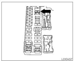
If a type (a) fuse is used to replace a type (b) fuse, the type (c) fuse will not be level with the fuse pocket as shown in the illustration. This will not affect the performance of the fuse. Make sure the fuse is installed in the fuse box securely.
