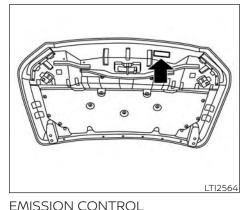
The emission control information label is attached to the underside of the hood as shown.
