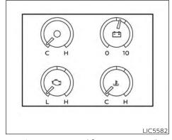
Auxiliary gauges (if so equipped)
