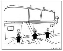
Rear bench seat (Crew Cab models) Top tether anchor point locations Anchor points are located under the rear window behind the rear bench seat (Crew Cab models) as shown
