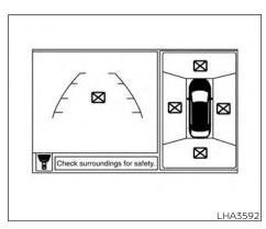
When the "[X]" icon is displayed on the screen, the camera image may be receiving temporary electronic disturbances from surrounding devices. This will not hinder normal driving operation but it is recommended that the system be inspected if it occurs frequently. It is recommended that you visit a NISSAN dealer for this service
