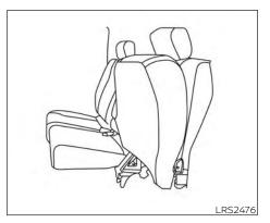
2. Fold the bottom of the seat cushion toward the back of the vehicle until it locks in place.
