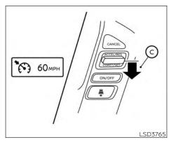
To set cruising speed, accelerate your vehicle to the desired speed, push the COAST/SET @ switch and release it. (The color of the cruise indicator changes to green and set vehicle speed indicator comes on.) Take your foot off the accelerator pedal. Your vehicle will maintain the set speed.
