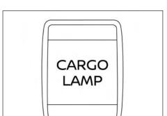
To turn on the cargo lamp, push the switch
