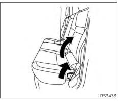
Lift up on the lever, located on the side of the seat, while lifting the front of the seat cushion up.
