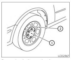
Removing bolt-on wheel caps (if so equipped)
