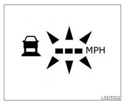
When the COAST/SET switch is pushed under the following conditions, the system cannot be set and the set vehicle speed indicator will blink for approximately 2 seconds:
