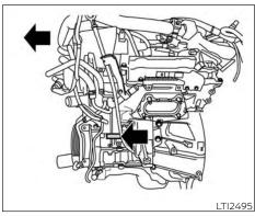
3.8L 6 cylinder (VQ38DD engine model) **FNGINE SERIAL NUMBER**
