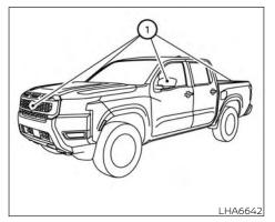
To display the multiple views, the Intelligent Around View® Monitor system uses cameras located in the front grille, on the vehicle's outside mirrors and one on the tail-gate  $\bigcirc$ .
