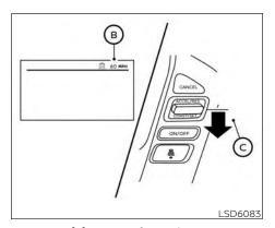
To set cruising speed, accelerate your vehicle to the desired speed, push the COAST/SET switch (a) and release it. The ICC system set indicator (green), vehicle ahead detection indicator, set distance indicator and set vehicle speed indicator (B) will come on. Take your foot off the accelerator pedal. Your vehicle will maintain the set speed.
