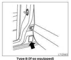
The Federal/Canadian Motor Vehicle Safety Standard (F.M.V.S.S./C.M.V.S.S.) certification label is affixed as shown. This label contains valuable vehicle information, such as: (GVWR), (GAWR), month and year of manufacture, (VIN), etc. Review it carefully.
