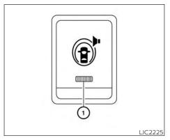
The warning systems switch is used to turn on and off the following systems that are activated using the Settings menu in the vehicle information display:
