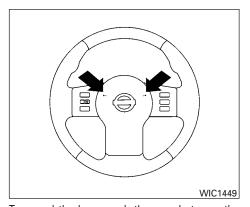
To sound the horn, push the area between the horn icons on the steering wheel.
