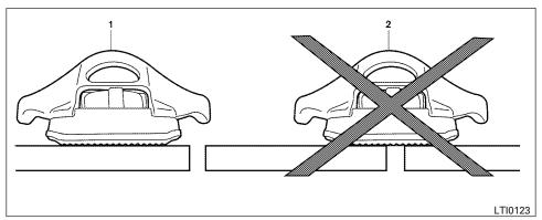
1 correct installation, 2 incorrect installation
