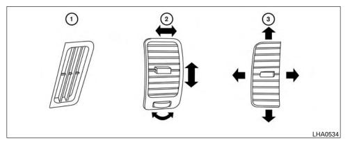
Adjust air flow direction for the vents directed at the driver's and passenger's side windows (1), driver and passenger (2), or center (3) by moving the vent slide and/or vent assemblies.
