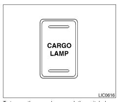
To turn on the cargo lamp, push the switch down to the ON position.
