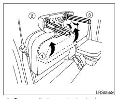
1. To access the jump seat extension (passenger's side only) (1) on the jump seat, pull up (2) on the extension to unfold it to the open position. Then unfold the two support leas (3) and lower the jump seat to the full open seating position.
