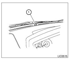
The sunload sensor (1), located on the top center of the instrument panel, helps the system maintain a constant temperature. Do not put anything on or around this sensor.
