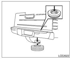
To reinstall the wheel, insert the tire chain through the wheel. Be sure the rubber spacer is centered on the wheel before lifting. Use the assembled jack rod and slowly rotate the winch clockwise to raise the wheel to the vehicle.
