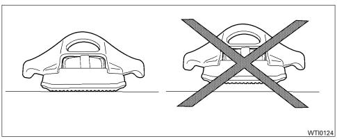
5. There should be no gap between the bottom of the cleat and the top of the channel. Tighten the center bolt hand tight (20-40 inlbs).
