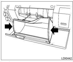
1. Open the glove box and press in on the sides so that it will open completely allowing it to hang by the cord.
