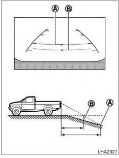
the hill is the place (B). Note that any object on the hill is closer than it appears on the monitor.
