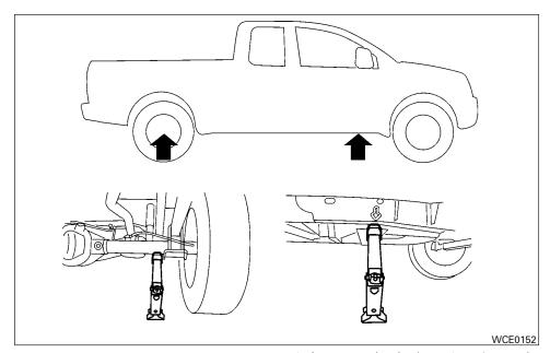
Always refer to the illustration for the correct placement and jack-up points for your specific vehicle model and jack type.
