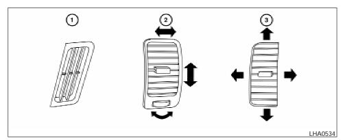
Adjust air flow direction for the driver's and passenger's side windows (1), driver and passenger (2), or center (3) vent by moving the vent slide and/or vent assemblies.
