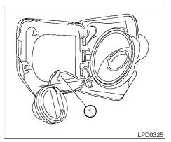
Loop the tether strap around the hook (1) while refueling.
