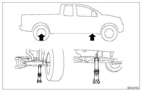
2. Place the jack directly under the jack-up point as illustrated so the top of the jack contacts the vehicle at the jack-up point. The jack-up points are indicated by stamped arrows on the side of the frame.
