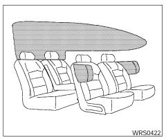
Front seat-mounted side-impact supplemental air bag (if so equipped) and roof-mounted curtain side-impact and rollover supplemental air bag (if so equipped) systems
