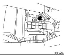
2. Lift upward to release the filter cover and remove the filter cover.
