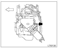
**QR25DE** engine **ENGINE SERIAL NUMBER**
