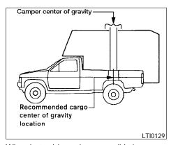
When the truck is used to carry a slide-in camper, the total cargo load of the truck consists of the camper manufacturer's weight figure, plus:
