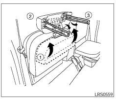
To access the jump seat extension ① on the passenger's side jump seat only pull up ② on the extension to unfold it to the open position. Then unfold the two support legs ③ and lower the jump seat to the full open ④ seating position.
