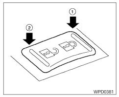
Door lock switch LOCKING WITH POWER DOOR LOCK SWITCH (if so equipped)
