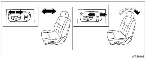
The reclining feature allows adjustment of the seatback for occupants of different sizes for added comfort and to help obtain proper seat belt fit (see "Precautions on seat belt usage" later in this section). Also, the seatback can be reclined to allow occupants to rest when the vehicle is stopped and the transmission is in P (Park) or N (Neutral) position with the parking brake fully applied.
