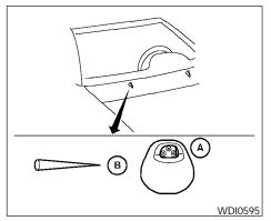
If you wax the surface of the hood, be careful not to let wax get into the washer nozzle (a). This may cause clogging or improper windshield washer operation. If wax gets into the nozzle, remove it with a needle or small pin (B).
