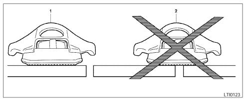
1 correct installation, 2 incorrect installation
