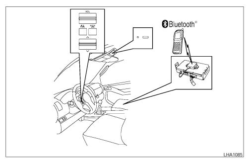
Your NISSAN is equipped with the Bluetooth® Hands-Free Phone System. If you have an approved Bluetooth® enabled cellular phone, you can set up the wireless connection between your cellular phone and the in-vehicle phone module. With Bluetooth® wireless technology, you can
