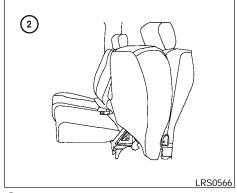
Fold the bottom of the seat cushion toward the back of the vehicle until it locks in place.
