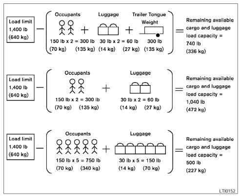
Steps for determining correct load limit
