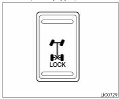
The Electronic Locking Rear Differential (E-Lock) system can help provide added traction if the vehicle is stuck or becoming stuck.
