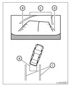
3. Slowly back up the vehicle adjusting the steering wheel so that the predicted course lines (B) enter the parking space (C).
