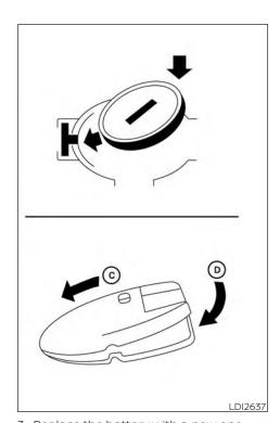
3. Replace the battery with a new one.
