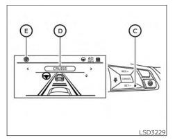
5. Push the SET- switch (a). The ProPILOT Assist system begins to automatically maintain the set speed. The ProPILOT Assist activation indicator (D) and Pro-PILOT Assist status indicator (E) illuminate (blue). When a vehicle ahead is traveling at a speed of 20 mph (30 km/h) or below and the SET-switch is pushed, the set speed of your vehicle is 20 mph (30 km/h).
