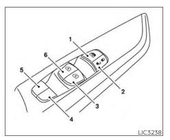
To open a window, push the switch to the detent and continue to hold down until the desired window position is reached. To close a window, pull the switch to the detent and continue to hold up until the desired window position is reached.
