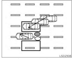
Illustration 6 - Entering from the side Illustration 6: If the driver activates the turn signal while another vehicle is in the detection zone, then the system chimes (twice), the side BSW/RCTA indicator light and the BSW indicator flash
