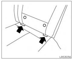
**LATCH lower anchor location** I ATCH lower anchor location
