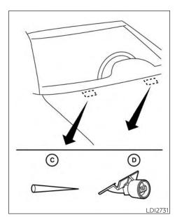
If you wax the surface of the hood, be careful not to let wax get into the washer nozzle ①. This may cause clogging or improper windshield-washer operation. If wax gets into the nozzle, remove it with a needle or small pin ②.
