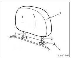
NON-ADJUSTABLE HEAD RESTRAINT/HEADREST **COMPONENTS**
