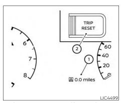
**5 inch (13 cm) Type A (if so equipped)** Odometer/Twin trip odometer
