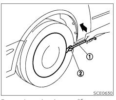
Removing wheel cover (if so equipped)
