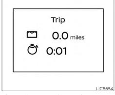
Elapsed time and trip odometer
