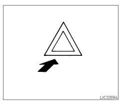
Push the switch on to warn other drivers when you must stop or park under emergency conditions. All turn signal lights flash.
