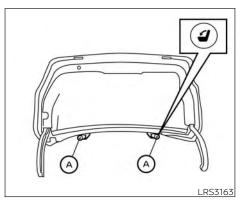
To fold down either side of the rear seat, open the trunk and pull on the knob on that side 🔕 .
