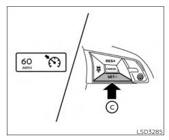
To set cruising speed, accelerate your vehicle to the desired speed, push the SET- @ switch and release it. (The color of the cruise indicator changes to green and set vehicle speed indicator comes on.) Take vour foot off the accelerator pedal. Your vehicle will maintain the set speed.
