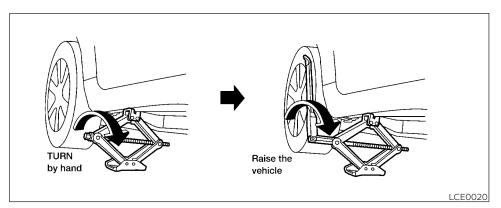
To lift the vehicle, securely hold the jack lever and rod with both hands. Carefully raise the vehicle until the tire clears the ground. Remove the wheel nuts, and then remove the tire.
