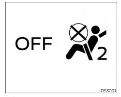
7 If the booster seat is installed in the front passenger seat, place the ignition switch in the ON position. The front passenger air bag status light " May or may not illuminate, depending on the size of the child and the type of booster seat being used. For additional information, see "Front passenger air bag and status light" (P. 65).
