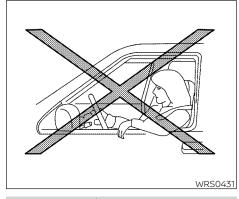
Even with the NISSAN Advanced Air Bag System, never install a rearfacing child restraint in the front seat. An inflating front air bag could seriously injure or kill your child. For additional information, see "Child restraints" (P. 32).
