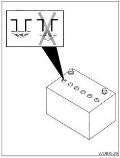
2. Check the fluid level in each cell. If it is necessary to add fluid, add only distilled water to bring the level up to the bottom of the filler opening. Do not overfill. Reinstall the vent caps.
