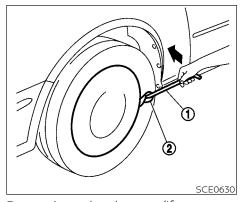
Removing wheel cover (if so equipped)
