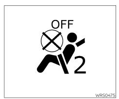
7. If the booster seat is installed in the front passenger seat, place the ignition switch in the ON position. The front passenger air bag status light 🌋 may or may not illuminate, depending on the size of the child and the type of booster seat being used. For additional information, refer to "Front passenger air bag and status light" in this section.
