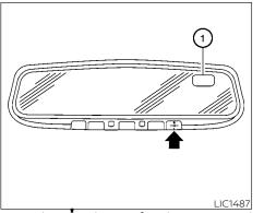
Press the -N- button for about 1 second when the ignition switch is placed in the ON position to toggle the compass display (1) on or off. The display will indicate the direction of the vehicle's heading. N: North
