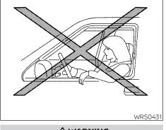
Even with the NISSAN Advanced Air Bag System, never install a rearfacing child restraint in the front seat. An inflating front air bag could seriously injure or kill your child. For additional information, refer to "Child restraints" in this section.
