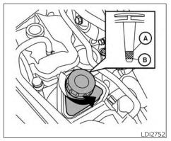
Check the fluid level in the reservoir
