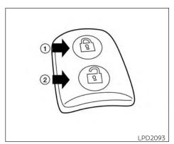
**Door lock switch**LOCKING WITH POWER DOOR
