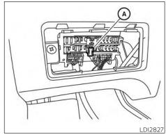
3. Remove the fuse with the fuse puller
