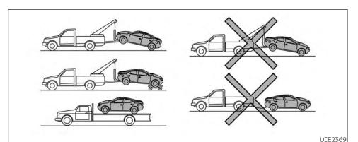
2WD models with Continuously Variable Transmission (CVT)
