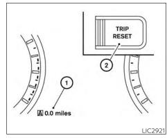
Odometer/Twin trip odometer
