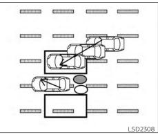
Illustration 6 - Entering from the side Illustration 6: If the driver activates the turn signal while another vehicle is in the detection zone, then the system chimes (twice) and the side indicator light flashes.
