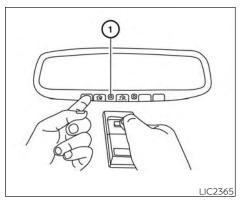
Position the end of your hand-held transmitter 1-3 in (2-8 cm) away from the HomeLink® surface, keeping the HomeLink® indicator light ① in view.
