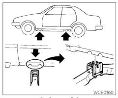
Jack-up point Jacking up vehicle and removing the damaged tire
