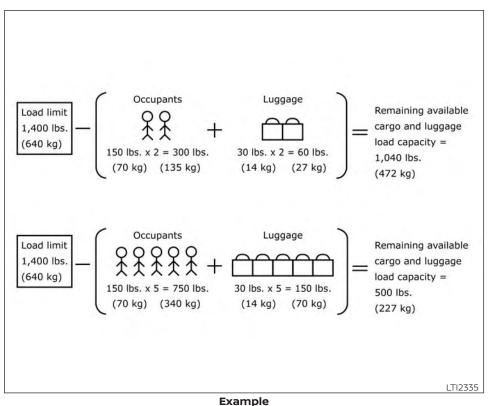
Steps for determining correct load limit
