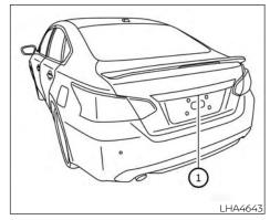
To display the rear view, the Rear View Monitor system uses a camera located just above the vehicle's license plate ①.
