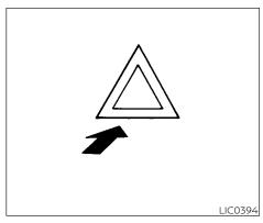
Push the switch on to warn other drivers when you must stop or park under emergency conditions. All turn signal lights flash.
