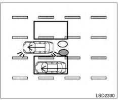
Illustration 2 - Approaching from behind Illustration 2: If the driver activates the turn signal when another vehicle is in the detection zone, then the system chimes (twice) and the
