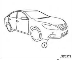
The FEB system uses a radar sensor (1) located on the front of the vehicle to measure the distance to the vehicle ahead in the same lane.
