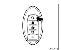
button will be on the NISSAN Intelligent Key® if the vehicle has remote engine start. This feature allows the engine to start from outside the vehicle.
