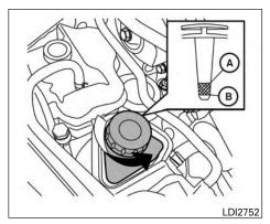
Check the fluid level in the reservoir.
