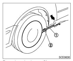
Removing wheel cover (if so equipped)
