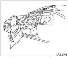
SRS air bag warning labels (located on the sun visors)
