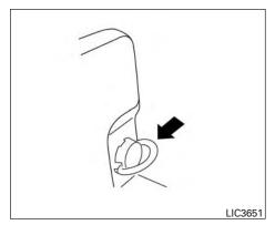
To install a cargo net, attach the net to the retainers.
