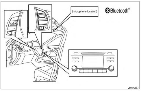
Your NISSAN is equipped with the Bluetooth® Hands-Free Phone System. If you have a compatible Bluetooth® enabled cellular phone, you can set up the wireless connection between your cellular phone and the in-vehicle phone module. With Bluetooth® wireless technology, you can make or receive a hands-free telephone call with your cellular phone in the vehicle.
