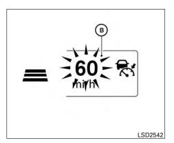
When passing another vehicle, the set speed indicator (B) will flash when the vehicle speed exceeds the set speed. The vehicle detect indicator will turn off when the area ahead of the vehicle is open. When the pedal is released, the vehicle will return to the previously set speed.
