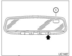
Press the -Nbutton for about 1 second when the ignition switch is placed in the ON position to toggle the compass display (1) on or off. The display will indicate the direction of the vehicle's heading.
