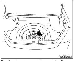
Turn the clamp to remove the spare tire. Remove the spare tire.
