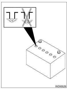
Check the fluid level in each cell. If it is necessary to add fluid, add only distilled water to bring the level up to the bottom of the filler opening. Do not overfill. Reinstall the vent caps. Vehicles operated in high temperatures or under severe conditions require frequent checks of the battery fluid level.
