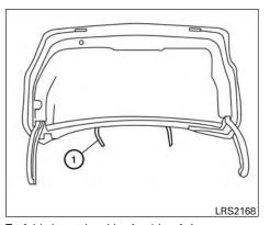
To fold down the driver's side of the rear seat. open the trunk and pull on the strap (1).
