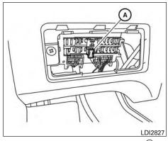
3. Remove the fuse with the fuse puller (A).
