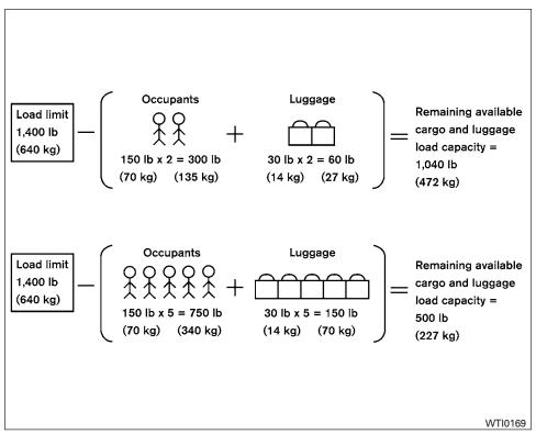
Steps for determining correct load limit
