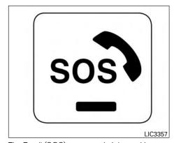
The E-call (SOS) system switch is used in combination with a NissanConnect<sup>SM</sup> Services subscription to call for assistance in case of an emergency.
