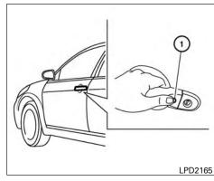
ing the door handle, push the door handle request switch to unlock the door.
