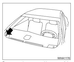
Be sure you do not put anything on top of the autolight sensor located in the top side of the instrument panel. The autolight sensor controls the autolight; if it is covered, the autolight sensor reacts as if it is dark out and the headlights will illuminate. If this occurs while parked with the engine off and the key in the ON position, your vehicle's battery could become discharged.
