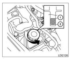
Check the fluid level in the reservoir.
