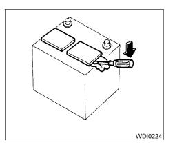
1. Remove the vent caps with a screwdriver as shown. Use a cloth to protect the battery case.
