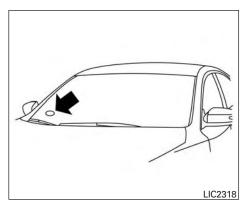
Be sure you do not put anything on top of the autolight sensor located in the top side of the instrument panel. The autolight sensor controls the autolight; if it is covered, the autolight sensor reacts as if it is dark out and the headlights will illuminate. If this occurs while parked with the engine off and the ignition switch placed in the ON position, your vehicle's battery could become discharged.
