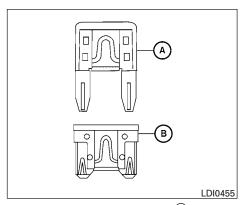
Two types of fuses are used. Type (A) is used in the fuse boxes in the engine compartment. Type (B) is used in the passenger compartment fuse hox.
