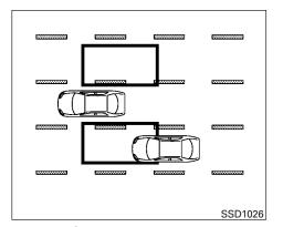
The Blind Spot indicator light illuminates if a vehicle enters the detection zone from behind in an adjacent lane.
