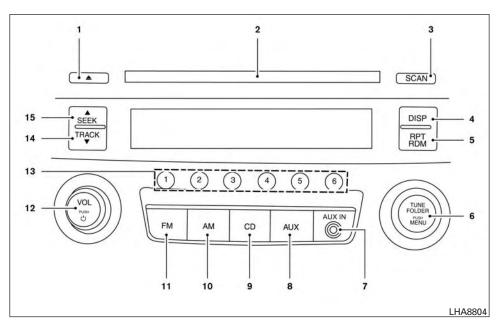
FM/AM RADIO WITH COMPACT DISC (CD) PLAYER (Type A) (if so equipped)
