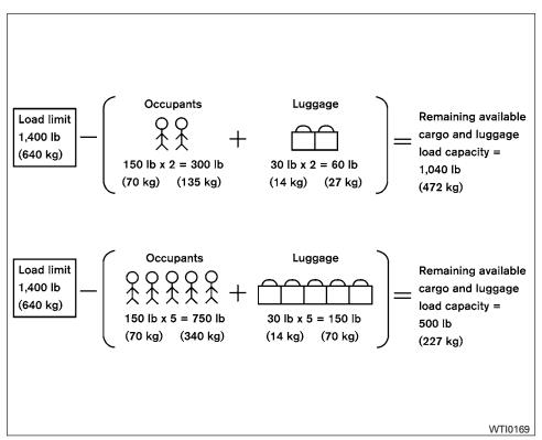
Steps for determining correct load limit
