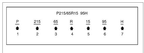
H: Tire speed rating. You should not drive the vehicle faster than the tire speed rating.
