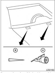
If you wax the surface of the hood, be careful not to let wax get into the windshield-washer nozzle (A). This may cause clogging or improper windshield-washer operation. If wax gets into the nozzle, remove it with a needle or small pin (B).
