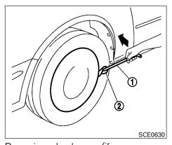
Removing wheel cover (if so equipped)
