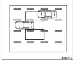
If the driver activates the turn signal while another vehicle is in the detection zone, then the Blind Spot indicator light flashes and a chime will sound twice.
