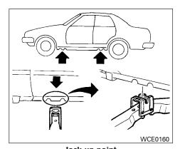
Jack-up point lacking up vehicle and remove
