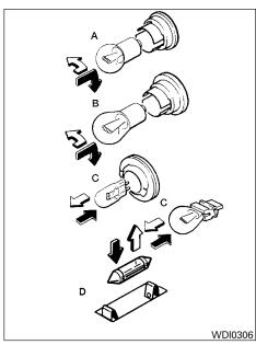
replacing a bulb, first remove the lens, light and/or cover.
