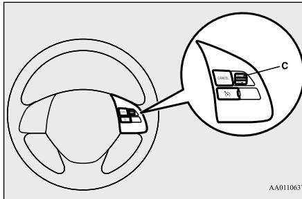
To increase your speed in small amounts, push up the RES + switch for less than about 1 second and release it.
