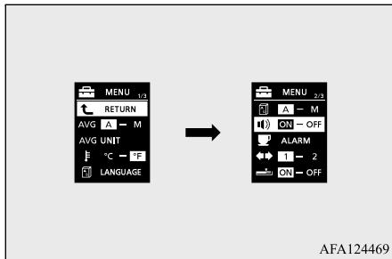
3. Press and hold the multi-information meter switch (for about 2 seconds or more) to switch in sequence from ON (operation sound on) → OFF (operation sound off) → ON (operation sound on). The setting is changed to the selected condition.
