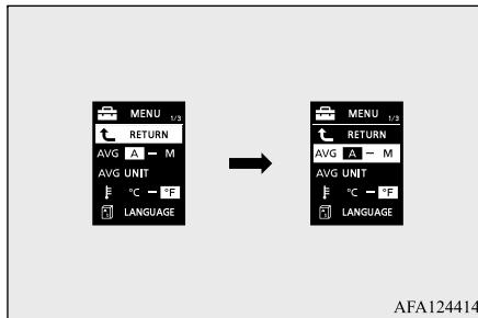
3. Press and hold the multi-information meter switch (for about 2 seconds or more) to switch in sequence from A or 1 (Auto reset) → M, 2 or P (Manual reset) → A or 1 (Auto reset).
