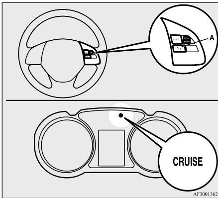
2. Accelerate or decelerate to your desired speed, then push down and release the SET - switch (B) when the "CRUISE" indicator light is illuminated. The vehicle will then maintain the desired speed.
