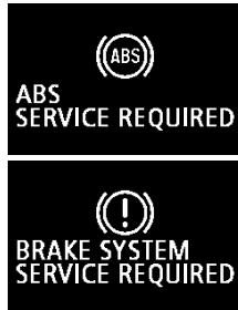
The anti-lock braking system and brake force distribution function may not work, so hard braking could make the vehicle unstable.
