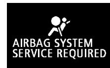
The system checks itself every time the ignition switch is turned to the “ON” position or the operation mode is put in ON. The SRS warning light will come on for several seconds and then go out. This is normal and means the system is working properly.
