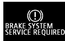
When the ignition switch is turned to the "ON" position or the operation mode is put in ON, if the brake fluid is low, this warning is displayed.
