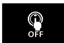
If the driver's door is opened while the engine is stopped and the operation mode is in any position other than OFF, the operation mode ON buzzer will sound intermittently to remind you to put the operation mode in OFF.
