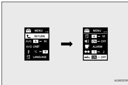
3. Press and hold the multi-information meter switch for about 2 seconds or more to switch in sequence from ON (with the green bar graph) → OFF (without the green bar graph) → ON (with the green bar graph).
