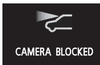
When the sensor performance returns, the FCM functions will resume operation. If the message continues showing, there is a possibility that the sensor has a malfunction. Contact an authorized Mitsubishi Motors dealer for inspection of the sensor.
