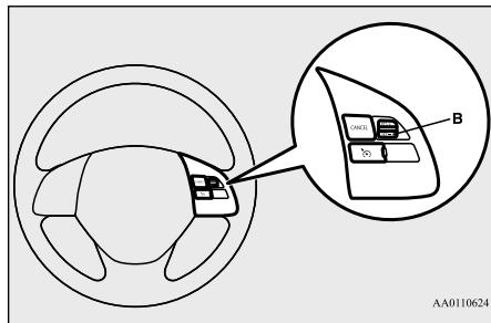
To slow down your speed in small amounts, push down the SET - switch for less than about 1 second and release it.
