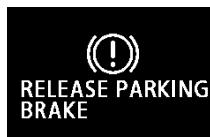
This warning is displayed if the vehicle is being driven with the parking brake still applied. The warning light in the instrument cluster only comes on when the parking brake is applied.
