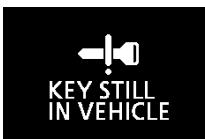
When the operation mode is in OFF, the F.A.S.T.-key is left in the passenger compartment, all the doors and the liftgate are closed, and someone tries to lock the vehicle by pressing the driver's or front passenger's door lock/unlock switch, or the liftgate LOCK switch, the warning display is displayed and the buzzer sounds for about 3 seconds as a
