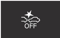
To turn on the FCM again, press the FCM ON/OFF switch. The
