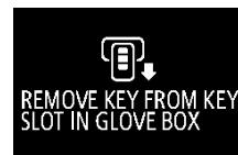
If the operation mode is in OFF and the driver's door is opened with the F.A.S.T.-key in the key slot, the outer buzzer sounds for approximately 3 seconds and the inner buzzer sounds for approximately 1 minute. A warning display also appears for approximately 1 minute to remind you to remove the key.
