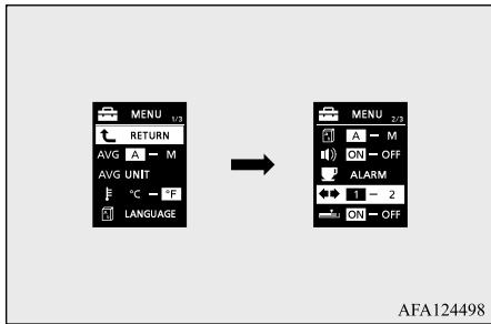
3. Press and hold the multi-information meter switch for about 2 seconds or more to switch in sequence from 1 (turn signal sound 1) → 2 (turn signal sound 2) → 1 (turn signal sound 1).
