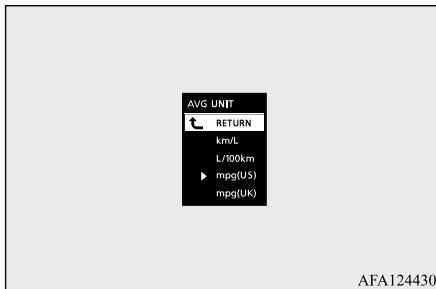
5. Press and hold the multi-information meter switch (for about 2 seconds or more) to change the setting to the selected unit.
