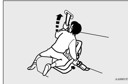
If your child restraint system requires the use of a tether strap, fasten the tether strap in accordance with procedures 6 and 7.
