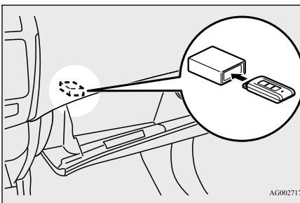
4. With the first valid F.A.S.T.-key, press and hold the UNLOCK button for 4 to 8 seconds and then press and hold the LOCK button during this time.
