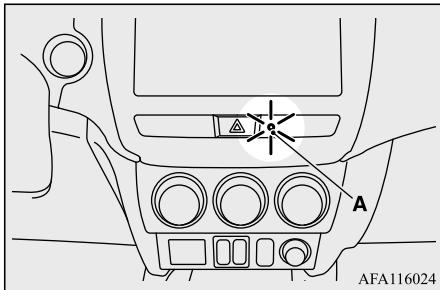
4. The system has entered the armed stage after about 20 seconds\*, when the theft-alarm indicator (A) blinking becomes slower.
