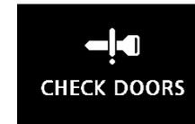
When the operation mode is in OFF, and someone tries to lock the vehicle by pressing the driver's or front passenger's door lock/unlock switch, or the liftgate LOCK switch while one of the doors or the liftgate is not fully closed, the warning display is displayed and the buzzer sounds for about 3 seconds as a warning, and the doors and the liftgate cannot be locked.
