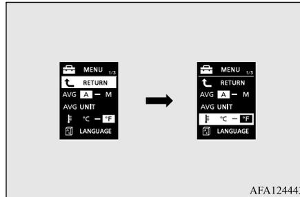
3. Press and hold the multi-information meter switch (for about 2 seconds or more) to change in sequence from °F → °C → °F.
