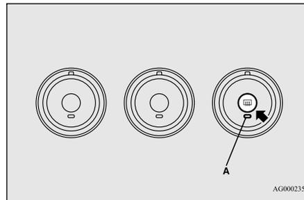
After about 20 minutes of operation, the system will shut off automatically.
