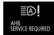
[When the sensor is malfunctioning]
