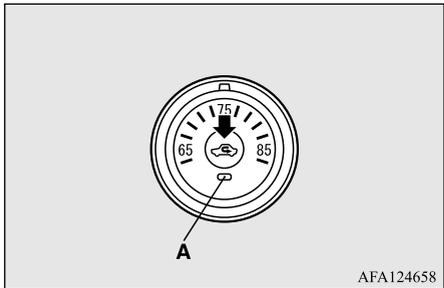
When the air conditioning turns on, the air selection is controlled automatically. When the air conditioning turns off, the air selection automatically goes back to the outside air position.
