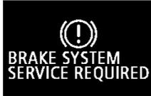
The anti-lock braking system and brake force distribution function may not work, so hard braking could make the vehicle unstable. Avoid hard braking and high-speed driving. Stop the vehicle in a safe place and contact an authorized Mitsubishi Motors dealer or repair facility of your choice.
