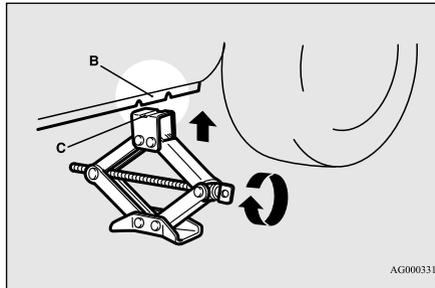
4. Make sure that the flange portion at the jacking point fits in the groove at the top of the jack. Insert the bar (D) into the wheel nut wrench (E). Then put the end of the bar into the shaft's jack end, as shown in the illustration.
