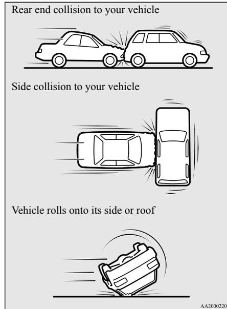
**The front airbags and driver's knee airbag MAY DEPLOY when**
