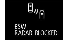
When the warning display appears, the radar sensor cannot detect a vehicle traveling side by side or an approaching vehicle, because foreign objects, such as dirt, snow or ice, adhere to the bumper surface around the sensor.
