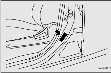
This placard shows the maximum number of occupants permitted to ride in your vehicle as well as “the combined weight of occupants and cargo” (A), which is called the vehicle capacity weight. The weight of roof load is included in the definition of “cargo” when determining the vehicle capacity weight. This placard also tells you the size and recommended inflation pressure for the original equipment tires on your vehicle. For more information, refer to “Tires” on page 9-14.
