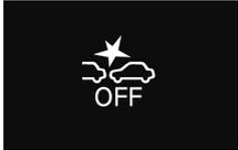
To turn on the FCM again, press the FCM ON/OFF switch. The
