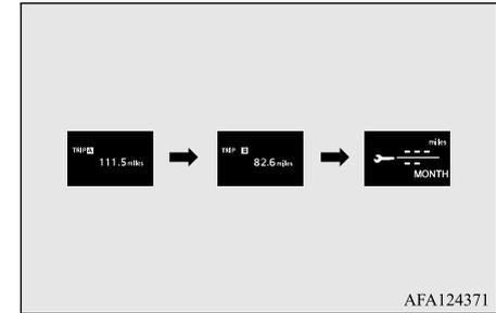
2. Press and hold the multi-information meter switch (for about 2 seconds or more) to display “
