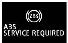
If there is a malfunction in the system, the anti-lock braking system warning light will come on and the warning display will appear
