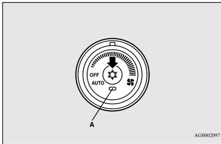
**7** Push the switch again and the air conditioning compressor will stop and the indicator light (A) goes off.
