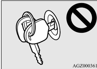
In cases like the above, move the offending object(s) away from the key and turn the key back to the “ACC” or “OFF” position. Then try to start the engine again. If the engine does not start, contact an authorized Mitsubishi Motors dealer.
