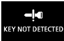
When the operation mode in any mode other than OFF, if the door(s) are opened, the F.A.S.T.-key is removed from the passenger compartment, and then the door(s) are closed,
