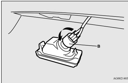
3. Pull the bulb out of the socket.
