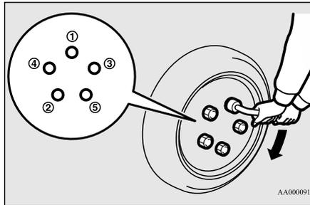
8. Lower the vehicle slowly until the tire touches the ground, by rotating the wheel nut wrench counterclockwise.
