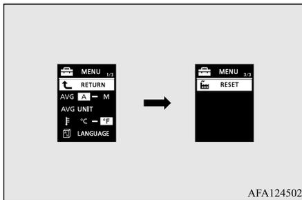
3. Press and hold the multi-information meter switch (for about 5 seconds or more), the buzzer sounds and all of the function settings are returned to the factory settings.
