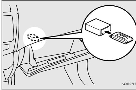
4. With the first valid F.A.S.T.-key, press and hold the UNLOCK button for 4 to 10 seconds and then press and hold the LOCK button during this time.
