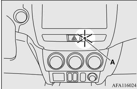
4. The system has entered the armed stage after about 20 seconds, when the theft-alarm indicator (A) flashing becomes slower.
