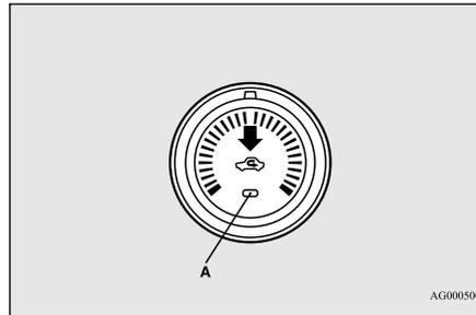
When the air conditioning turns on, the air selection is controlled automatically. The air selection indicator light (A) shows the selected position.
