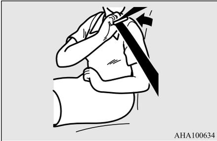
4. Pull the seat belt out slowly while holding the latch plate. Push the latch plate into the buckle until you hear a “click”. Pull up on the belt to be sure the latch plate is locked securely in the buckle.
