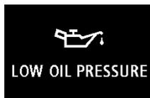
If the engine oil pressure drops while the engine is running, the warning display is displayed on the information screen in the multi-information display.
