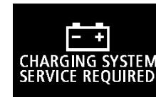
If there is a fault in the charging system, the warning display warning is displayed on the information screen in the multi-information display. The warning light in the instrument cluster also illuminates.
