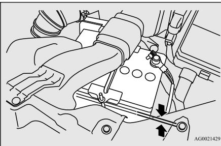
The electrolyte level must be between the limits shown on the outside of the battery. Fill it with distilled water as needed. The inside of the battery is divided into several compartments. Take the cap off of each compartment and fill to the mark.
