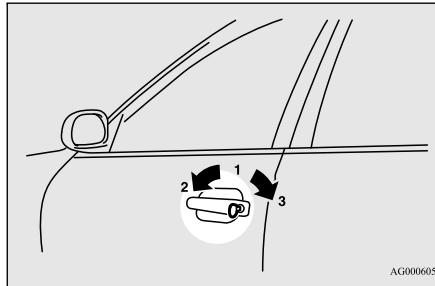
1- Insert or remove the emergency key
