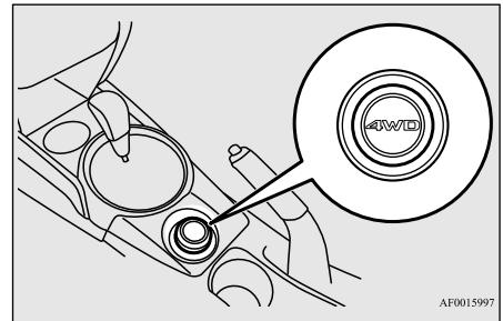
By pressing the drive mode-selector, the drive mode can be changed in order of “2WD”, “4WD AUTO” and “4WD LOCK”.
