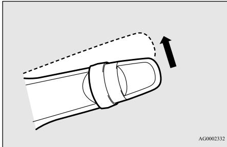
The wipers will operate once if the lever is moved to the "AUTO" position and the knob (C) is turned in the "+" direction when the ignition switch or the operation mode is in ON.
