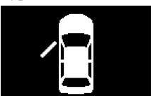
If any of the doors or the liftgate is not completely closed, this displays the open door or liftgate.
