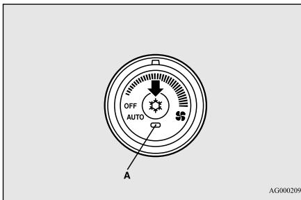
Push the switch again and the air conditioning compressor will stop and the indicator light (A) goes off.
