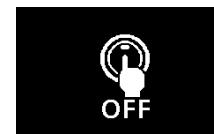
If the driver's door is opened while the engine is stopped and the operation mode is in any position other than OFF, the operation mode ON buzzer will sound intermittently to remind you to put the operation mode in OFF.
