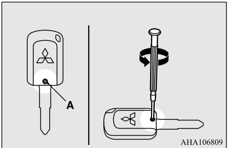
3. With the Mitsubishi mark facing you, insert the cloth-covered tip of a flat blade screwdriver into the notch in the remote control transmitter case and use it to open the case.
