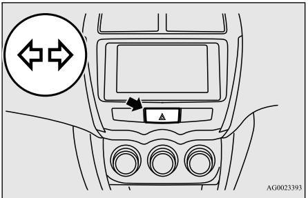
If you press the flasher switch, the front and rear turn signals will flash intermittently, and so will the hazard warning lights. This is an emergency warning system and should not be used when the vehicle is in motion, except for emergencies.
