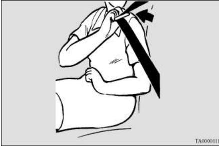
4. Pull the seat belt out slowly while holding the latch plate. Push the latch plate into the buckle until you hear a “click”. Pull up on the belt to be sure the latch plate is locked securely in the buckle.
