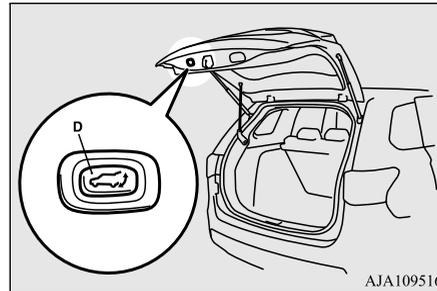
If the close switch on the power liftgate is pressed, the power liftgate will close after the warning buzzer sounds 3 times and the hazard warning flasher blinks 2 times.
