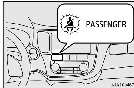
When the ignition switch is turned to the “ON” position or the operation mode is put in ON, this indicator normally comes on and goes off a few seconds later.
