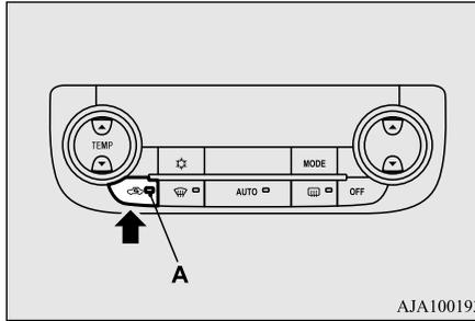
When the air conditioning turns on, the air selection is controlled automatically. When the air conditioning turns off, the air selection automatically goes back to the outside position.
