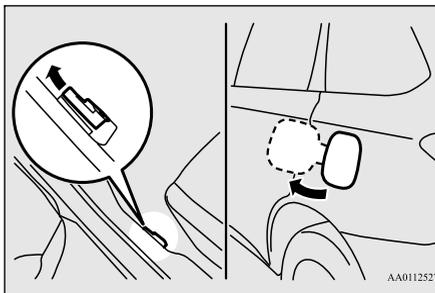
3. Open the fuel tank filler pipe by slowly turning the fuel tank filler cap counter-clockwise.
