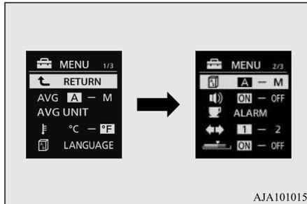
3. Press and hold the multi information display switch to switch from A/1 (language cooperation: enabled) to M/2/P (language cooperation: disabled), or from M/2/P to A/1. The setting is changed to the selected condition.
