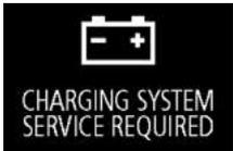
If there is a fault in the charging system, the warning display is displayed on the information screen in the multi information display. The warning light in the instrument cluster also illuminates.
