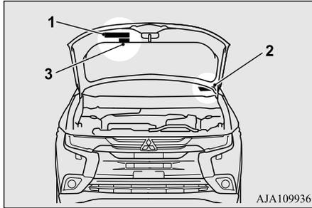
The air conditioning label is affixed on the inside panel of the engine hood.
