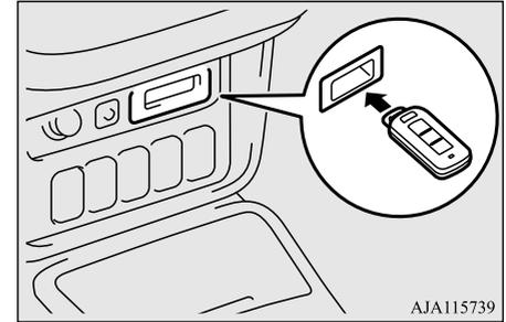
4. With the first valid F.A.S.T.-key, press the UNLOCK button for 4 to 10 seconds and press the LOCK button during this time.
