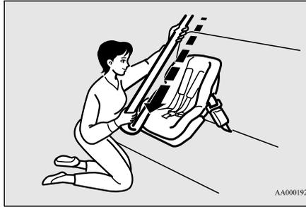
4. After the belt has retracted, tug on it. If the belt is in the ALR function, you will not be able to pull it out. If the webbing can be pulled out from retractor, the ALR function has not been activated and you will need to repeat steps 3 and 4.
