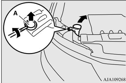
2. Turn the cap (B) counterclockwise to remove it.
