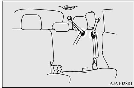
Put the seat belt webbing in the back slot (A) on the clip and insert the metal plate of the latch plate into the front slot (B) as shown in the illustration.
