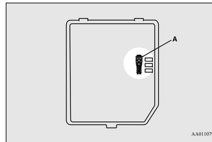
3. Clamp it on the fuse you wish to remove, and pull the fuse straight out from the fuse block.
