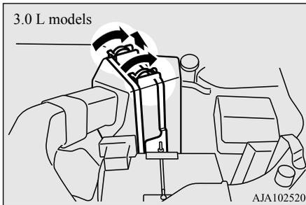
4. Replace the air cleaner filter and put the cover back on in its original position.
