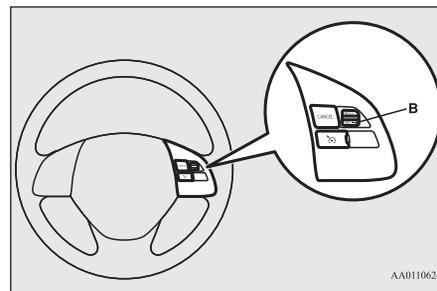
To slow down your speed in small amounts, push down the SET - switch (B) for less than about 1 second and release it.
