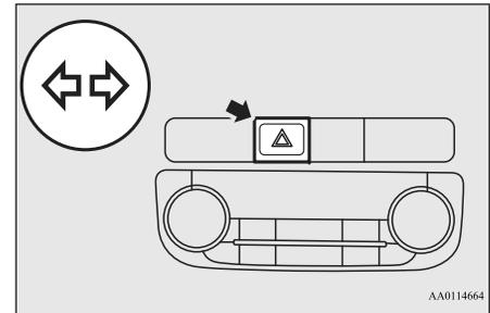
If you press the flasher switch, the front and rear turn signals will flash intermittently, and so will the hazard warning lights. This is an emergency warning system and should not be
