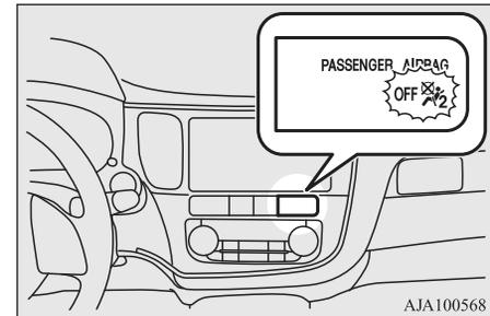
The indicator normally comes on when the ignition switch is turned to the "ON" position or the operation mode is put in ON, and goes out a few seconds later. In the following situations, the indicator will stay on to show that the passenger front airbag is not operational.
