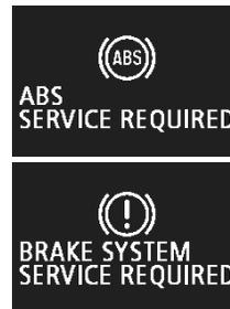
The anti-lock braking system and brake force distribution function may not work, so hard braking could make the vehicle unstable. Avoid hard braking and high-speed driving. Stop the vehicle in a safe place and contact an authorized Mitsubishi Motors dealer or repair facility of your choice.
