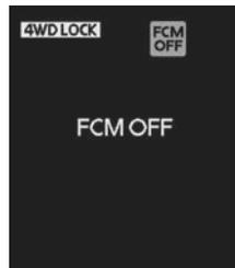
To turn on the FCM again, press and hold the FCM switch. A buzzer will sound, the “FCM OFF” message and the
