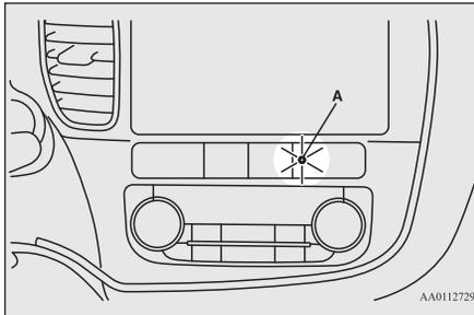
4. The system has entered the armed stage after about 20 seconds, when the theft-alarm indicator (A) flashing becomes slower.
