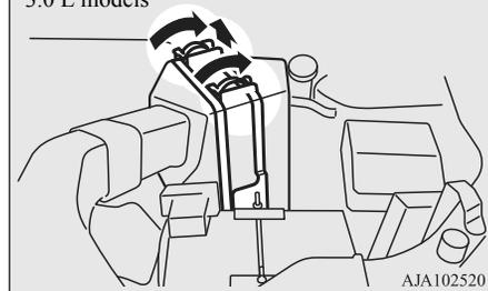
4. Replacing the air cleaner filter and put the cover back on in its original position.
