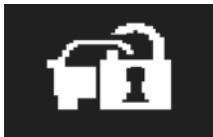
When registration of ID code is complete, the buzzer will sound 3 times and the immobilizer display will come on for 30 seconds.
