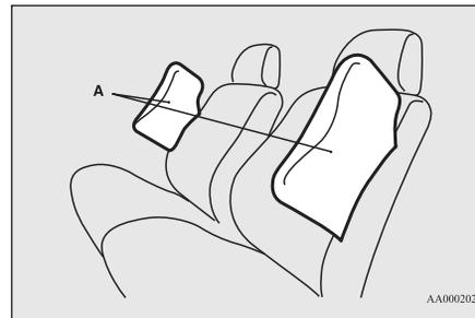
A label is attached to the seatbacks in vehicles equipped with side airbags.
