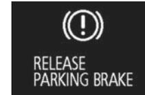
This warning is displayed if the vehicle is being driven with the parking brake still applied. The warning light in the instrument cluster only comes on when the parking brake is applied.
