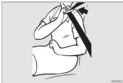
3. Pull the seat belt out slowly while holding the latch plate. Push the latch plate into the buckle until you hear a "click". Pull up on the belt to be sure the latch plate is locked securely in the buckle.
