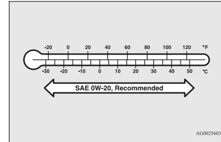
SAE 0W-20 engine oil is strongly recommended for optimum fuel economy and cold starting.
