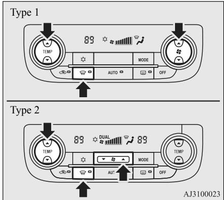
1. Push the defogger switch to change to the “” position.
