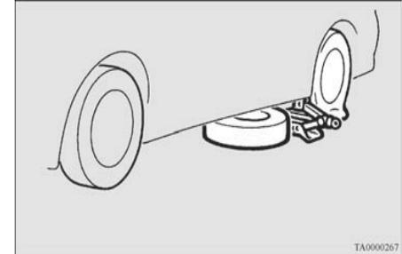
3. Rotate the jack by hand until the flange portion (B) fits in the groove (C) at the top of the jack.
