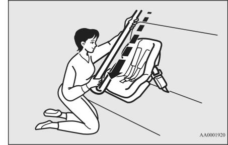
5. After confirming that the belt is locked, grab the shoulder part of the belt near the buckle and pull up to remove any slack from the lap part of the belt allowing the slack to feed into the retractor. Remember, if the lap belt portion is not tight, the child restraint system will not be secure. It may help to put your weight on the child restraint system and/or push on its seat-back while pulling up on the belt (See illustration).
