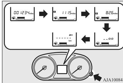
2. Press and hold the multi information display switch for about 2 seconds or more to make the spanner mark start flashing. (If there is no operation for about 10 seconds with flashing, the display will revert to its original indication.)
