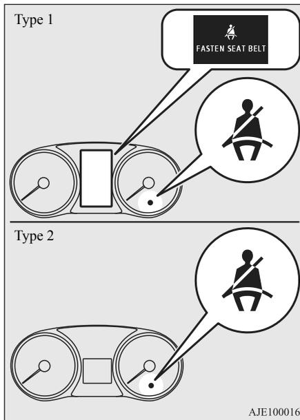
A tone and warning light are used to remind the driver to fasten the seat belt.
