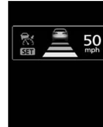
You can set the speed anywhere from approximately 25 mph (40 km/h) to 110 mph (180 km/h).
