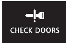
When the ignition switch is in the “LOCK (PUSH OFF)” position, and someone tries to lock the vehicle by pressing the driver’s or front passenger’s door lock/unlock switch, or the tailgate LOCK switch while one of the doors or the tailgate is not fully closed, the warning display is displayed and the buzzer sounds for about 3 seconds as a warning, and the doors and the tailgate cannot be locked.
