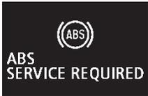
If there is a malfunction in the system, the anti-lock braking system warning light will come on and the warning display will appear on the information screen in the multi-information display.
