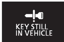
When the ignition switch is in the “LOCK (PUSH OFF)” position, the F.A.S.T.-key is left in the passenger compartment, all the doors and the tailgate are closed, and someone tries to lock the vehicle by pressing the driver’s or front passenger’s door lock/unlock switch, or the tailgate LOCK switch, the warning display is displayed and the buzzer sounds for about 3 seconds as a warning, and the doors and the tailgate cannot be locked.
