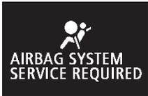
Under normal conditions, the warning light comes on when the ignition switch is turned to the “ON” position and goes off a few seconds later.
