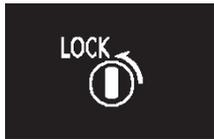
If the driver's door is opened while the ignition switch is in a position other than "LOCK" (PUSH OFF), the ignition switch return reminder buzzer will sound intermittently to remind you to return the ignition switch to the "LOCK" (PUSH OFF) position.
