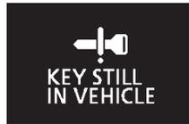
When the ignition switch is in the “LOCK (PUSH OFF)” position, the F.A.S.T.-key is left in the passenger compartment, all the doors and the tailgate are closed, and someone tries to lock the vehicle by pressing the LOCK switch of the doors and the tailgate, the warning display is displayed and the buzzer sounds for about 3 seconds as a warning, and the doors and the tailgate cannot be locked.
