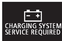
If there is a fault in the charging system, the warning display warning is displayed on the information screen in the multi-information display. The warning light in the instrument cluster also illuminates.
