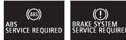
The anti-lock braking system and brake force distribution function may not work, so hard braking could make the vehicle unstable.
