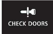
When the ignition switch is in the “LOCK (PUSH OFF)” position, and someone tries to lock the vehicle by pressing the LOCK switch of the doors and the tailgate while one of the doors or the tailgate is not fully closed, the warning display is displayed and the buzzer sounds for about 3 seconds as a warning, and the doors and the tailgate cannot be locked.
