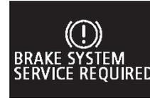
When the ignition switch is turned to the “ON” position, if the brake fluid is low, this warning is displayed. The warning light in the instrument cluster also illuminates.
