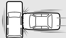
When the vehicle detects rollover of the vehicle (Curtain airbag only)
