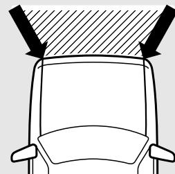
The front airbags and driver's knee airbag are designed to deploy when the vehicle suffers a moderate to severe frontal impact. A typical condition is shown in the illustration to the left.
