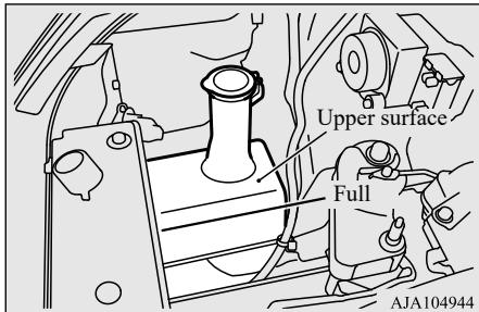
When freezing weather is anticipated, flush out the water in the reservoir by operating the pump. Fill the reservoir with windshield anti-freeze (not radiator antifreeze), and operate the system for a few seconds to flush out the residual water.
