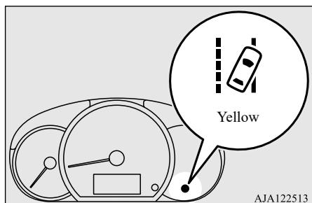
If the warning light remains even after the ignition switch is turned to the “OFF” position and then turned back to the “ON” position or the operation mode is put in OFF and then turned back to ON, contact your autho-
