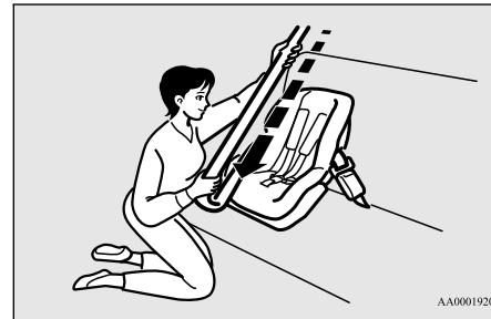
4. After the belt has retracted, tug on it. If the belt is in the ALR function, you will not be able to pull it out. If the webbing can be pulled out from retractor, the ALR function has not been activated and you will need to repeat steps 3 and 4.
