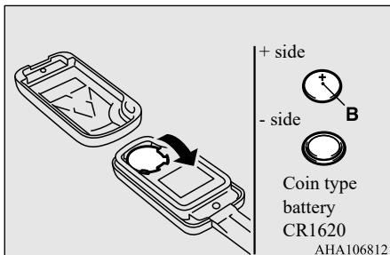
6. Close the remote control transmitter firmly.
