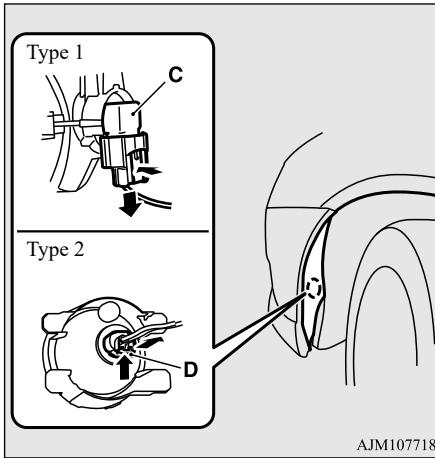
4. Turn the bulb counterclockwise to remove it.
