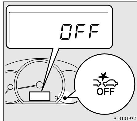
To turn on the FCM again, press and hold the FCM ON/OFF switch. The
