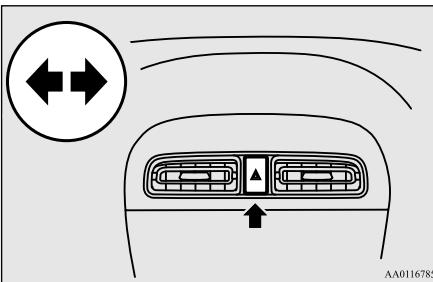
If you press the flasher switch, the turn signals will flash intermittently, and so will the hazard warning lights. This is an emergency warning system and should not be used when the vehicle is in motion, except for emergencies.
