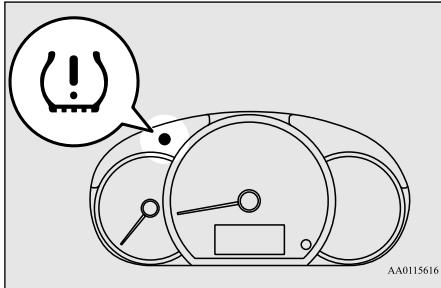
When the ignition switch is turned to the "ON" position or the operation mode is put in ON, the tire pressure monitoring system warning light normally illuminates and goes off a few seconds later.
