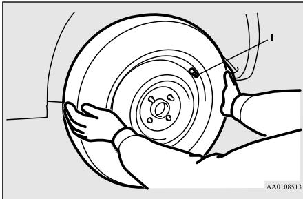
7. Install the wheel nuts with their tapered ends facing inward, then tighten by hand until the wheel is no longer loose.
