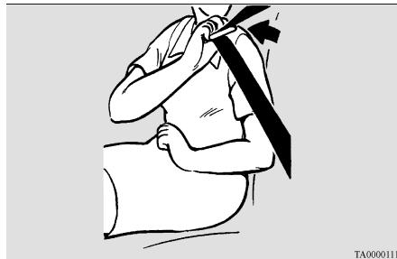
4. The lap part of the belt must always be worn low and snug across the hips. Pull up on the shoulder portion of the belt to take up any slack in the lap belt.
