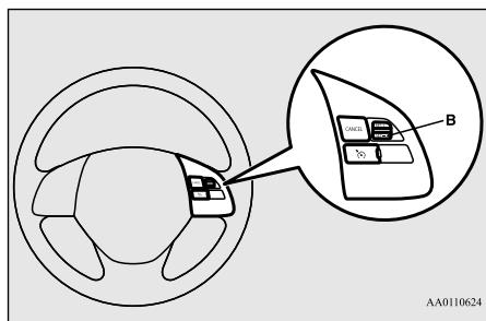
To slow down your speed in small amounts, press the SET - switch for less than about 1 second and release it.
