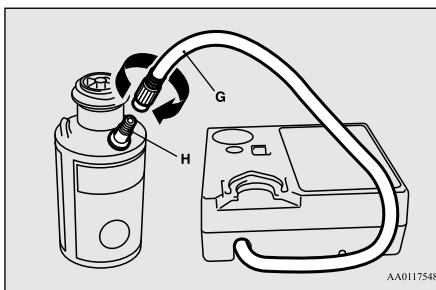
10. Install the bottle onto the compressor.
