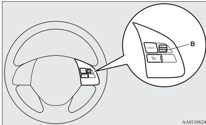
To slow down your speed in small amounts, press the SET - switch for less than about 1 second and release it.
