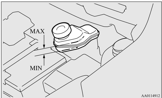
The fluid level falls slightly with wear of the brake pads, but this does not indicate any abnormality.
