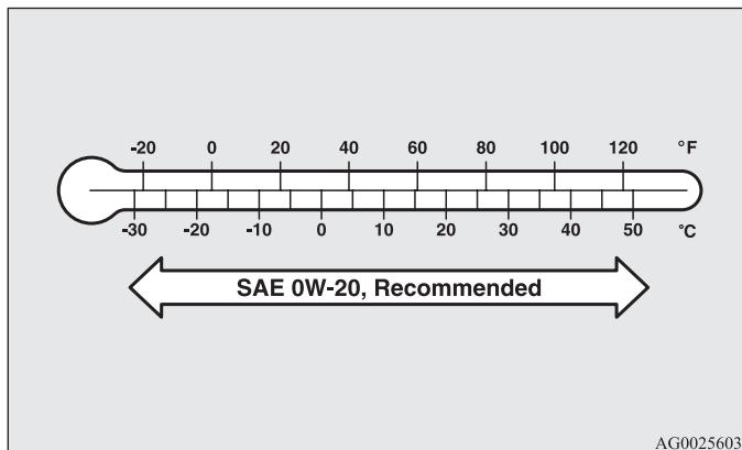
SAE 0W-20 engine oil is strongly recommended for optimum fuel economy and cold starting.
