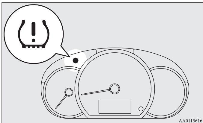
When the ignition switch is turned to the “ON” position or the operation mode is put in ON, the tire pressure monitoring system warning light normally illuminates and goes off a few seconds later.
