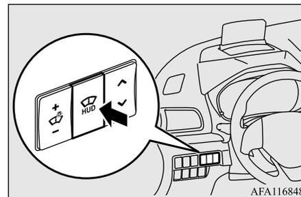
2. The setting top screen will be displayed if the vehicle is stopped, push the switch again.
