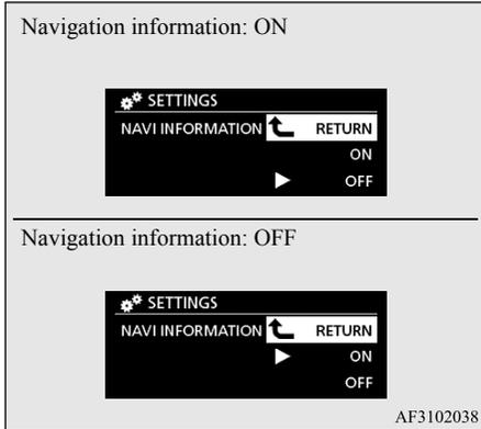
7. Push again the
