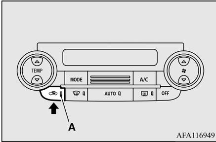
**7** When the air conditioning turns on, the air selection is controlled automatically. When the air conditioning turns off, the air selection automatically goes back to the outside position.
