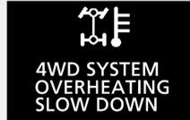
Reduce speed and, if the indicator stops blinking, you may resume normal driving.
