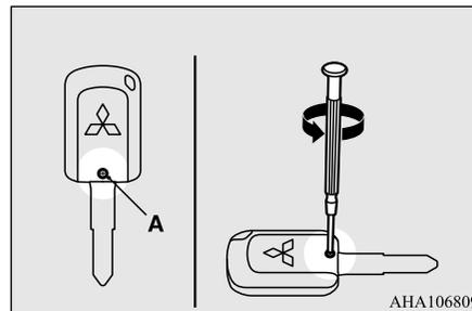
3. With the Mitsubishi mark facing you, insert the cloth-covered tip of a flat blade screwdriver into the notch in the key case and use it to open the case.
