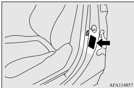
This placard shows the maximum number of occupants permitted to ride in your vehicle as well as “the combined weight of occupants and cargo” (A), which is called the vehicle capacity weight. The weight of any non-factory installed options, as well as the tongue weight of a trailer being towed and roof load is included in the definition of “cargo” when determining the vehicle capacity
