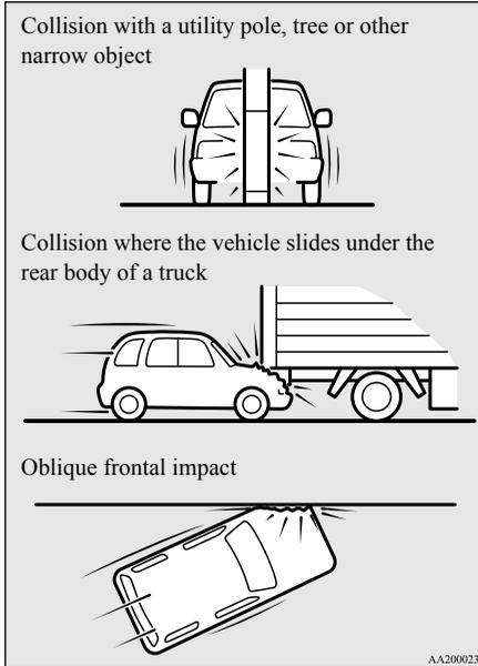
**The front airbags and driver's knee airbag ARE NOT DESIGNED TO DEPLOY when**
