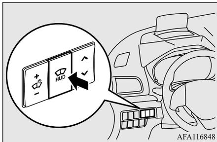
2. The setting top screen will be displayed, push and hold the
