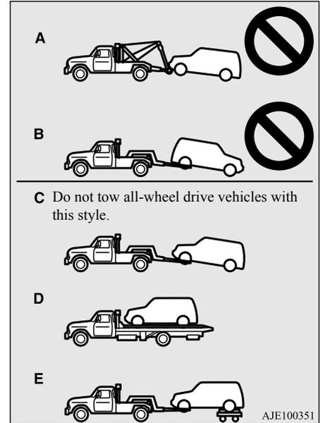
**Towing the vehicle by a tow truck**
