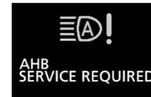
[When the sensor is malfunctioning]
