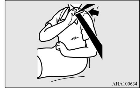
5. Pull the seat belt out slowly while holding the latch plate. Push the latch plate into the buckle until you hear a "click". Pull up on the belt to be sure the latch plate is locked securely in the buckle.
