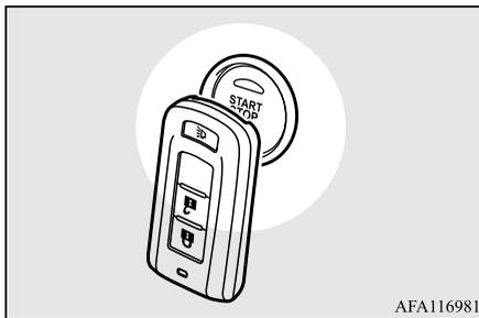
When registration of ID code is complete, the buzzer will sound three times and the immobilizer display will come on for 30 seconds.
