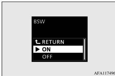
If you turn the BSW ON/OFF, the Rear Cross Traffic Alert (RCTA) also turns ON/OFF at the same time.
