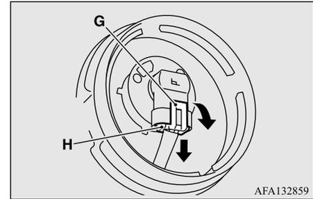
6. Turn the bulb (I) counterclockwise to remove it.
