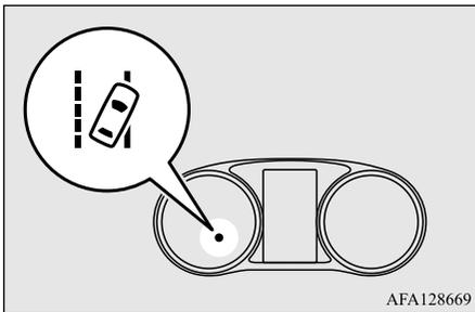
To turn the LDW back on, press the LDW switch again. The LDW indicator in the instrument cluster will then come on.
