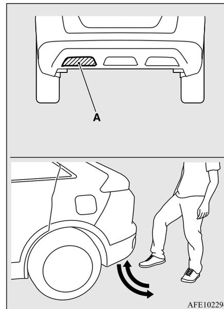
While carrying the F.A.S.T.-key within the operating range of the F.A.S.T.-key, if you make a kicking motion to move your foot underneath the lower-left trapezoid shaped section of the rear bumper (where the sensor is fitted) and then withdraw your foot, the warning buzzer sounds, the turn signal lights blink, and the power remote liftgate operates as follows:
