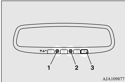
Normally, use the automatic mode. When the operation mode is put in ON, the green indicator (1) illuminates and the reflection factor of the mirror is automatically changed.
