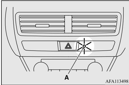
4. The system has entered the armed stage after approximately 20 seconds\*, when the theft-alarm indicator (A) blinking becomes slower.
