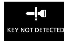
Warning display (when the engine switch is pressed two times or more)
