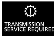
When the warning display or the warning display appears on the information screen in the multi-information display while you are driving, there could be a malfunction in the CVT.
