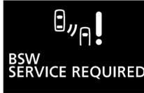
When the warning display appears, the BSW does not operate normally because there is a malfunction in the system. Have the vehicle inspected at an authorized Mitsubishi Motors dealer as soon as possible.
