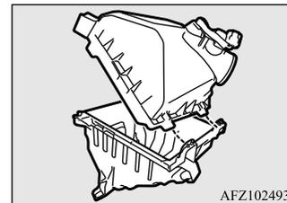
3. Put the duct back on in its original position.
