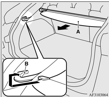
2. Remove the cover (A) from the mounting grooves (B), and the cover will be rolled back into the retracted position.
