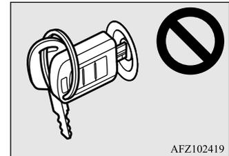
In cases like the above, move the offending object(s) away from the key and turn the key back to the “ACC” or “OFF” position. Then try to start the engine again. If the engine does not start, contact an authorized Mitsubishi Motors dealer.
