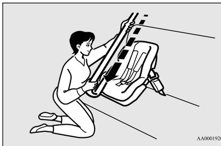
7. After the belt has retracted, tug on it. If the belt is in the ALR function, you will not be able to pull it out. If the webbing can be pulled out from retractor, the ALR function has not been activated and you will need to repeat steps 6 and 7.
