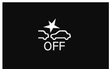
To turn on the FCM again, press the FCM ON/OFF switch. The
