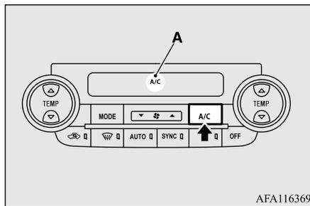
Push the switch again and the air conditioning compressor will stop and the indicator goes off.
