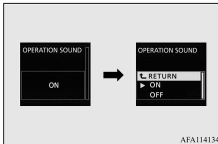
3. Press the  $\checkmark$  switch or  $\wedge$  switch to select the sound, and then press the  $\text{☰}$  switch to confirm the setting. The setting is changed to the selected condition.
