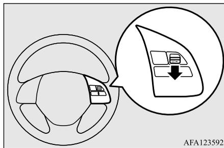
To slow down your speed in small amounts, push down the “SET -” switch for less than approximately 1 second and release it.
