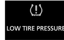
**Tire pressure monitoring system warning light / display**
