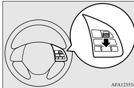
The set indicator comes on, the set speed is indicated and the following distance indicator changes to the active display.
