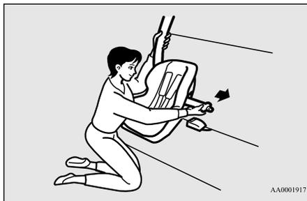
6. To activate the ALR child restraint installation function, slowly pull the shoulder part of the belt all the way out of the retractor until it stops. Then let the belt feed back into the retractor.
