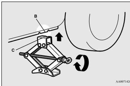
4. Check that the flange portion at the jacking point fits in the groove at the top of the jack.
