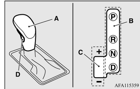
In the main gate, selector lever has four positions, and is equipped with a lock button (D) to avoid inadvertent selection of the wrong gear.
