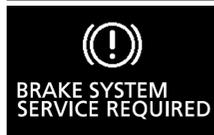
The anti-lock braking system and brake force distribution function may not work, so hard braking could make the vehicle unstable.
