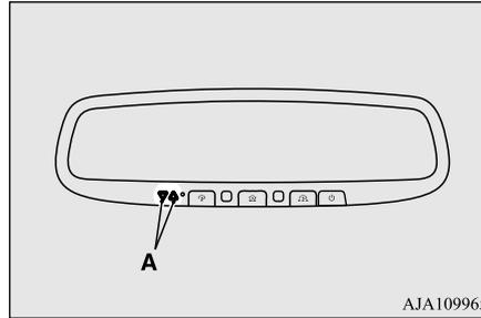
1. Within 5 seconds after successfully programming the garage door opener (refer to “Programming a new HomeLink®,” section), both garage door operation indicators (A) will flash rapidly green indicating that the garage door feedback has been enabled.
