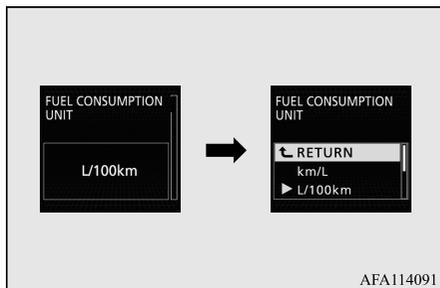
3. Press the  $\blacktriangledown$  switch or  $\blacktriangle$  switch to select the units, and then press the  $\text{☰}$  switch to confirm the setting.
