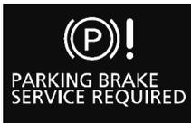
If there is a malfunction in the system, the warning light will come on. In addition, the warning display appears on the information screen in the multi-information display.
