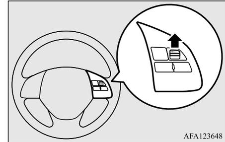
To increase your speed in small amounts, push up the “RES +” switch for less than approximately 1 second and release it. Each time you push up the “RES +” switch, your vehicle will go approximately 1 mph (1.6 km/h) faster.
