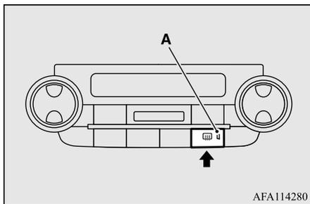
After approximately 15 to 20 minutes of operation, the system will shut off automatically.
