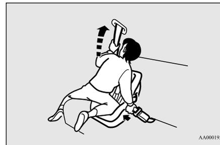
9. Push and pull the child restraint system in all directions to check that it is installed securely.
