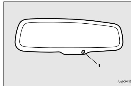
When the operation mode is put in ON, the reflection factor of the mirror is automatically changed.
