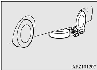
3. Rotate the jack by hand until the flange portion (B) fits in the groove (C) at the top of the jack.
