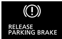
This warning is displayed if the vehicle is being driven with the parking brake still applied. The brake warning light in the instrument cluster only comes on when the parking brake is applied.
