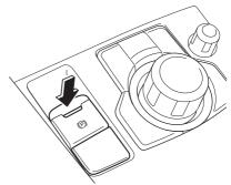
Firmly depress the brake pedal and press the electric parking brake switch. If the electric parking brake switch is pressed without depressing the brake pedal, the display or indicator light in the instrument cluster notifies the driver that the brake is not depressed.
