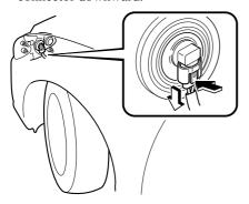
Turn the socket and bulb assembly to remove it. Carefully remove the bulb from its socket in the reflector by gently pulling it straight backward out of the socket.
