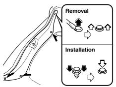
Pull the center of each plastic retainer and remove the retainers and the trunk side trim.
