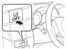
The Lane-keep Assist System (LAS) & Lane Departure Warning System (LDWS) indication (white) is displayed in the multi-information display, and the system goes on stand-by.
