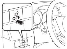
Drive the vehicle in the center of the driving lane while the Lane-keep Assist System (LAS) & Lane Departure Warning System (LDWS) OFF indicator light in the instrument cluster is turned off.
