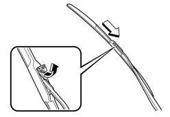
3. Tilt the blade assembly and remove it from the arm
