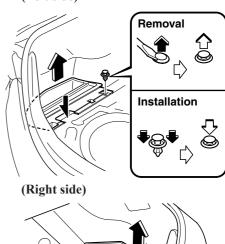
Pull the center of each plastic retainer and remove the retainers and the trunk end trim.
