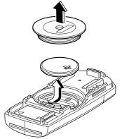
6. Insert a new battery with the positive pole facing up, and then cover the battery with the battery cap.
