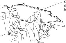
Only one side curtain air bag will deploy on the side of the vehicle that receives the force of an impact.
