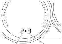
Selected gear position Suitable gear position
