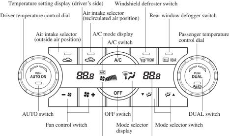
Airflow display Temperature setting display (Passenger's side)
