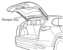
Do not modify or replace the liftgate damper stay. Consult an Authorized Mazda Dealer if a liftgate damper stay is deformed or damaged for reasons such as a collision or if there is some other problem.
