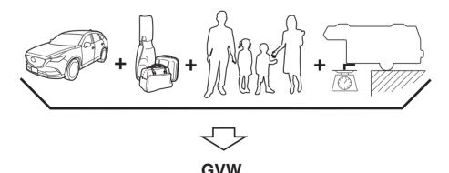
GVW (Gross Vehicle Weight) is the Vehicle Curb Weight + cargo + passengers.
