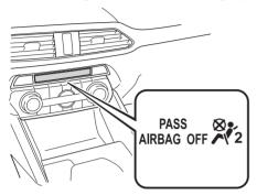
If the front passenger occupant classification sensor is normal, the indicator light turns on when the ignition is switched ON. The light turns off after a few seconds. Then, the indicator light turns on or is off under the following conditions:
