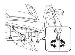
4. Pull the center of each plastic retainer and remove the retainers, and then partially peel back the mudguard.
