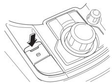
Firmly depress the brake pedal and press the electric parking brake switch. If the electric parking brake switch is pressed without depressing the brake pedal, the display or indicator light in the instrument cluster notifies the driver that the brake is not depressed.
