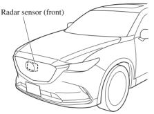
If "Front Radar Sensor Blocked" is displayed in the multi-information display of the instrument cluster, clean the area around the radar sensor (front).
