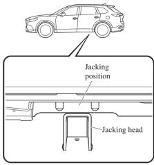
5. Continue raising the jack head gradually by rotating the screw with your hand until the jack head is inserted into the jack-up position.
