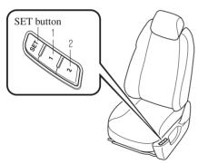
The driving position can be programmed or operated using the buttons on the side of the seat or the key.
