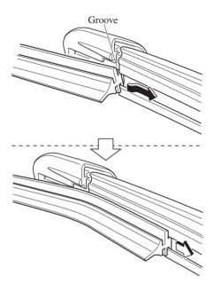
6. After pulling the blade rubber in the direction of the arrow and sliding the blade rubber to a position to check the blade holder groove, slide the blade rubber end in the opposite direction.
