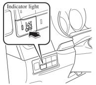
The Lane-keep Assist System (LAS) & Lane Departure Warning System (LDWS) indication (white) is displayed in the multi-information display, and the system goes on stand-by.
