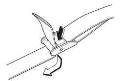
2. Hook the clips of the flat tire belts to the hooks under the third-row seat.
