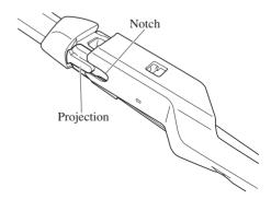
9. Slide the blade component and install it to the wiper arm.
