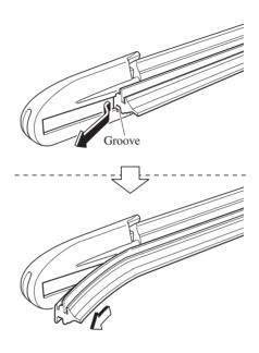
5. Insert the end of the new blade rubber into the groove of the blade holder until it contacts the end of the blade holder.
