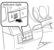
Drive the vehicle in the center of the driving lane while the Lane-keep Assist System (LAS) & Lane Departure Warning System (LDWS) OFF switch indicator light is turned off.
