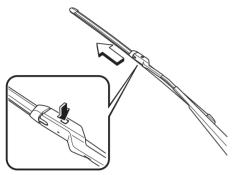
Pull the blade rubber in the direction of the arrow and slide it to a position where the blade holder groove can be checked.
