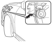
6. Turn the socket and bulb assembly counterclockwise and remove it.
