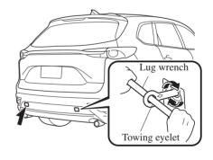
4. Hook the towing rope to the towing eyelet.
