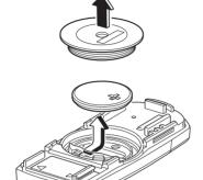
6. Insert a new battery with the positive pole facing up, and then cover the battery with the battery cap.
