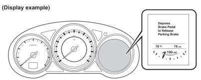
If the warning light turns on/flashes simultaneously or a symbol is indicated in the display, check the information regarding the warning light or symbol. (page 4-32)
