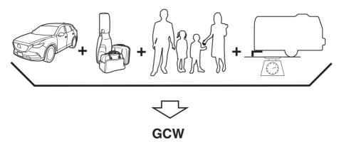
**GCW (Gross Combination Weight)** is the weight of the loaded vehicle (GVW) plus the weight of the fully loaded trailer.
