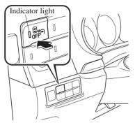
When the Blind Spot Monitoring (BSM) OFF switch is pressed, the Blind Spot Monitoring (BSM) and Rear Cross Traffic Alert (RCTA) systems are turned off and the Blind Spot Monitoring (BSM) OFF switch indicator light turns on.
