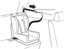
6. Push the child-restraint system firmly into the vehicle seat. Be sure the belt retracts as snugly as possible. A clicking noise from the retractor will be heard during retraction if the system is in the automatic locking mode. If the belt does not lock the seat down tight, repeat this step.
