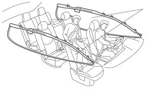
Both curtain air bags will deploy after the roll-over accident is detected.
