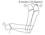
3. Make sure the seatback is securely latched by pushing it back until it is fully locked.
