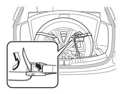
6. While pressing the flat tire against the third-row seat, pull the ends of the flat tire belts and secure the flat tire.
