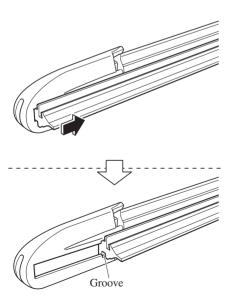
4. Pull the end of the blade rubber from the blade holder groove in the direction of the arrow and remove the blade rubber from the blade holder.
