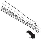
4. Remove the metal stiffeners from the blade rubber and install them in the new blade.
