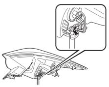
6. Turn the socket and bulb assembly counterclockwise and remove it.
