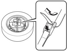
4. Pull the end of the flat tire belt and secure the sub-woofer and the wiring harness to the flat tire.
