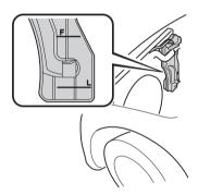
If it is at or near L, add enough coolant to the coolant reservoir to provide freezing and corrosion protection and to bring the level to F.
