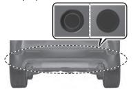
The ultrasonic sensors are mounted in the rear bumper.
