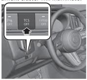
Press the switch again to turn the TCS back on. The TCS OFF indicator light\* will turn off.
