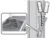
1. Forward sensing camera (FSC)
