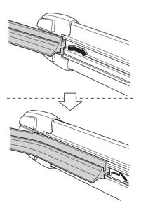
After pulling the blade rubber in the direction of the arrow and sliding the blade rubber to a position to check the blade holder groove, slide the blade rubber end in the opposite direction.
