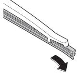
Remove the metal stiffeners from the blade rubber and install them in the new blade.
