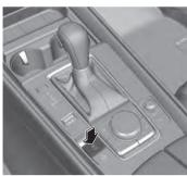
If the EPB switch is pressed without depressing the brake pedal, a message is displayed on the multi-information display to notify the driver to depress the brake pedal.
