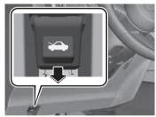
2. Insert your hand into the hood opening, slide the latch lever in the direction of the arrow as shown in
