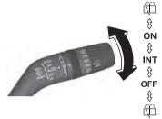
Turn the wiper on by turning the rear wiper/washer switch.
