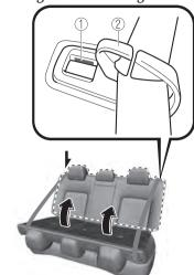
2. Press the seatback rearward and lock it in place. After returning the seatback to its upright position, make sure it is securely locked.
