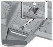
1. Tilt/Slide switch When pulling the tilt/slide switch rearward 1 time, the sunshade opens and when pressing the tilt/slide switch forward 1 time, it closes.
