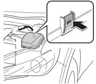
3. If any fuse but the MAIN fuse is blown, replace it with a new one of the same amperage rating.
