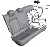
5. Push the child-restraint system firmly into the vehicle seat. Be sure the belt retracts as snugly as possible. A clicking noise from the retractor will be heard during retraction if the system is in the automatic locking mode. If the belt does not lock the seat down tight, repeat this step.
