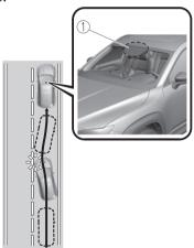
1. Forward sensing camera (FSC)
