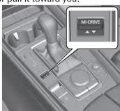
2. While checking the list displayed in the instrument cluster, push the Mi-Drive switch forward or pull it toward you to select a drive mode.
