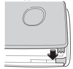
10.Insert the tabs of the lower cover into the slots of the transmitter and install the lower cover.
