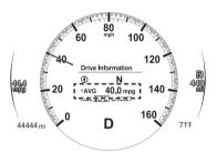
The average fuel economy can be reset by pressing the INFO switch for 1.5 seconds or more. After the data is cleared, the fuel consumption is recalculated and the - - - L/100 km (- - - mpg) for the 30 seconds prior to it being displayed is indicated.
