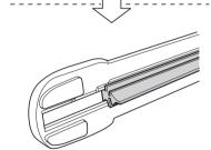
5. Pull the end of the blade rubber from the blade holder groove in the direction of the arrow and remove
