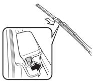
Pull the blade rubber in the direction of the arrow and slide it to a position where the blade holder groove can be checked.
