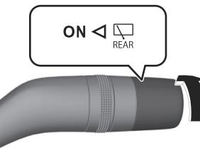
The wiper operates continuously.
