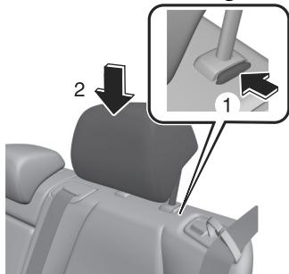
**Removing or Installing a Head Restraint**
