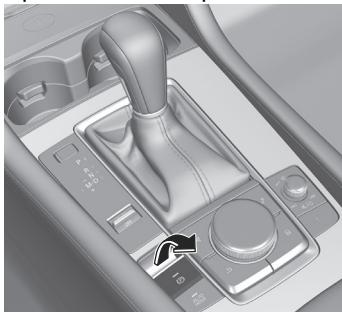
3. The parking brake is applied and the EPB indicator light <sup>(P)</sup> <sub>PARK</sub> in the instrument cluster and the EPB switch indicator light turn on.
