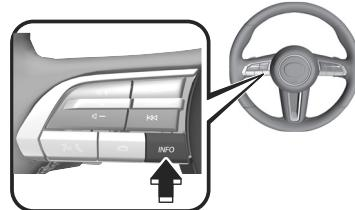
After resetting the data, - - - L/100 km (- - - mpg) is displayed until the average fuel economy is recalculated and displayed.
