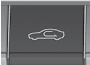
The mode is switched between recirculate mode and fresh air mode each time the switch is pressed. The display indicates whether recirculate mode (⟳) or fresh air mode (↔) is selected.
