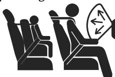
**Do not install a front-facing child-restraint system on the front passenger seat unless it is unavoidable.**
