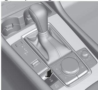
3. When the parking brake is released, the EPB indicator light <sup>(P)</sup> <sub>PARK</sub> in the instrument cluster and the EPB switch indicator light turn off.
