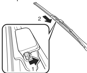
4. Pull out the end of the blade rubber from the notch at the end of the blade.
