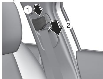
2. Make sure that the seat belt anchor adjuster is securely locked.
