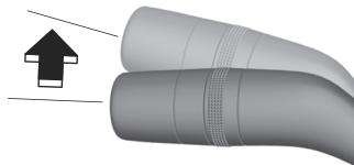
The headlights are switched to high beams and the headlight high-beam indicator light
