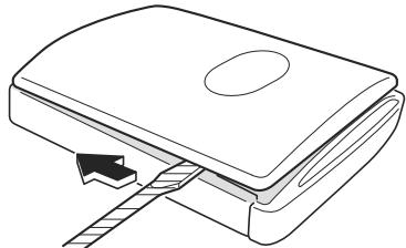
4. Twist the flathead screwdriver and remove the upper cover.
