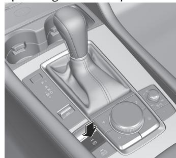
After the parking brake auto operation is canceled, a warning sound is activated one time, and the EPB switch indicator light switches from illumination to flashing, and then turns off after a certain period of time has passed.
