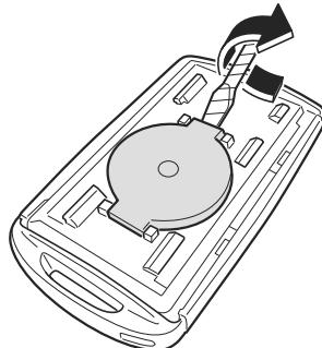
6. Remove the battery using the tape-wrapped flathead screwdriver.
