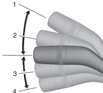
While the lever is in the 2 or 3 position, each turn signal light flashes and the turn signal light
