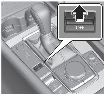
2. When the sport mode is selected, the select mode indicator light **SPORT** turns on in the instrument cluster.
