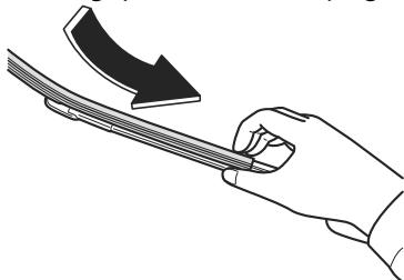
7. When all of the blade rubber is inserted, adjust the position.
