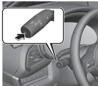
When the HBC is canceled, the HBC indicator light (green)
