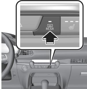
3. The rear window defogger operates and the switch indicator light turns on.
