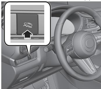
The Off-Road Traction Assist operates and the Off-Road Traction Assist indicator light
