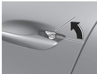
5. Attach the auxiliary key to its original position.
