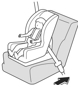
6. Push the child-restraint system firmly into the vehicle seat. Be sure the belt retracts as snugly as possible. A clicking noise from the retractor will be heard during retraction if the system is in automatic locking mode. If the belt does not lock the seat down tight, repeat the previous step and also this one.
