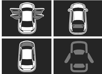
The light turns on if any door/liftgate/hood is not closed securely.
