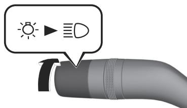
The headlights, parking lights, taillights, side-marker lights, and the license plate lights turn on, and the parking lights indicator light
