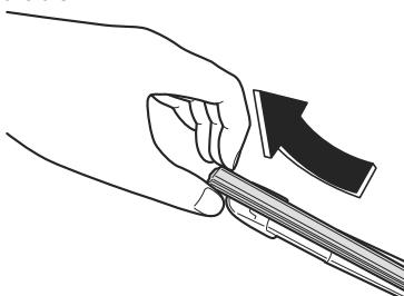
5. Remove the blade rubber by pulling it out as it is or by peeling it off toward the opposite side.
