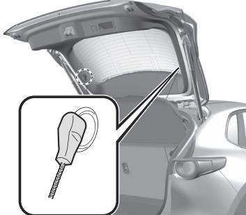
2. Press the luggage compartment cover upward from near the pins and remove the luggage compartment cover from the pins.
