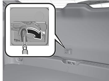
The liftgate is unlocked.
