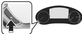
The display changes each time the TRIP switch is pressed.
