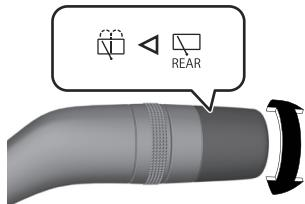
While the switch is in the position, the washer fluid is sprayed and the wiper operates.
