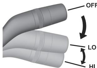
In the LO position, the windshield wipers operate at low speed. In the HI position, the wipers operate at high speed.
