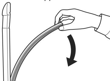
6. Insert a new blade rubber through the notch at the end of the blade. When inserting the blade rubber, do not grip the blade body tightly.
