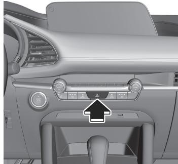
All the turn signal lights flash and the turn signal light
