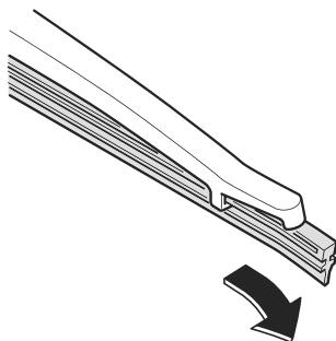
5. Remove the metal stiffeners from the blade rubber and install them in the new blade rubber.
