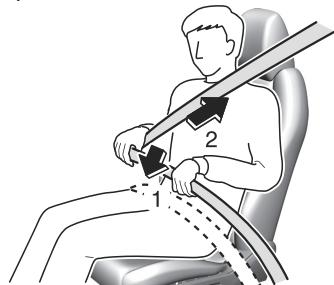
6. The belt should not touch the neck, jaw, or face and it should pass over the shoulder.
