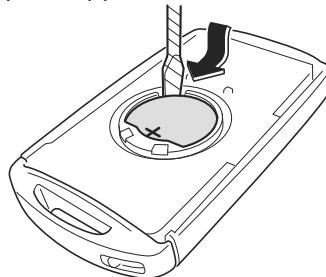
7. Insert a new battery into the key so that the positive pole is facing up.
