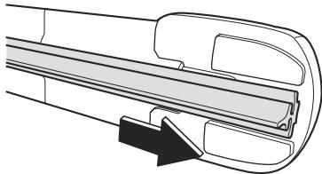
8. Make sure that the blade rubber is correctly installed to the blade holder.
