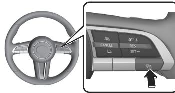
When the system is on, the MRCC standby indication (white)
