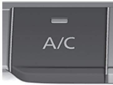
The cooling/dehumidifying function switches between on and off each time the switch is pressed. The indicator light turns on while the function is operating.
