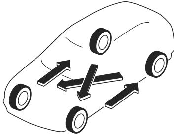
Do not include (TEMPORARY USE ONLY) spare tire in rotation. Also, inspect them for uneven wear and damage. Abnormal wear is usually caused by one or a combination of the following:
