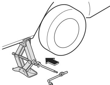
7. Turn the jack handle clockwise and raise the vehicle high enough so that the spare tire can be installed. Before removing the lug nuts, make sure your Mazda is firmly in position and that it cannot slip or move.
