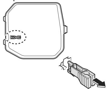
4. Inspect the fuse and replace it if it is blown.
