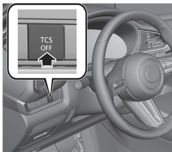
The TCS operation is canceled and the TCS OFF indicator light
