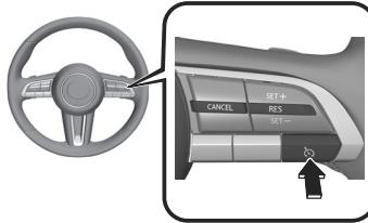
When the system is on, the cruise control standby indication (white)
