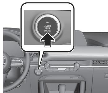
5. The engine starts and the KEY indicator light (green)
