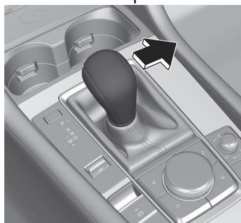
Manual shift mode is canceled and the manual shift mode indication and the gear position indication in the instrument cluster turn off.
