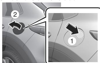
4. Slowly turn the fuel-filler cap. The fuel-filler cap opens.
