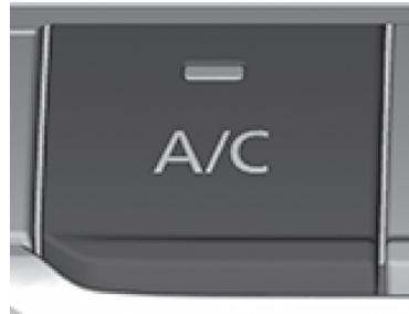
The cooling/dehumidifying function switches between on and off each time the switch is pressed. The indicator light turns on while the function is operating.
