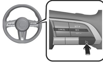
When the system is on, the cruise control standby indication (white)
