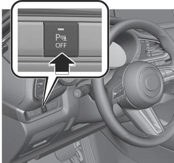
The parking sensors turn off and the parking sensor OFF switch indicator light turns on.
