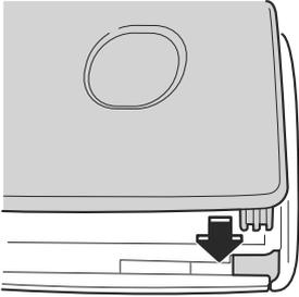
10. Attach the lower cover so that its tabs are inserted into the slots of the key.
