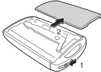
2. Remove the auxiliary key.
