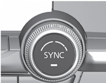
The mode switches between independent mode and interconnection mode each time the switch is pressed.
