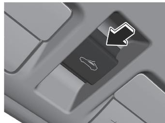
To stop it partway, press the tilt/slide switch.
