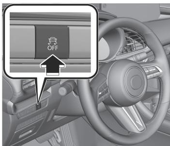
The TCS/DSC operation is canceled and the DSC OFF indicator light
