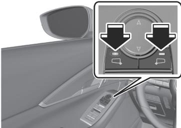
3. Press the adjustment switch to adjust the angle of the outside mirror.
