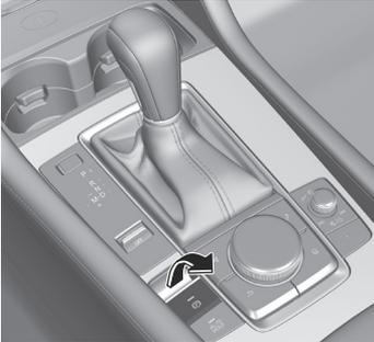
The parking brake is applied and the EPB indicator light
