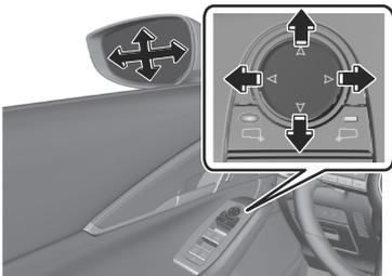
4. Press the select button on the side of the outside mirror that has been adjusted.
