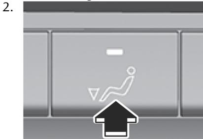
3. Set the air intake selector to the outside air position (indicator light turns off).
