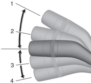
Each turn signal light flashes and the turn signal light
