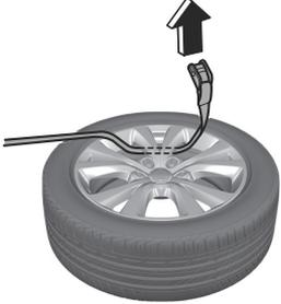
6. Thread the belt through the buckle, then pull the belt end to secure the flat tire.
