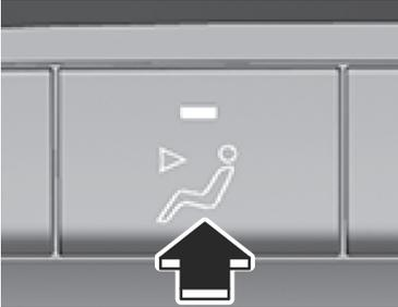
3. Set the air intake selector to the outside air position (indicator light turns off).
