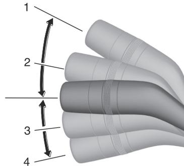
While the lever is in the 2 or 3 position, each turn signal light flashes and the turn signal light
