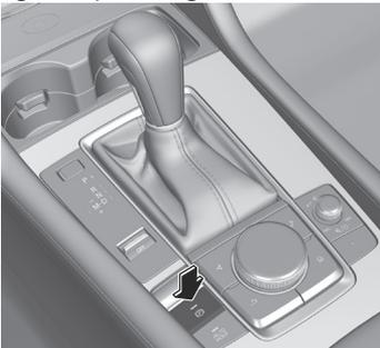
When the parking brake is released, the EPB indicator light
