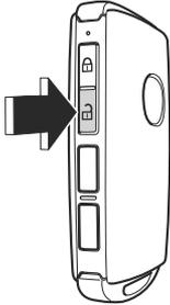
When the vehicle receives a key operation signal, the headlights, parking lights, taillights, side-marker lights, and the license plate lights turn on.
