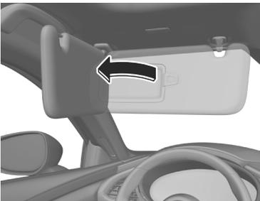
The visor extender\* extends the sunvisor's range of sun shading. To use, pull it out.
