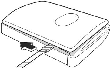
4. Twist the flathead screwdriver and remove the upper cover.
