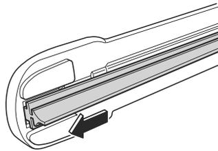
8. Make sure that the blade rubber is correctly installed to the blade holder.
