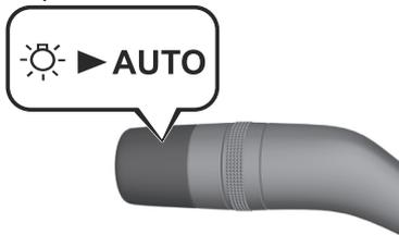
The daytime running lights turn on automatically when it is bright, and the headlights, parking lights, taillights, side-marker lights, and the license plate lights turn on automatically when it is dark.
