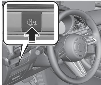
When the i-ACTIVSENSE mute switch is pressed while the following systems are operating, the warning sound deactivates.
