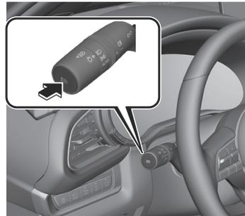
When the HBC is canceled, the HBC indicator light (green)
