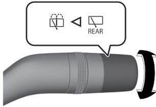
While the switch is in the
