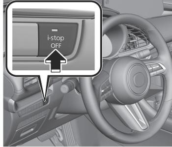
The i-stop function stops and the i-stop OFF switch indicator light turns on.
