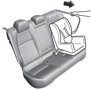
6. Push the child-restraint system firmly into the vehicle seat. Be sure the belt retracts as snugly as possible. A clicking noise from the retractor will be heard during retraction if the system is in the automatic locking mode. If the belt does not lock the seat down tight, repeat this step.
