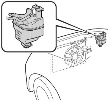
If it is at or near the LOW position, add enough coolant to the coolant
