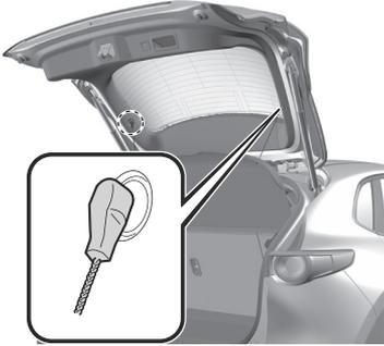
2. Press the luggage compartment cover upward from near the pins and remove the luggage compartment cover from the pins.
