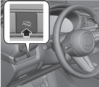
The Off-Road Traction Assist operates and the Off-Road Traction Assist indicator light
