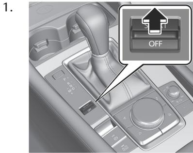
When the sport mode is selected, the select mode indicator light **SPORT** turns on in the instrument cluster.
