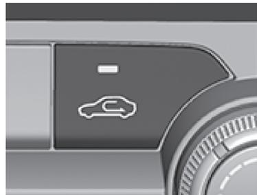
The mode is switched between recirculate mode and fresh air mode each time the switch is pressed.
