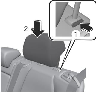
**Removing or Installing a Head Restraint**
