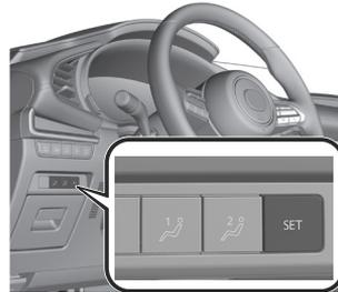
4. Do the following operation within 5 seconds after the sound is activated to program the driving position.
