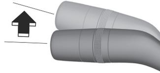
The headlights are switched to high beams and the headlight high-beam indicator light
