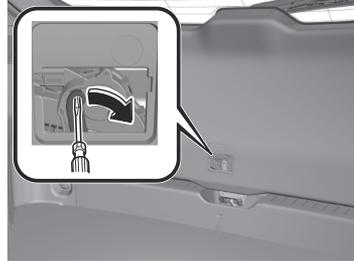
The liftgate is unlocked.
