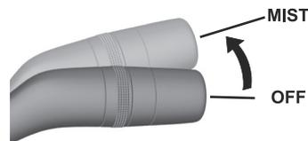
The windshield wipers operate while the lever is in the MIST position. Set the lever to the MIST position and immediately release it to operate the windshield wipers only once.
