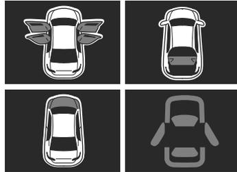
The light turns on if any door/liftgate/hood is not closed securely. In addition, the warning sound is activated if any door/liftgate is not closed and the vehicle is driven.
