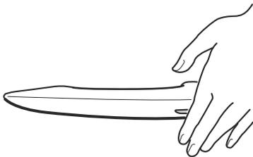
The following locations are locked by touching the sensing area of the door lock touch sensor.
