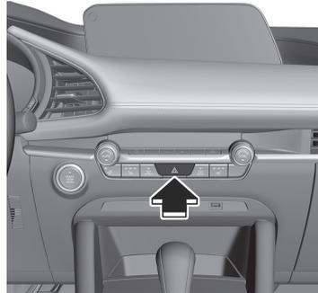
All the turn signal lights flash and the turn signal light
