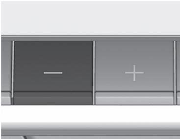
The airflow amount changes each time the switch is pressed. The airflow amount is indicated on the display. The airflow amount can be adjusted to 7 levels.
