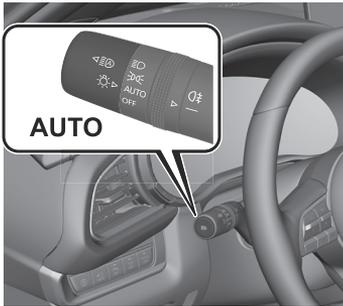
The HBC determines the surrounding conditions and operates automatically. When the HBC operates, the HBC indicator light (green)
