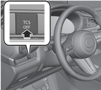
The TCS operation is canceled and the TCS OFF indicator light
