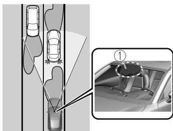
1. Forward Sensing Camera (FSC)\*<sup>1</sup>
