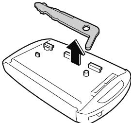
**Installing the auxiliary key**
