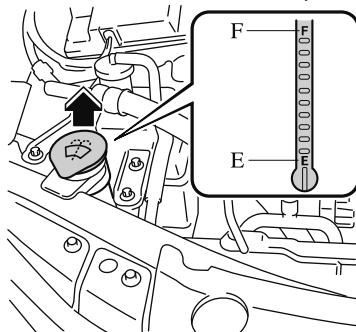
The top of the float should be between F and E.
