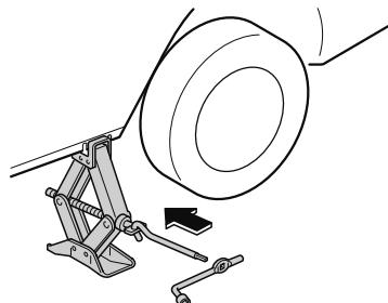
8. Turn the jack handle clockwise and raise the vehicle high enough so that the spare tire can be installed. Before removing the lug nuts, make sure your Mazda is firmly in position and that it cannot slip or move.
