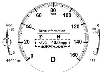
The average fuel economy and trip meters can be reset by pressing the INFO switch for 1.5 seconds or more while in each mode. After the data is cleared, the fuel consumption is recalculated and the - - - L/100 km ( - - - mpg) for the 1 minute prior to it being displayed is indicated.
