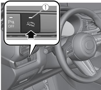
1. Off-Road Traction Assist switch indicator light
