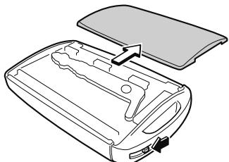
2. Remove the auxiliary key.
