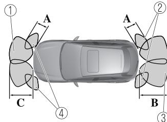
1. Front ultrasonic sensor detection range
