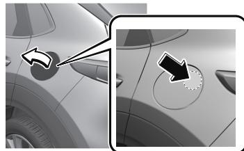
3. To remove the fuel-filler cap, turn it counterclockwise.
