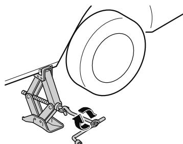
**WARNING****Do not jack up the vehicle higher than is necessary:**
