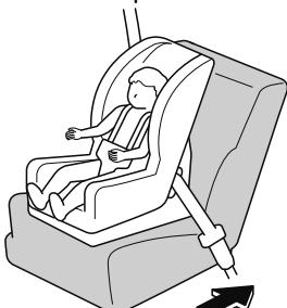
**Seating a child in a child-restraint system on the front passenger seat is dangerous under certain conditions (With Front Passenger Occupant Classification System):**
