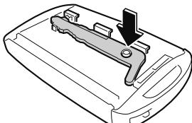
2. Insert the tabs of the lower cover into the slots of the transmitter and install the lower cover.
