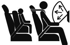
**Do not install a front-facing child-restraint system on the front passenger seat unless it is unavoidable:**
