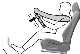
2. Adjust the steering wheel height so that the gauges can be viewed easily.
