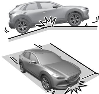
This vehicle is equipped with low profile tires allowing class-leading performance and handling. As a result, the sidewall of the tires are very thin and the tires and wheels can be damaged if driven through potholes or on rough/uneven roads at excessive speeds. Use care and reduce speed when traveling on rough/uneven roads or through potholes.
