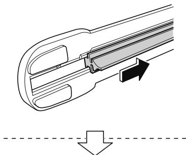
8. Make sure that the blade rubber is correctly installed to the blade holder.
