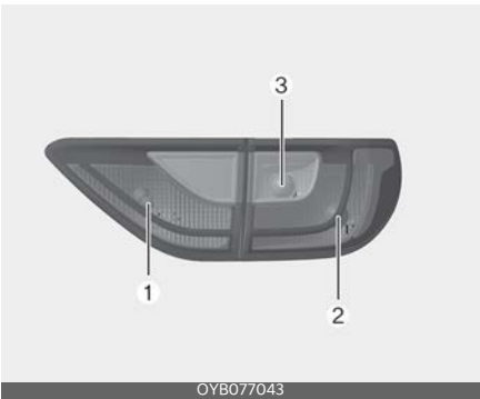
Rear combination lamp - Type B
