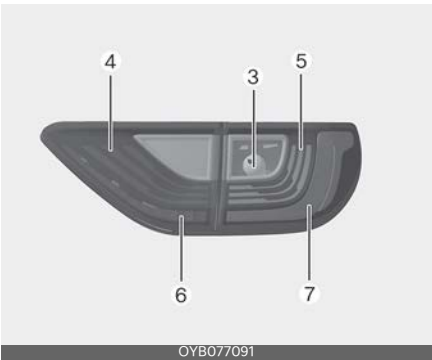
Rear combination lamp - Type B
