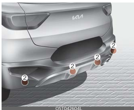
[2] : Rear ultrasonic sensors
