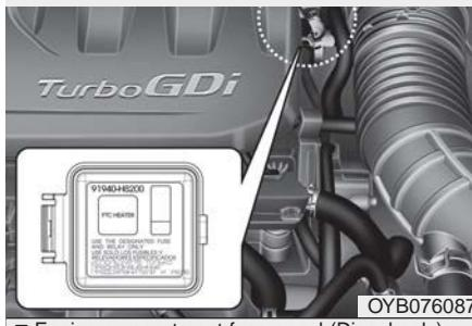
■ Engine compartment fuse panel (Diesel only)
