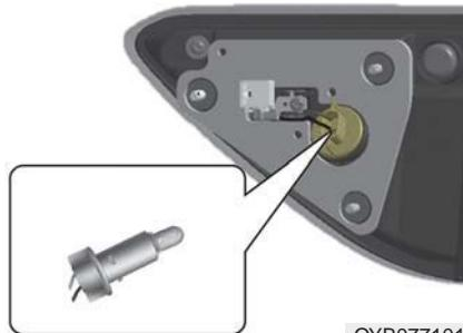
3. Remove the socket from the assembly by turning the socket counterclockwise until the tabs on the socket align with the slots on the assembly.
