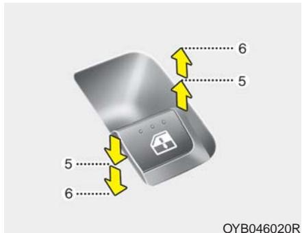
Pressing or pulling up the power window switch momentarily to the second detent position (6) completely lowers or lifts the window even when the switch is released. To stop the window at the desired position whilst the window is in operation, pull up or press and release the switch to the opposite direction of the movement.
