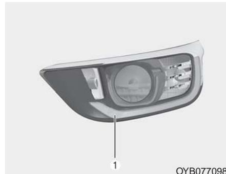
If the position lamp + DRL (LED) (1) does not operate, have your vehicle checked by a professional workshop.
