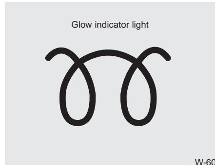
3. Turn the ignition switch to the ON position to pre-heat the engine. Then the glow indicator light will illuminate.
