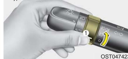
Fog lights are used to provide improved visibility when visibility is poor due to fog, rain or snow, etc. The fog lights will turn on when the fog light switch (1) is turned on after the parklight is turned on.
