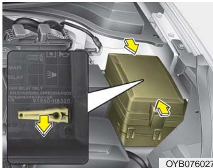
3. Pull the suspected fuse straight out. Use the removal tool provided in the main fuse box in the engine compartment.
