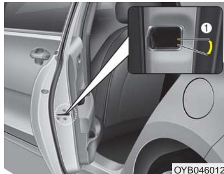
If the power door lock switch does not operate electrically, the only way to lock the door(s) is with the mechanical key from the outside key hole.
