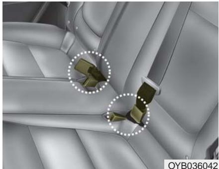
The rear seat belt buckles can be stowed in the pocket between the rear seatback and cushion when not in use.
