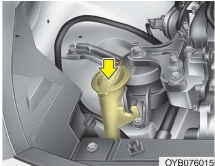
The reservoir is translucent so that you can check the level with a quick visual inspection.
