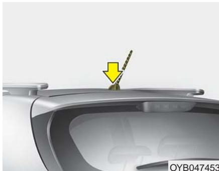
Your car uses a roof antenna to receive both AM and FM broadcast signals. This antenna is a removable type.
