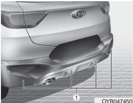
The reverse parking distance warning assists the driver during backward movement of the vehicle by chiming if any object is sensed within a distance of 120 cm (47 in.) behind the vehicle.
