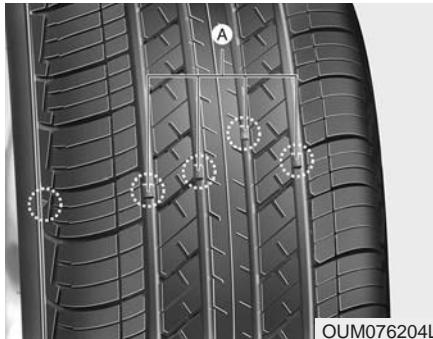
If the tyre is worn evenly, a tread wear Indicator (A) will appear as a solid band across the tread. This shows there is less than 1.6 mm (1/16 in.) of tread left on the tyre. Replace the tyre when this happens. Do not wait for the band to appear across the entire tread before replacing the tyre.
