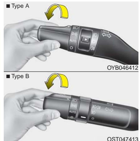
When the light switch is in the head-light position (3rd position), the head, tail, position, license and instrument panel lights are ON.
