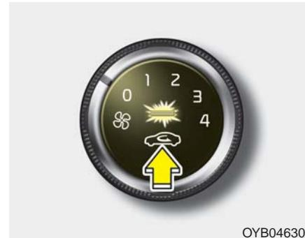
The air intake control is used to select the outside (fresh) air position or recirculated air position.
