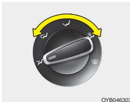
The mode selection knob controls the direction of the air flow through the ventilation system.
