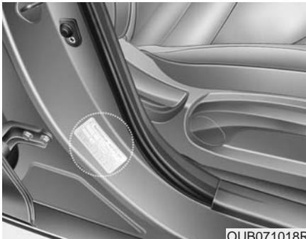
All specifications (sizes and pressures) can be found on a label attached to the driver's side centre pillar.
