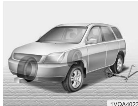
4. Remove the wheel lug nut wrench, jack, jack handle, and spare tyre from the vehicle.
