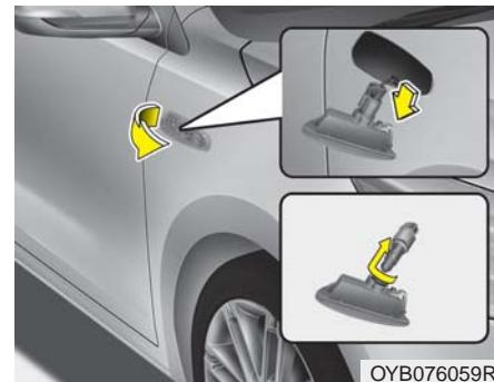
1. Remove the lamp assembly from the vehicle by prying the lens and pulling the assembly out.
