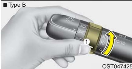
To turn the rear fog lights off, turn the rear fog light switch to the on position again.
