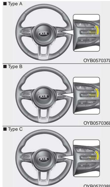
If any method other than the cruise /CRUISE/ button was used to cancel cruising speed and the system is still activated, the most recent set speed will automatically resume when you move the lever up (to RES+).
