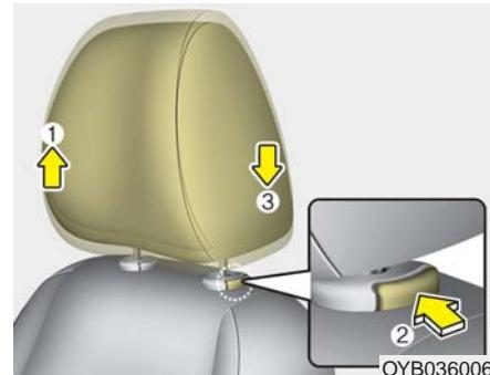
To raise the headrest, pull it up to the desired position (1). To lower the headrest, push and hold the release button (2) on the headrest support and lower the headrest to the desired position (3).
