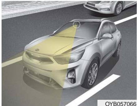
The Lane Keeping Assist (LKA) system detects the lane markers on the road with a front view camera at the front windscreens, and assists the driver's steering to help keep the vehicle in the lanes.
