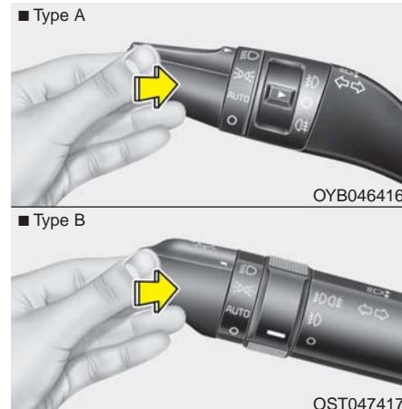
To turn on the high beam headlights, push the lever away from you. Pull it back for low beams.
