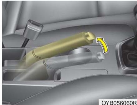
Check the stroke of the parking brake by counting the number of "clicks" heard whilst fully applying it from the released position. Also, the parking brake alone should securely hold the vehicle on a fairly steep grade. If the stroke is more or less than specified, have the system serviced by a professional workshop. Kia recommends to visit an authorised Kia dealer/service partner.
