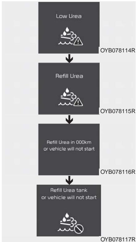
The lack warning messages of Urea solution appear below Urea solution approximately 3.6 L. When the warning message "Low Urea" is displayed with SCR warning lamp (⚠), the urea solution tank needs to be refilled. If not refilled for a considerable mileage, visual warning system will escalate the intensity by displaying the message "Refill Urea" with SCR warning lamp (⚠).
