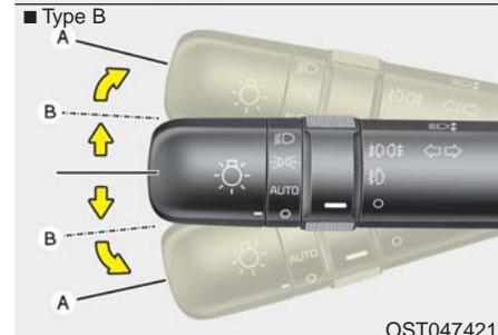
The ignition switch must be on for the turn signals to function. To turn on the turn signals, move the lever up or down (A).
