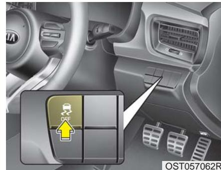
The Electronic Stability Control (ESC) system is designed to stabilize the vehicle during cornering manoeuvres. ESC checks where you are steering and where the vehicle is actually going.
