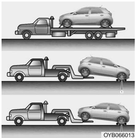
If emergency towing is necessary, we recommend having it done by an authorised Kia dealer or a commercial tow-truck service. Proper lifting and towing procedures are necessary to prevent damage to the vehicle. The use of wheel dollies (1) or flatbed is recommended.
