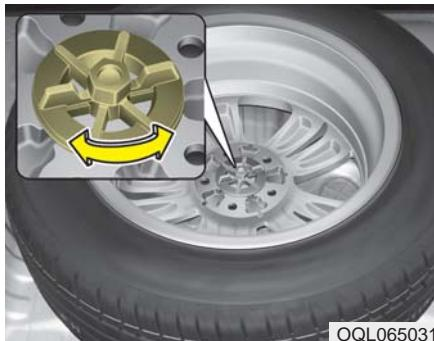
Turn the tyre hold-down wing bolt counterclockwise.
