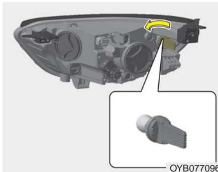
4. Insert a new bulb by inserting it into the bulb-socket and rotating it until it locks into place.
