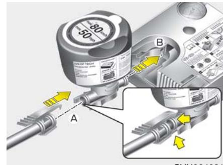
4. Connect the filling hose (3) onto the connector of the sealant bottle (A).
