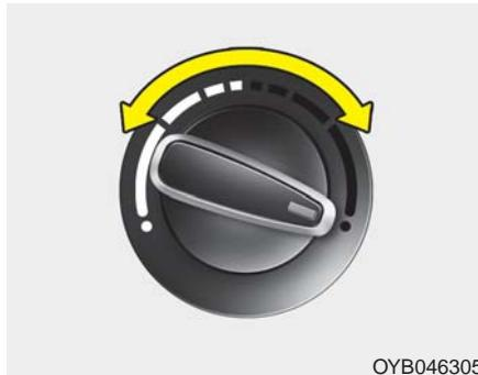
The temperature control knob allows you to control the temperature of the air flowing from the ventilation system. To change the air temperature in the passenger compartment, turn the knob to the right position for warm and hot air or left position for cooler air.
