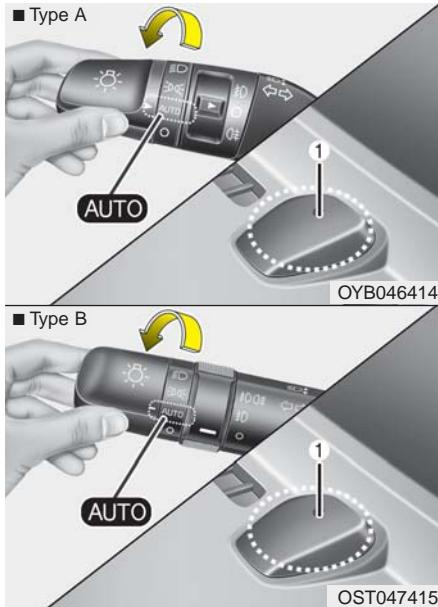
When the light switch is in the AUTO light position, the taillights and headlights will be turned ON or OFF automatically depending on the amount of light outside the vehicle.
