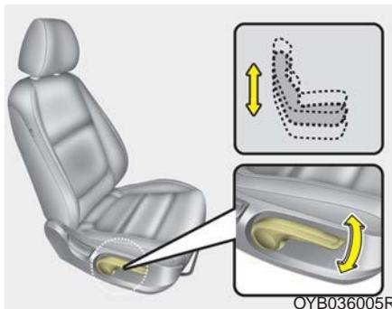
To change the height of the seat cushion, push the lever that is located on the outside of the seat cushion upwards or downwards.
