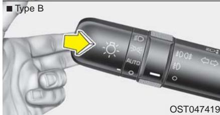
To flash the headlights, pull the lever towards you. It will return to the normal (low beam) position when released. The headlight switch does not need to be on to use this flashing feature.
