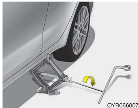
8. Insert the jack handle into the jack and turn it clockwise, raising the vehicle until the tyre just clears the ground. This measurement is approximately 30 mm (1.2 in). Before removing the wheel lug nuts, make sure the vehicle is stable and that there is no chance for movement or slippage.
