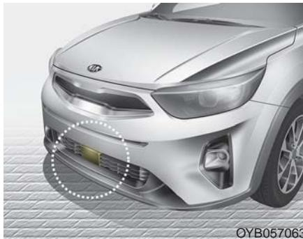
The sensor is to maintain a certain distance from the vehicle in front. However, the smudged sensor lens with foreign substances, such as snow and rain, adversely affects the sensing performance. It may even temporarily cancel the FCA. Always keep the sensor lens clean.
