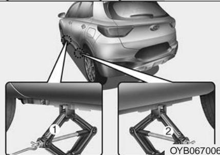
7. Place the jack at the front (1) or rear (2) jacking position closest to the tyre you are changing. Place the jack at the designated locations under the frame. The jacking positions are plates welded to the frame with two tabs and a raised dot to index with the jack.
