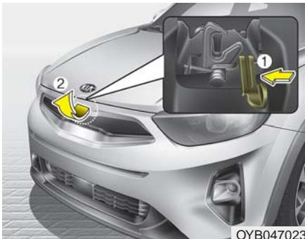
2. Go to the front of the vehicle, raise the bonnet slightly, push the secondary latch (1) inside of the bonnet centre and lift the bonnet (2).
