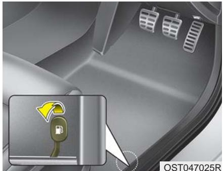
The fuel filler door must be opened from inside the vehicle by pulling up on the fuel filler door opener located on the front floor area on the driver's seat.
