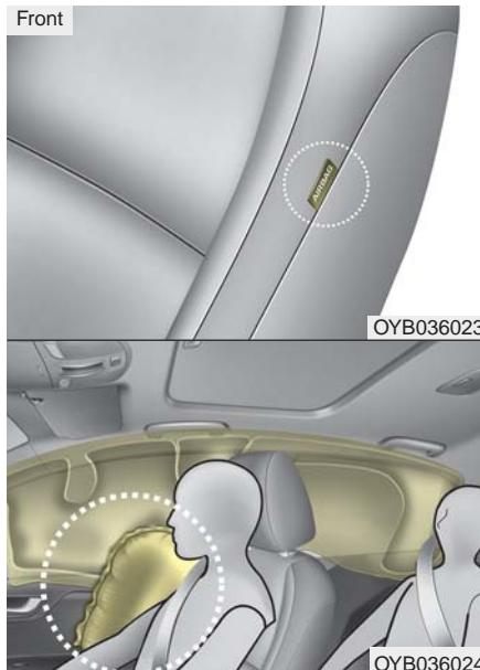
The side air bags are designed to deploy only during certain side-impact collisions, depending on the crash severity, angle, speed and point of impact. The side impact air bags are not designed to deploy in all side impact situations.
