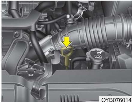
The automatic transmission fluid level should be checked regularly.
