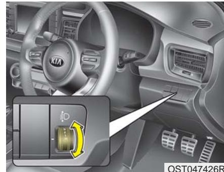
To adjust the headlight beam level according to the number of the passengers and loading weight in the luggage area, turn the beam levelling switch.
