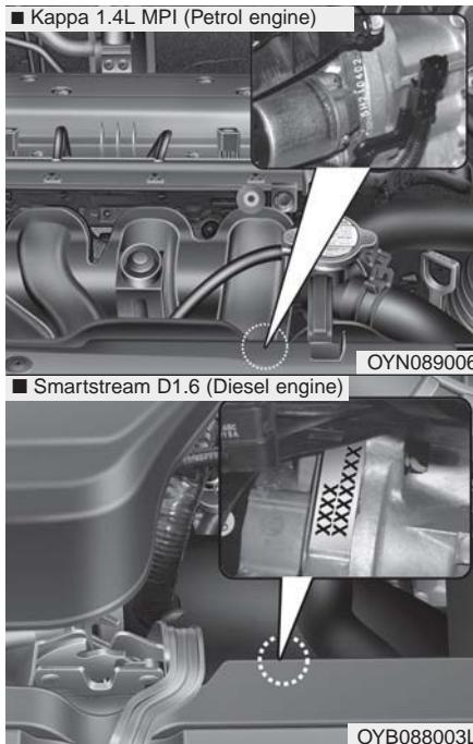
The engine number is stamped on the engine block as shown in the drawing.
