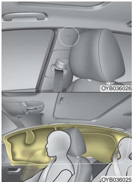
Curtain air bags are located along both sides of the roof rails above the centre pillar.
