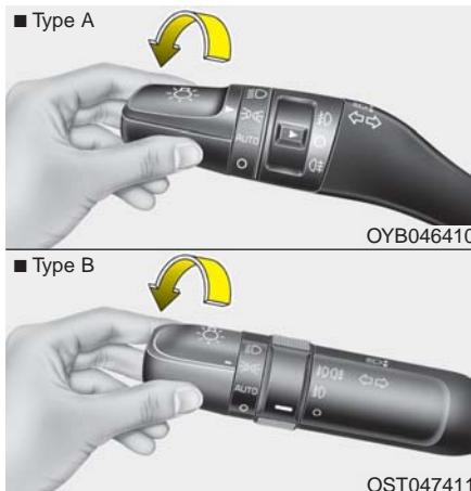
When the light switch is in the parking light position (2nd position), the tail position, license and instrument panel lights will turn ON.
