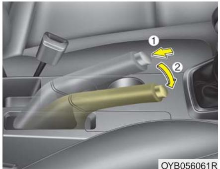
To release the parking brake, first apply the foot brake and pull up the parking brake lever slightly. Secondly depress the release button (1) and lower the parking brake lever (2) whilst holding the button.
