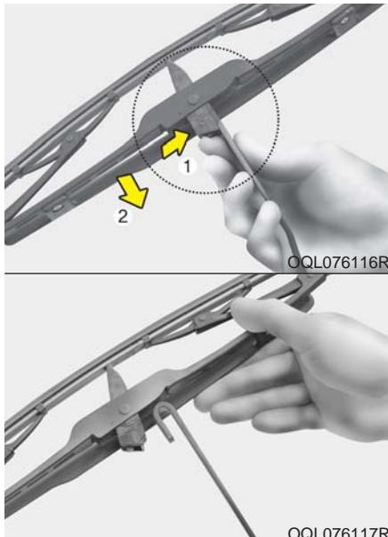
2. Compress the clip and slide the blade assembly downward.
