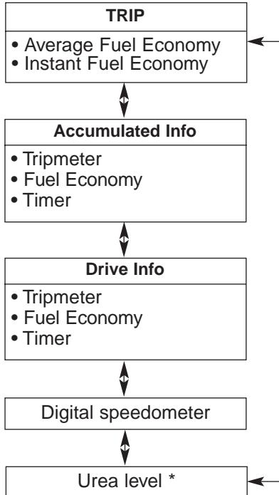
To change the trip mode, scroll the MOVE scroll switch ( $\wedge/\vee$ ) in the trip computer mode.
