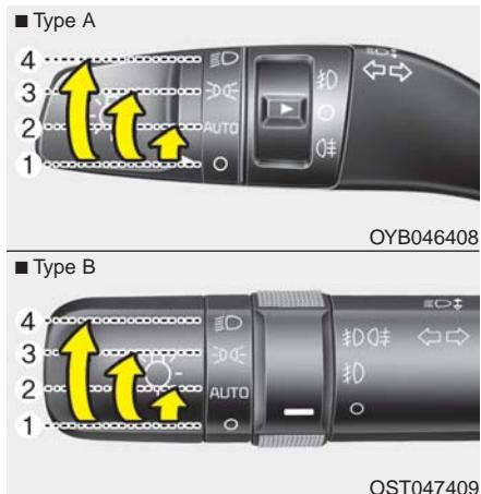
The light switch has a Headlight and a Parking light position.
