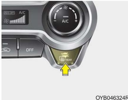
The defroster heats the window to remove frost, fog and thin ice from the rear window, whilst the engine is running.
