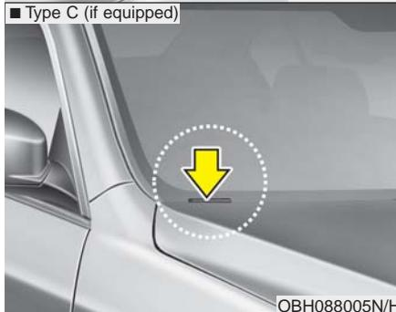
The VIN is also on a plate attached to the top of the dashboard.
