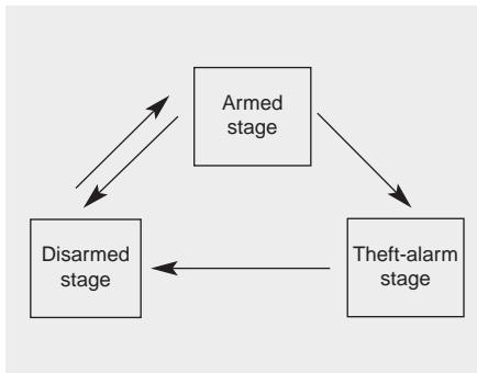
This system is designed to provide protection from unauthorised entry into the car. This system is operated in three stages: the first is the "Armed" stage, the second is the "Theft-alarm" stage, and the third is the "Disarmed" stage. If triggered, the system provides an audible alarm with blinking of the hazard warning lights.
