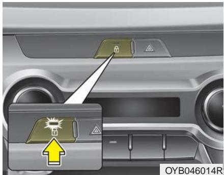
It is operated by pressing the door lock/unlock switch.
