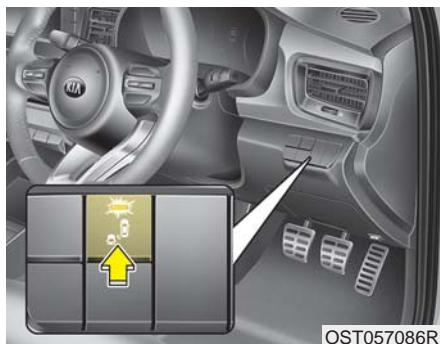
The indicator on the switch will illuminate when the Blind-Spot Collision Warning (BCW) system switch is pressed with the ignition switch ON. If the vehicle speed exceeds 30 km/h (18.6 mph), the system will activate.
