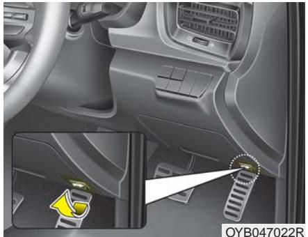
1. Pull the release lever to unlatch the bonnet. The bonnet should pop open slightly.
