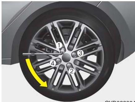
6. Loosen the wheel lug nuts counterclockwise one turn each, but do not remove any nut until the tyre has been raised off the ground.
