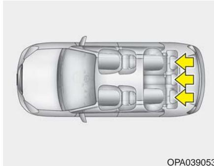
The rear seat is equipped with headrests for the occupant's safety and comfort.
