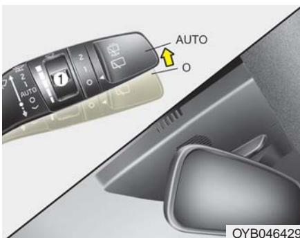
The rain sensor located on the upper end of the windscreen glass senses the amount of rainfall and controls the wiping cycle for the proper interval. The more it rains, the faster the wiper operates. When the rain stops, the wiper stops.
