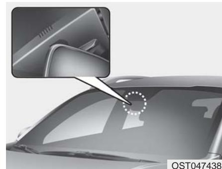
Auto defogging reduces the possibility of fogging up the inside of the windscreens by automatically sensing the moisture of inside the windscreen and air flow toward the windscreen can increase.
