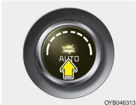
1. Push the AUTO button. The modes, fan speeds, air intake and air-conditioning will be controlled automatically according to the temperature setting.
