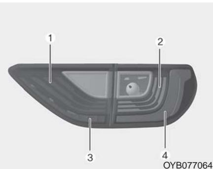
If the stop and tail lamp (LED) (1,2,3,4) does not operate, have your vehicle checked by a professional workshop.
