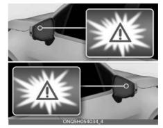
The warning light on the cluster, outside rearview mirror (side-view mirror) and head-up display (if equipped) will appear when the vehicle on both lanes is detected from the rear.
