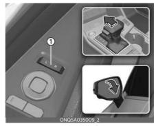
The position of the outside rearview mirror switch (1) determines whether the mirrors will move:
