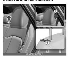
To remove the headrest, raise it as far as it can go then press the release button (1) while pulling the headrest up (2).
