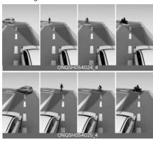
Forward Collision-Avoidance Assist may not detect other vehicles, powered two-wheelers, pedestrians or cyclists in front of you when driving on curved roads. This may result in no warning, braking assist or steering assist when necessary.
