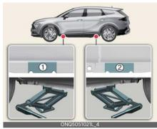
9. Insert the jack handle into the jack and turn it clockwise, raising the vehicle until the tire just clears the ground. This measurement is approximately 1.2 inches (30 mm). Before removing the wheel lug nuts, make sure the vehicle is stable and that there is no chance for movement or slippage.
