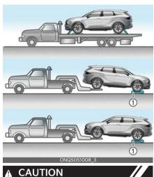
The AWD vehicle should never be towed with the wheels on the ground. This can cause serious damage to the transmission or the AWD system.
