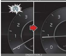
If the engine restarts automatically by the Early Engine Restart function, a message will appear on the LCD display (if equipped) when the "AUTO STOP" page on the instrument cluster is selected.
