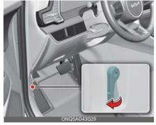
2. Go to the front of the vehicle, raise the hood slightly, push the secondary hood release lever (1) to the left and lift the hood (2).
