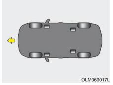
Tie-down hook (for flatbed towing, if equipped)
