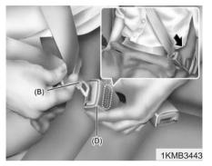
Pull the webbing and insert the tongue plate (B) into the open end of the buckle (D) until an audible "click" is heard, indicating the latch is locked. Make sure the belt is not twisted.
