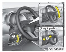
To change the steering wheel angle, pull down the lock-release lever (1), adjust the steering wheel to the desired angle (2) and height (3, if equipped) then pull up the lock-release lever to lock the steering wheel in place. Be sure to adjust the steering wheel to the desired position before driving.
