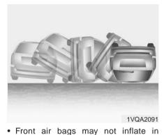
rollover accidents because front air bag deployment would not provide additional occupant protection.
