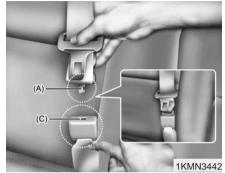
Insert the tongue plate (A) into the open end of the buckle (C) until an audible "click" is heard, indicating the latch is locked. Make sure the belt is not twisted.
