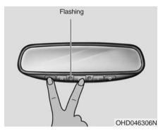
1. When programming the buttons for the first time, press and hold the left and center buttons ( ①, ①) simultaneously until the indicator light begins to flash after approximately 20 seconds. (This procedure erases the factory-set default codes. Do not perform this step to program additional hand-held transmitters.)
