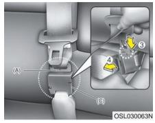
2. To retract the rear center seatbelt, insert the tongue plate or similar small rigid device into the web release hole (C). Pull up on the seat belt web (A) and allow the webbing to retract automatically.
