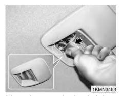
3. Insert the tongue plate into the hole on the belt assembly cover.
