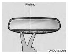
1. When programming the buttons for the first time, press and hold the left and center buttons ( ①, ①) simultaneously until the indicator light begins to flash after approximately 20 seconds. (This procedure erases the factory-set default codes. Do not perform this step to program additional hand-held transmitters.)
