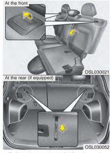
4. Pull on the seatback folding lever, then fold the seat toward the front of the vehicle.
