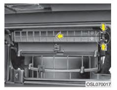
Remove the climate control air filter case while pressing the lock on the right of the cover.
