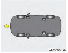
Tie-down hook (for flatbed towing, if equipped)
