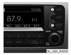
Press 1 ~ 6 button more than 0.8 seconds or longer to save the current station to the respective button with a beep.
