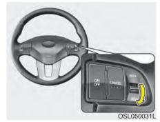
Push the - SET switch, and release it at the desired speed. The SET indicator light in the instrument cluster will illuminate. Release the accelerator at the same time. The desired speed will automatically be maintained.
