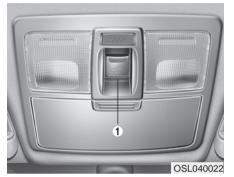
If your vehicle is equipped with a sunroof, you can slide or tilt your sunroof with the sunroof control lever located on the overhead console (1).
