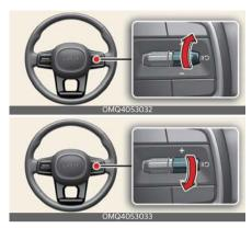
The set speed limit will be displayed on the instrument cluster.
