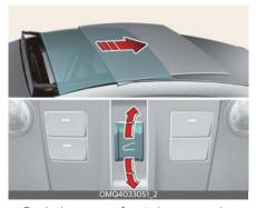
Push the sunroof switch rearward to the first detent position, the sunroof glass opens. If the power sunshade is closed, the power sunshade will open first.
