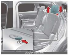
To raise the headrest, pull it up to the desired position (1). To lower the headrest, push and hold the release button (3) on the headrest support and lower the headrest to the desired position (2).
