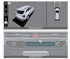
3D view function shows the vehicle in various angles. Press the 3D view icon on the Surround View Monitor screen to choose the angle. Press the 3D view icon again to reset the angle.
