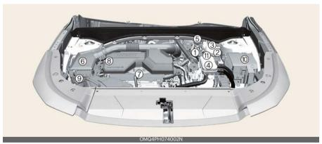
\* The actual engine room in the vehicle may differ from the illustration. 1. Electric Control Unit (ECU) 9-5 2. Engine coolant reservoir 9-17 3. Engine coolant reservoir cap 9-17 4. Inverter coolant reservoir 9-18 5. Brake fluid reservoir 9-21 9-24 6. Air cleaner 7. Engine oil dipstick 9-15 8. Engine oil filler cap 9-15 9. Windshield washer fluid reservoir 9-22 10.Fuse box 9-44
