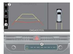
The rear-view function of the Surround View Monitor displays the vehicle's rear situation on the navigation system according to the driver's settings, assisting in safe parking.
