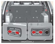
You can adjust the direction of air delivered from these vents using the vent control levers as shown.
