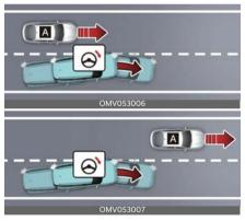
[A]: Approaching car from side Lane-Change Side function can help mitigate or avoid a collision with vehicles or powered two-wheelers in the next lane when changing lanes by assisting the driver's steering.
