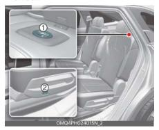
The 2nd row seat can be unlocked by pulling the strap located beneath the 2nd row seat seatback. If the strap is located beneath the 2nd row seatback, there is a label attached to show where the strap is located in.
