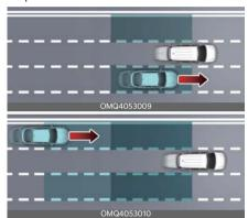
Blind-Spot Collision-Avoidance Assist can help detect and informs the driver that a vehicle is approaching at high speed from the blind spot area.
