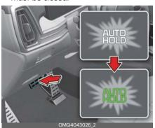
When coming to a complete stop by pressing the brake pedal, the AUTO HOLD indicator changes from white to
