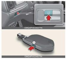
1 Power liftgate open/close button and Press the power tailgate open/close button for 1 second. The tailgate opens or closes with a warning sound.
