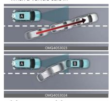
[A]: Your vehicle, [B]: Front vehicle If a vehicle cuts in front of you, Leading Departure Alert may not operate properly.
