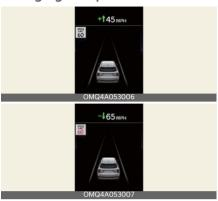
If the speed limit of the road changes during the operation of Manual Speed Limit Assist or Smart Cruise Control, an arrow in the direction of up or down is displayed to inform the driver that the set speed needs to be changed. The driver can change the set speed according to the speed limit by using the (+) or (-) switch on the steering wheel.
