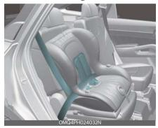
All passenger seat belts move freely under normal conditions and only lock under extreme or emergency conditions (emergency locking mode). So, in order to secure a child restraint, you must manually pull the seat belt all the way
