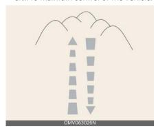
When you are driving up or down hills drive as straight as possible. Use extreme caution in driving up or down steep hills. You may flip over your vehicle depending on the grade, terrain and water/mud conditions.
