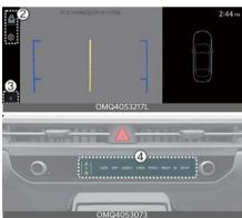
The rear top view shows an image of the vehicle looking down from above, allowing you to determine the distance from the rear vehicle or object when parking. Press the Rear Top View button to turn on the Rear Top View.
