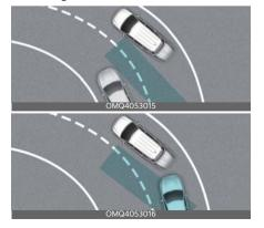
Blind-Spot Collision-Avoidance Assist may not operate properly on a curved road. Blind-Spot Collision-Avoidance Assist may not detect the vehicle in the next lane.
