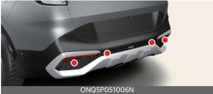
Rear ultrasonic sensors
