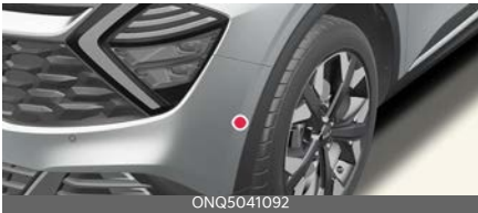
Rear side ultrasonic sensors
