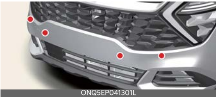
Front ultrasonic sensors
