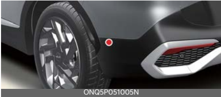
Rear ultrasonic sensors
