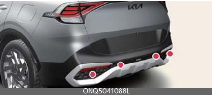
Rear ultrasonic sensors
