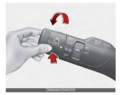
The parking lamp and headlamp will be turned ON or OFF automatically depending on the amount of daylight as measured by the ambient light sensor on the center dashboard.
