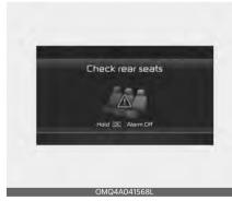
If you do not want to use the Rear Occupant Alert (ROA) system, press OK button on the steering wheel when the 1st alert is displayed on the cluster. Doing so will deactivate the 2nd alert once.
