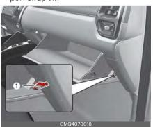
Remove the climate control air filter cover by pulling out both sides of the cover.
