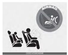
Never place a rear-facing child restraint in the front passenger's seat.
