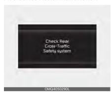
When Rear Cross-Traffic Collision-Avoidance Assist is not working properly, the 'Check Rear Cross-Traffic Safety system' warning message will appear on the cluster, and the function will turn off automatically or the function will be limited. Have the function inspected by an authorized Kia dealer.
