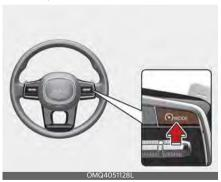
2. Press the Driving Assist ( ) MODE) button at the desired speed. The set speed and Cruise ( ) CRUISE) indicator will appear on the cluster.
