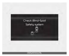
When Safe Exit Assist is not working properly, the 'Check Blind-Spot Safety
