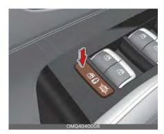
To cancel the electronic child safety lock, push the electronic child safety lock switch one more time and then the indicator turns off.
