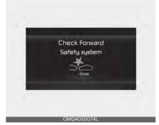
When Forward Collision-Avoidance Assist is not working properly, the 'Check Forward Safety system' warning message will appear, and the (/i) and
