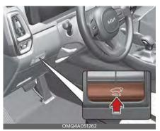
While the liftgate is opening or closing, press the button to stop liftgate operation.
