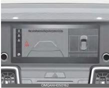
To warn the driver of an approaching vehicle from the rear left/right side of your vehicle, the warning light on the side view mirror will blink and a warning will appear on the cluster. At the same time, an audible warning will sound and the steering wheel will vibrate. If the Rear View Monitor is operating, a warning will also appear on the infotainment system screen.
