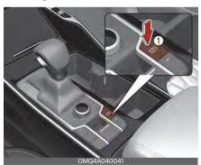
Press the Parking/View button (1) to turn Rear View Monitor on or off.
