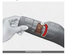
The fog lights will turn on when the fog light switch (1) is turned to the on position after the headlamp is turned on. To turn off the fog lights:
