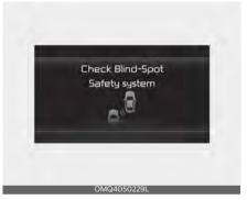
When Blind-Spot Collision-Avoidance Assist is not working properly, the 'Check Blind-Spot Safety system' warning message will appear on the cluster, and the function will turn off automatically or the function will be limited. Have the function inspected by an authorized Kia dealer.
