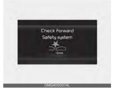
When Forward Collision-Avoidance Assist is not working properly, the 'Check Forward Safety system' warning message will appear, and the( 1)
