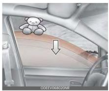
If the upward movement of the window is blocked by an object or part of the body, the window will detect the resistance and will stop upward movement. The window will then lower approximately 30 cm (11.8 inches) to allow the object to be cleared.
