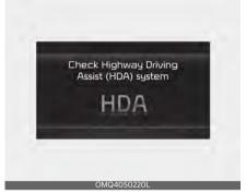
When Highway Driving Assist is not working properly, the 'Check Highway Driving Assist (HDA) system' warning message will appear, and the ( ) warning light will appear on the cluster. Have the function inspected by an authorized Kia dealer.
