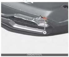
Remove the socket (A) from the assembly by turning the socket counterclockwise until the tabs on the socket align with the slots on the assembly.
