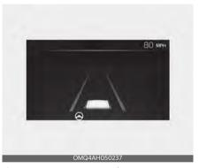
If the vehicle ahead and/or both lane markings are detected and your vehicle speed is above 60 km/h (40 mph) and below 200 km/h (120 mph), the green (A) indicator light will appear on the
