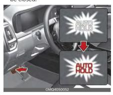
When coming to a complete stop by pressing the brake pedal, the AUTO HOLD indicator changes from white to green indicating the AUTO HOLD is engaged. The vehicle will remain at a standstill even if you release the brake pedal.
