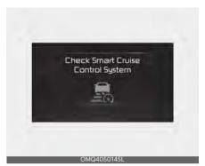
When Smart Cruise Control is not working properly, the 'Check Smart Cruise Control system' warning message will appear, and the ( ) warning light will appear on the cluster. Have the function inspected by an authorized Kia dealer.
