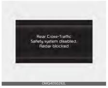
When the rear bumper around the rear corner radar or rear sensor is covered with foreign material, such as snow or rain, or installing a trailer or carrier, it can reduce the detecting performance and temporarily limit or disable Rear Cross-Traffic Collision-Avoidance Assist.
