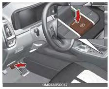
Releasing the parking brake with EPB switch.
