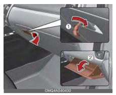
The glove box can be locked and unlocked with the mechanical key (1).
