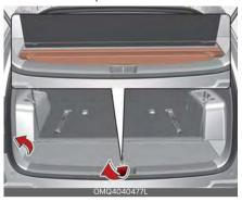
3. While pushing the guide pin, pull out the cargo security screen.
