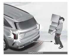
If you are positioned in the detecting area ( $50 \sim 100 \text{ cm} [20 \sim 40 \text{ inches}]$  behind the vehicle) carrying a smart key, the hazard warning lights will blink and chime will sound to alert you the smart key has been detected and the liftgate will open.
