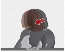
The headrest may be adjusted forward to 3 different positions by pulling the headrest forward to the desired position. To adjust the headrest to it's furthest backwards position, pull it fully forward to the farthest position and release it. Adjust the headrest so that it properly supports the head and neck.
