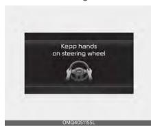
If the driver takes their hands off the steering wheel for several seconds, the 'Keep hands on the steering wheel' warning message will appear and an audible warning will sound in stages. First stage: Warning message Second stage: Warning message (red steering wheel) and audible warning
