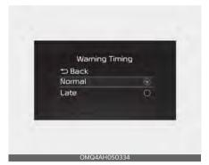
With the ENGINE START/STOP button in the ON position, select 'Driver Assistance → Warning Timing' from the Settings menu to change the initial warning activation time for Forward Collision-Avoidance Assist.
