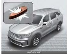
When all the doors (and liftgate) are closed and locked, the door handle lamp will come on for about 15 seconds if any of the below is performed.
