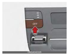
Press the OFF button to turn off the air climate control system.
