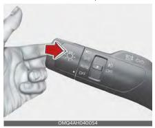
It will return to the normal (low beam) position when released. The head-lamp switch does not need to be on to use this flashing feature.
