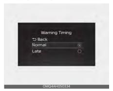
With the ENGINE START/STOP button in the ON position, select 'Driver Assistance → Warning Timing' from the Settings menu to change the initial warning activation time for Forward Collision-Avoidance Assist.
