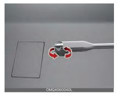
4. Use the wheel lug nut wrench to loosen the bolt enough to lower the spare tire.
