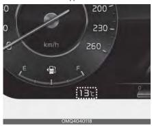
This gauge indicates the current outside air temperatures by 1 °C (1 °F).
