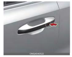
Carrying the smart key, you may lock and unlock the vehicle doors (and liftgate). Also, you may start the engine. Refer to the following for more details.
