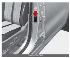
The vehicle certification label attached on the driver's side center pillar gives the vehicle identification number (VIN).
