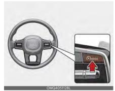
Press the Driving Assist ( MODE) button to turn Smart Cruise Control off.
