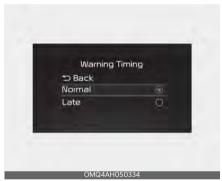
With the ENGINE START/STOP button in the ON position, select 'Driver Assistance → Warning Timing' from the Settings menu to change the initial warning activation time for Blind-Spot Collision-Avoidance Assist.
