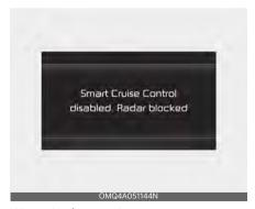
When the front radar cover or sensor is covered with snow, rain, or foreign
