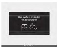
When Highway Driving Assist is operating, your vehicle will stop if the vehicle ahead of you stops. Also, if the vehicle ahead of you starts moving approximately within 30 seconds after the stop, your vehicle will start as well. In addition, after the vehicle has stopped and approximately 30 seconds have passed, the 'Use switch or pedal to accelerate' message will appear on the cluster. Depress the accelerator pedal or push the + switch, - switch or () switch to start driving.
