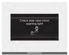
When the side view mirror warning light is not working properly, the `Check side view mirror warning light' warning message will appear on the cluster for several seconds, and the master ( ) warning light will appear on the cluster. If the master warning light appears, have the vehicle inspected by an authorized Kia dealer.
