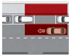
After the vehicle stops, when an approaching vehicle from the rear area is detected as soon as a passenger opens a door, Safe Exit Warning will warn the driver with a warning message and an audible warning to help prevent a collision.
