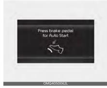
If you shift the gear from N to D (Manual mode) or R without depressing the brake pedal after stopping engine automatically, the engine does not restart automatically and a warning chime alarms. When this happens, press the brake pedal for auto start.
