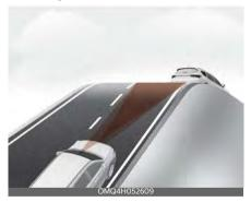
During uphill or downhill driving, the Smart Cruise Control may not detect a moving vehicle in your lane, and cause your vehicle to accelerate to the set speed. Also, vehicle speed will rapidly decrease when the vehicle ahead is detected suddenly.
