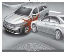
In an angled collision, the force of impact may direct the occupants in a direction where the air bags would not be able to provide any additional benefit, and thus the sensors may not deploy any air bags.
