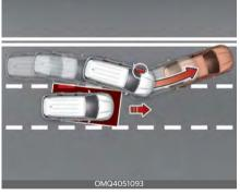
When changing lanes by detecting the lane ahead, if the function judges that there is a collision risk with an approaching vehicle in the blind spot, the function will help avoid collision by applying the differential brake.
