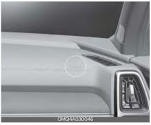
The indication of the function's presence are the letters "AIR BAG" located on the air bag pad cover on the steering wheel and on the cover of the driver's side knee bolster located below the steering wheel and the passenger's side front panel pad above the glove box.
