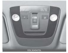
The sunroof can only be operated when the ignition switch or ENGINE START/ STOP button is in the ON or START position.
