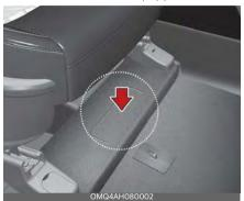
The number is punched on the floor under the front right side seat. To check the number, open the cover.
