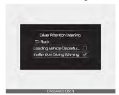
With the ENGINE START/STOP button in the ON position, select or deselect 'Driver Assistance → Driver Attention Warning' from the Settings menu to set whether or not to use each function.
