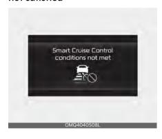
If the Driving Assist ( MODE) button, + switch, - switch or ( ) switch is operated when the function's operating conditions are not satisfied, the 'Smart Cruise Control conditions not met' will appear on the cluster, and an audible warning will sound.
