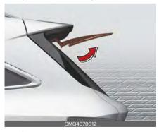
3. Lift up the wiper blade, and pull the blade to remove it.
