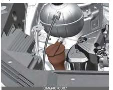
Check the fluid level in the washer fluid reservoir and add fluid if necessary. Plain water may be used if washer fluid is not available.
