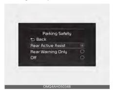
With the ENGINE START/STOP button in the ON position, select or deselect 'Driver Assistance → Parking Safety' from the Settings menu to set whether or not to use each function.
