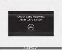
When Lane Following Assist is not working properly, the 'Check Lane Following Assist (LFA) system' warning message will appear on the cluster. If this occurs, have the function inspected by an authorized Kia dealer.
