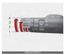
To operate the lights, turn the knob at the end of the control lever to one of the following positions:
