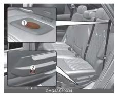
Or, the 2nd row seat can be unlocked by pulling the strap located beneath the 2nd row seat seatback. If the strap is located beneath the 2nd row seatback, there is a label attached to show where the strap is located in.
