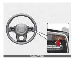
Press the Driving Assist ( MODE) button to turn Manual Speed Limit Assist off. The Speed Limit indicator ( LIMIT) will go off.
