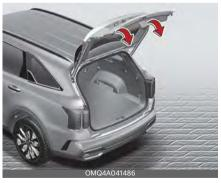
To close the liftgate, lower and push down the liftgate firmly. Make sure that the liftgate is securely latched. Features of your vehicle Liftgate
