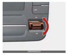
The temperature will increase to the maximum (HI) by moving the switch upwards.
