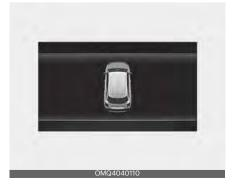
The warning chime will operate when the vehicle is being driven at or above 3 km/h (2 mph) with the hood open.
