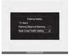
With the ENGINE START/STOP button in the ON position, select 'Driver Assistance → Parking Safety → Rear Cross-Traffic
