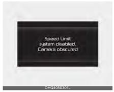
When the front windshield where the front view camera is located is covered with foreign material, such as snow or rain, it can reduce the detecting performance and temporarily limit or disable Intelligent Speed Limit Assist.
