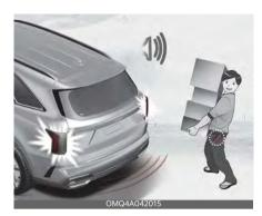
The hazard warning lights will blink and chime 6 times and then the lift-gate will open.
