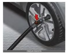
Unscrew the valve cap from the valve of the defective tire and screw the filling hose of the sealant bottle onto the tire valve.
