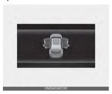
This warning is displayed indicating which door, the hood, the liftgate or the sunroof is open.
