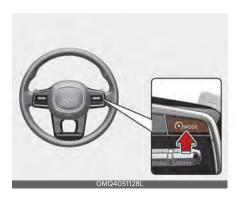
Press the Driving Assist ( MODE) button to turn Cruise Control off. The Cruise ( CRIUSE) indicator will go off.
