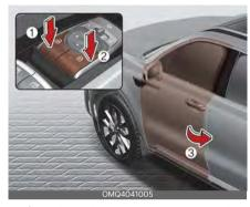
If you lock the door with the central door lock button (2), all vehicle doors will lock automatically.
