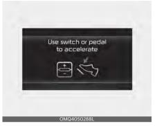
In traffic, your vehicle will stop if the vehicle ahead of you stops. Also, if the vehicle ahead of you starts moving, your vehicle will start as well.
