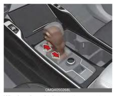
Whether the vehicle is stationary or in motion, manual mode is selected by pushing the shift lever from the D (Drive) position into the manual gate. To return to D (Drive) range operation, push the shift lever back into the main gate. In manual mode, moving the shift lever backwards and forwards will allow you to make gearshifts rapidly. In contrast to a manual transmission, manual mode allows gearshifts with the accelerator pedal depressed.
