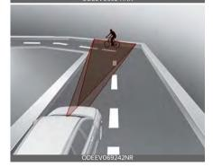
Forward Collision-Avoidance Assist may detect a vehicle, pedestrian, or cyclist in the next lane or outside the lane when driving on a curved road. If this occurs, the function may unnecessarily warn the driver and control the brake. Always check the traffic conditions around the vehicle.
