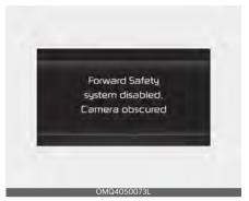
When the front windshield where the front view camera is located, is covered with foreign material, such as snow or rain, it can reduce the detecting performance and temporarily limit or disable Forward Collision-Avoidance Assist.
