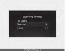
With the ENGINE START/STOP button in the ON position, select 'Driver Assistance → Warning Timing' from the Settings menu to change the initial warning activation time for Driver Attention Warning. When the vehicle is first delivered, Warning Timing is set to 'Normal'. If you change the Warning Timing, the warning time of other Driver Assistance systems may change.
