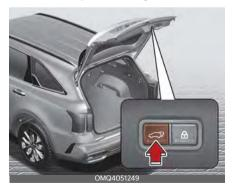
Press the power liftgate open/close button. The liftgate opens or closes with a warning sound.
