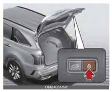
Press the power liftgate lock button while carrying the smart key. The liftgate closes and locks with a warning sound. Additionally, all doors will lock.
