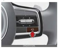
Press the (| ) button to temporarily pause the set speed limit. The set speed limit will turn off but the Speed Limit indicator ( TIMIT) will stay on.
