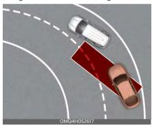
Blind-Spot Collision-Avoidance Assist may not operate properly when driving on a curved road. The function may recognize a vehicle in the same lane.
