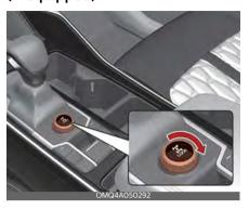
You can switch from DRIVE MODE to SNOW mode by turning the knob. If you turn the DRIVE/SNOW mode button again, the vehicle will go back to DRIVE MODE.
