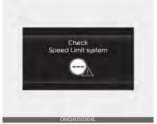
When Intelligent Speed Limit Assist is not working properly, the warning message will appear on the cluster for several seconds. If this occurs, have the function checked by an authorized Kia dealer.
