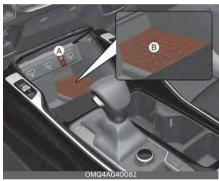
[A]: Indicator, [B]: Charging pad Firmly close all doors, and make sure to turn ON the ignition switch or press the ENGINE START/STOP button. To start wireless charging, place the smart phone equipped with wireless charging function on the wireless charging pad. For best wireless charging results, place the smart phone on the center of the charging pad.
