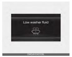
This warning message is displayed if the washer fluid level in the reservoir is nearly empty.
