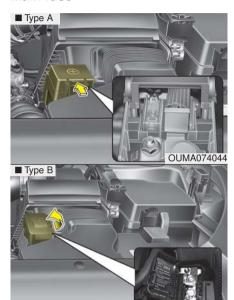
If the main fuse is blown, it must be removed as follows:
