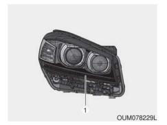
If the position lamp (LED) (1) does not operate, have the vehicle checked by an authorized Kia dealer. The LED lamps cannot be replaced as a single unit because it is an integrated unit. The LED lamps has to be replaced with the unit.
