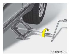
Insert the wheel lug nut wrench into the jack and turn it clockwise, raising the vehicle until the tire just clears the ground. This measurement is approximately 1 in. (30 mm).
