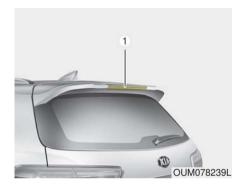
If the high mounted stop lamp (LED) (1) does not operate, have the vehicle checked by an authorized Kia dealer.
