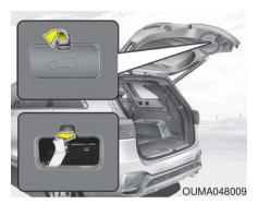
Your vehicle is equipped with an emergency liftgate safety release lever located on the bottom of the liftgate. When someone is inadvertently locked in the cargo area, the liftgate can be opened by pushing the release lever and pushing open the liftgate.
