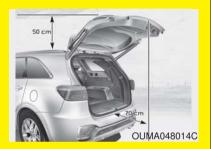
Make sure that there are no people or objects in the path of the power liftgate (or smart power liftgate) prior to use. Serious injury, damage to the vehicle or damage to surrounding objects may result if contact with the power liftgate (or smart power liftgate) occurs.
