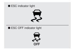
When ignition switch is turned to ON, the indicator light illuminates, then goes off if the ESC system is operating normally.
