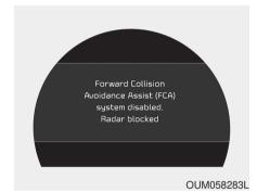
When the sensor cover or the sensor lens is smudged with the foreign substances, such as snow or rain, the FCA operation may temporarily stop. In this case, the warning message
