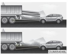
Always be cautious for vehicles that are taller with higher clearance, or vehicles carrying loads that stick out of the back of the vehicle.
