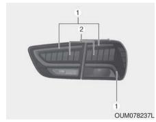
If the stop and tail lamp (LED) (1,2), does not operate, have the vehicle checked by an authorized Kia dealer.
