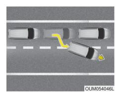
When vehicles are at a standstill and the vehicle in front of you changes to the next lane, be careful when your vehicle starts to move because it may not recognize the stopped vehicle in front of you.
