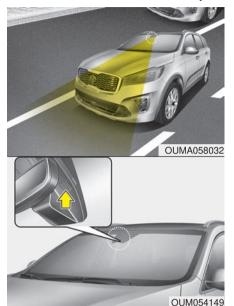
The Lane Keeping Assist System detects the lane markers on the road with a front view camera at the front windshield, and assists the driver's steering to help keep the vehicle in the lanes.
