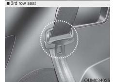
The rear seat belt buckles can be stowed in the pocket between the rear seatback and cushion when not in use.
