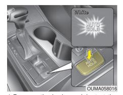
1.Depress the brake pedal, start the engine and then press the Auto Hold button. The white AUTO HOLD indicator will come on indicating the system is in standby. Before the Auto Hold will engage, the driver's door, engine hood and trunk must be closed and the driver's seat belt must be fastened.
