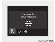
This warning message and light is to warn the driver the road may be icy. When the following conditions occur, the warning message displays for 4 seconds and light(including Outside Temperature Gauge) blinks 5 times and then illuminates.
