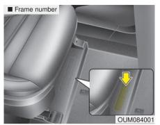
The vehicle identification number (VIN) is the number used in registering your vehicle and in all legal matters pertaining to its ownership, etc. The number is punched on the floor under the front passenger seat.
