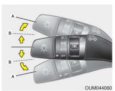
The ignition switch must be on for the turn signals to function. To turn on the turn signals, move the lever up or down (A). The green arrow indicators on the instrument panel indicate which turn signal is operating. They will self-cancel after a turn is completed. If the indicator continues to flash after a turn, manually return the lever to the OFF position.
