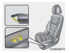
Press the front portion of the switch to raise the cushion extension, or the rear portion of the switch to lower it. Release the switch once the cushion extension reaches the desired position.
