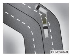
Your vehicle speed can be reduced due to a vehicle in the adjacent lane. Adjust your vehicle speed by depressing the brake pedal according to the road condition ahead and driving condition. Apply the accelerator pedal and select the appropriate set speed. Check to be sure that the road conditions permit safe operation of the smart cruise control system.
