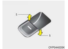
The driver's door has a master power window switch that controls all the windows in the vehicle.
