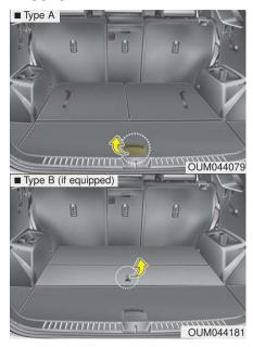
You can place a first aid kit, a reflector triangle, tools, etc. in the box for easy access.
