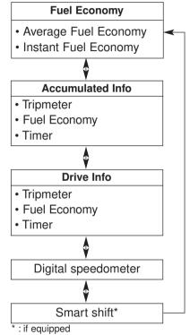
To change the trip mode, scroll the MOVE scroll switch  $(\triangle/\nabla)$  in the trip computer mode.
