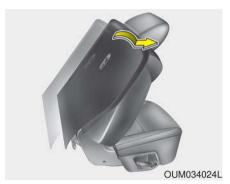
3. Fold the 2nd row seatback and push the seat to the farthest forward position.
