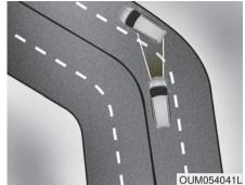
The FCA system may recognize a vehicle in the next lane when driving on a curved road.
