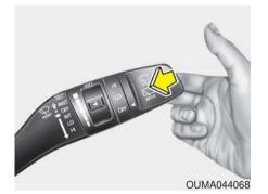
In the OFF position, pull the lever gently toward you to spray washer fluid on the windshield and to run the wipers 1-3 cycles.
