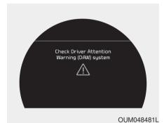
When the "Check System" warning message appears, the system is not working properly. In this case, have the vehicle inspected by an authorized Kia dealer.
