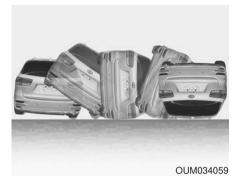
Front air bags may not inflate in all rollover accidents where the SRSCM indicates that the front air bag deployment would not provide additional occupant protection.
