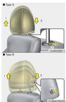
To raise the headrest, pull it up to the desired position (1). To lower the headrest, push and hold the release button (2) on the headrest support and lower the headrest to the desired position (3).
