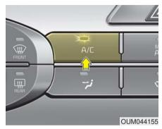
Press the A/C button to turn the air conditioning system on (indicator light will illuminate). Press the button again to turn the air conditioning system off.
