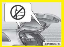
Do not grab the power liftgate struts while the liftgate is open.
