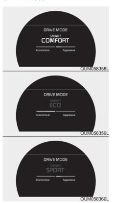
SMART mode selects the **SMART** proper driving mode among ECO, COMFORT and SPORT by judging the driver's driving habits (i.e. mild or dynamic) from the brake pedal depression or the steering wheel operation.
