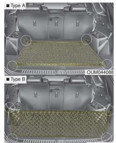
To keep items from shifting in the cargo area, you can use the holders located in the cargo area to attach the luggage net.
