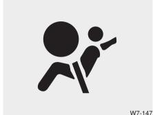
If the air bag warning light is illuminated for more than 6 seconds after the ignition is turned on, or of it illuminates during vehicle operation, an SRS component may not be functioning properly and you should have your vehicle checked by an authorized Kia dealer.
