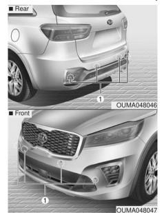
The parking assist system assists the driver during movement of the vehicle by chiming if any object is sensed within the distance of 100 cm (39 in.) in front and 120 cm (47 in.) behind the vehicle
