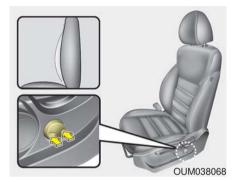
The lumbar support can be adjusted by pressing the lumbar support switch on the side of the seat.
