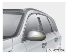
If the side repeater lamp (LED) (1), does not operate, have the vehicle checked by an authorized Kia dealer. The LED lamps cannot be replaced as a single unit because it is an integrated unit. The LED lamps has to be replaced with the unit.
