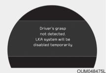
If the driver takes hands off the steering wheel for several seconds while the LKA is activated, the system will warn the driver.
