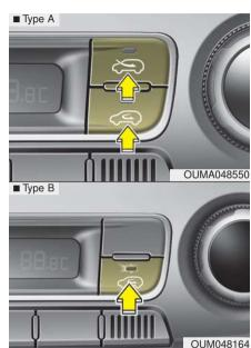
This is used to select the outside (fresh) air position or recirculated air position.
