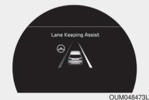
If the vehicle leaves a lane, the lane marker you cross will blink on the LCD display.
