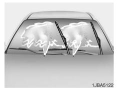
Commercial hot waxes applied by automatic vehicle washes have been known to make the windshield difficult to clean.
