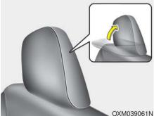
The headrest will fold down automatically when folding the seatback.
