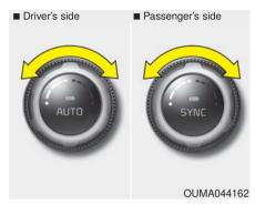
The temperature will increase to the maximum (HI) by turning the knob to the extreme right.
