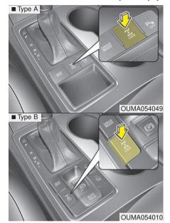
Engine power can be delivered to all front and rear wheels for maximum traction. AWD is useful when extra traction is required, such as, when driving on slippery, muddy, wet, or snow-covered roads
