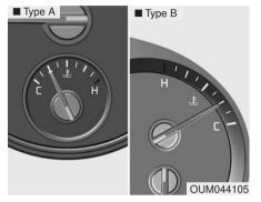
This gauge indicates the temperature of the engine coolant when the ignition switch or Engine Start/Stop button is ON.
