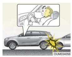
Air bags are not designed to inflate in rear collisions, because occupants are moved backward by the force of the impact. In this case, inflated air bags would not be able to provide any additional benefit.
