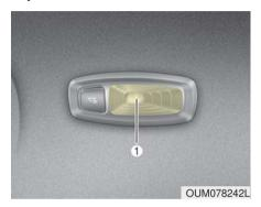
If the personal lamp (LED) (1), does not operate, have the vehicle checked by an authorized Kia dealer. The LED lamps cannot be replaced as a single unit because it is an integrated unit. The LED lamps has to be replaced with the unit.
