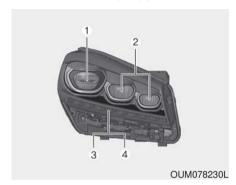
If the Low/High beam lamp(1,2), Front turn signal lamp(3), Day time running lamp/Position lamp(4) does not operate, have the vehicle checked by an authorized Kia dealer. The LED lamps cannot be replaced as a single unit because it is an integrated unit. The LED lamps has to be replaced with the unit.
