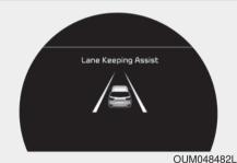
If the speed of the vehicle is over 64 km/h (40 mph) and the system detects lane markers, the color changes from gray to white. When the conditions below are met, LKA SYSTEM will be enable to assist steering.
