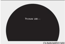
3.Move the lever down (to SET-), and release it at the desired speed. The set speed in the instrument cluster will display. Release the accelerator at the same time. The desired speed will automatically be maintained.
