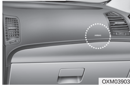
Passenger's front air bag
