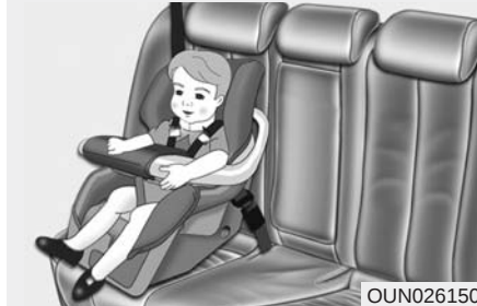
Forward-facing child restraint system
