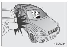
Front airbags may not inflate in side impact collision, because occupants move to the direction of the collision, and thus front airbag deployment does not provide proper protection.
