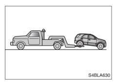
On 2WD vehicles, it is acceptable to tow the vehicle with the front wheels on the ground (without dollies) and the rear wheels off the ground.
