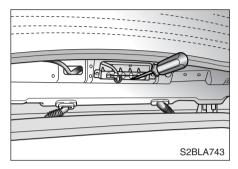
Separate the socket and the lens part by pulling the socket retaining tabs outward.
