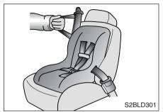
Pull the shoulder portion of the safety belt all the way out. When the shoulder portion of the safety belt is fully extended, it will shift the retractor to the "Auto Lock" (child restraint) mode.
