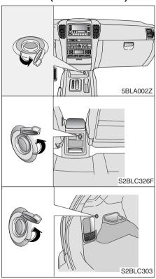
To plug in auxiliary electrical equipment, flip the outlet cover open from the edge of the cover and follow the proper installation instructions that are included with any electrical equipment you install. Maximum electrical draw must not exceed 10 ampere at 12 volts after engine is started.
