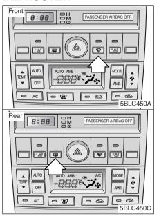
The defroster clears frost, fog and thin ice from the interior and exterior of the front windshield and rear window, while the engine is running.
