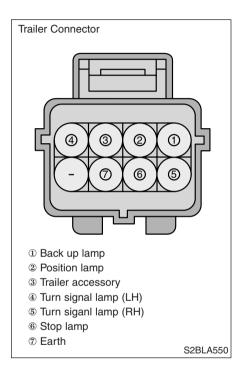
You must check the capacity of the lighting system and electrical equipment for a trailer before connecting the wires.
