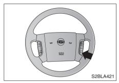
Depress the COAST/SET switch, located on the steering wheel, and release it at the speed you want. Release the accelerator at the same time. The desired speed will automatically be maintained and the CRUISE light on your instrument cluster will illuminate.
