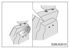
2. Remove the headrest and put the headrest poles into the holes on the rear of the seat cushion.
