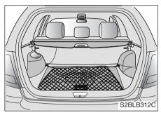
To keep items from shifting in the trunk, you can use the four rings located in the trunk to attach the cargo net.
