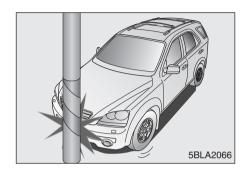
Airbags may not inflate if the vehicle collides with objects such as utility poles or trees, where the point of impact is concentrated to one area and the full force of the impact is not delivered to the sensors.
