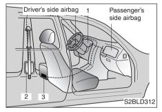
When the vehicle stops suddenly, or if the occupant tries to lean forward too quickly, the seat belt retractor will lock into position. However, in certain frontal collisions, the pre-tensioner will also activate and pull the seat belt into tighter contact against the occupant's body.
