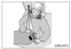
Insert the tongue plate into the open end of the buckle until an audible "click" is heard, indicating the belt is locked in the buckle.
