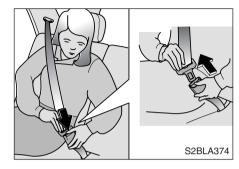
To unfasten the lap/shoulder belt: Press the release button on the buckle and allow the belt to slowly retract.
