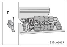
If the 120A "MAIN" fuse is blown, it must be removed as follows:
