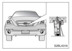
Go to the front of the vehicle, slightly raise the hood, push the secondary latch to the right and lift the hood.
