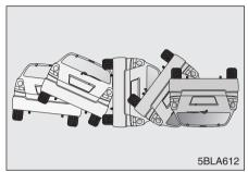
Airbags may not inflate in rollover accidents because airbag deployment would not provide proper protection to the occupants.
