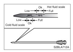
5. Pull out the dipstick again and check the fluid level.
