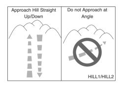
When you are driving up or down hills, drive as close to straight up and down the hills as possible. Use extreme caution in going up or down steep hills, since you can flip your vehicle over depending on the grade, terrain and water/mud conditions.
