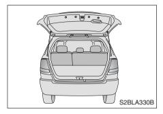
3. Pull the rear hatch back and up to open.
