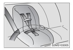
Placing a passenger safety belt Into the auto lock mode
