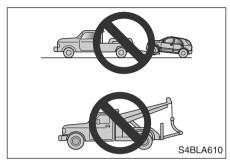
It is recommended that your vehicle be towed with a wheel lift or flatbed equipment. Do not tow with a slingbelt. Our company has not approved a slingbelt towing procedure.
