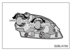
4. Remove the headlight bulb cover by turning it counterclockwise.
