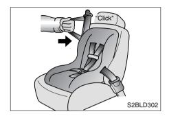
4. Slowly allow the belt to retract. Pull up on the shoulder webbing. A "clicking" or "ratcheting" sound will be heard as the belt retracts. This indicates the retractor is now in the automatic locking mode. Push down on the child restraint while you pull up on the belt in order to remove any slack in the belt.
