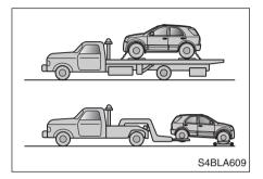
On 4WD Vehicles, it is recommended that your vehicle be towed with a wheel lift and dollies or flatbed equipment with all the wheels off the ground.
