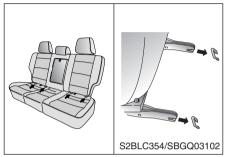
ISOFIX anchors have been provided in your vehicle. The ISOFIX anchors are located in the left and right outboard rear seating positions. Their locations are shown in the illustration. There is no ISOFIX anchor provided for the center rear seating position.
