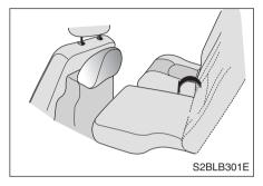
3. Press the lock release button on the seatbacks, then fold the seatback forward and down firmly.
