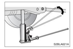
Securely tighten the valve of the jack. Move the jack handle up and down until the top of the jack contacts the proper point and takes on a slight load.
