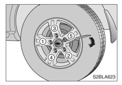
12. Once the wheel lug nuts have been tightened, lower the vehicle fully to the ground and continue to tighten the lug nuts until they are fully secured. Tighten the wheel lug nuts firmly in a "star" pattern. If you are unsure of the tightness of the wheel lug nuts, have them checked at the nearest service station. The specified tightening torque is 65-87 ft•lb (9~12 kg•m, 88-118 N•m).
