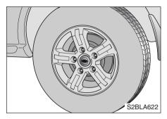
Mount the spare tire into position and install the wheel lug nuts with the beveled edge inward.
