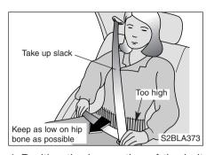
4. Position the lap portion of the belt across your lap as LOW ON THE HIPS as possible to reduce the risk of sliding under it during an accident. Adjust the belt to a SNUG FIT by pulling up on the shoulder portion of the safety belt. The belt retractor is designed to take up excess webbing automatically and to maintain tension on the belt. For maximum safety, do not put any excess slack into the safety belt.
