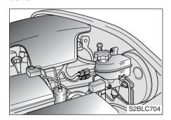
Check the fluid level in the reservoir periodically. The fluid level should be between MAX and MIN indicators on the side of the reservoir.
