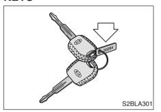
The key code number is stamped on the plate attached to your key set. Should you lose your keys, this number will enable an authorized Kia dealer to duplicate your keys easily. Remove this plate from the key ring and store it in a safe place. Also, record the code number and keep it in a safe and handy place, but not in the vehicle.
