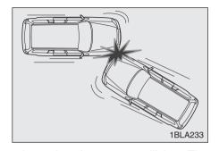
In a slant impact or collision, The force delivered will be relatively weaker than that of frontal or side collision. So, the airbags may not inflate.
