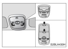
A compartment is provided at the overhead console to store sunglasses. To open the sunglass holder, press the cover and the holder will slowly open. Place your sunglasses in the compartment door with the lenses facing out.
