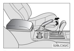
To release the parking brake, pull the handle up slightly and push the release button. Then lower the handle to the released position while holding the button in.
