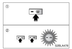
How to cancel forced air-conditioning operation and outside (fresh) air position in floor-defrost and defrost position;
