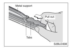
2. Firmly grasp the end of the rubber blade and pull until the tabs are free of the metal support.
