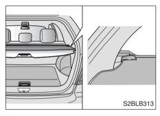
To use the tonneau cover, pull the handle backward and insert the edges into the slots of the slide rails.
