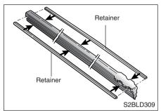
3. Remove the metal retainers from the rubber blade and install them in the new rubber blade.
