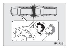
Airbags may not inflate in rear collisions, because occupants are moved backward by the force of the impact. In this case, the airbags do not provide proper protection.
