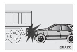
At the moment of an accident, drivers brake heavily with reflex. In such heavy braking, the front portion of the vehicle is lowered by the force of the braking and the vehicle can go under a vehicle with a higher ground clearance. Airbags may not inflate in this situation because impacts may not be delivered or may be delivered with less intensity.
