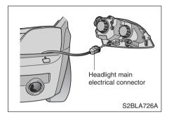
3. Disconnect the headlight main electrical connector.
