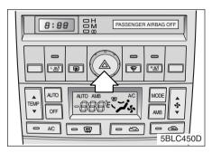
The hazard warning flasher causes the rear tail lights and front turn signal lights to flash on and off, which serves as a warning to other drivers to exercise caution when approaching or passing your vehicle.
