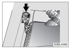
The auto fuel cutoff switch is located on the passenger's side of the engine compartment. In the event of a collision or sudden impact, the auto fuel cutoff device cuts off the fuel supply. If this device is activated, it must be reset by pressing in on the top of the switch before the engine can be restarted.
