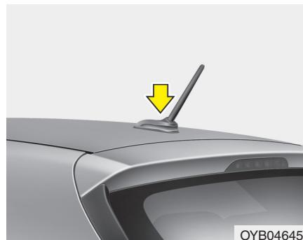
The micro pole antenna receives data transmitted from base stations and satellites (e.g. AM/FM, SXM, GPS, LTE) and also transmits to base stations (e.g. LTE). The antenna pole is removable type.
