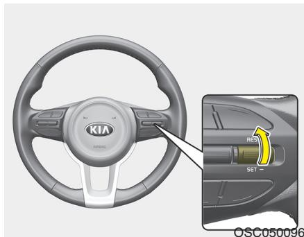
Release the switch when the desired speed is shown and the vehicle will accelerate to that speed.
