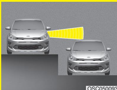
Blind-Spot Safety system may not operate properly when driving where the heights of the lanes are different. The function may not detect the vehicle on a road with different lane heights (underpass joining section, grade separated intersections, etc.).
