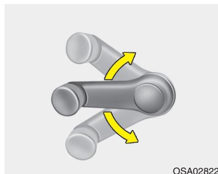
To raise or lower the window, turn the window regulator handle clockwise or counterclockwise.
