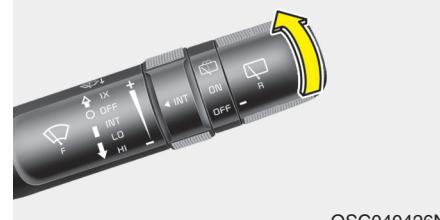
Push the lever away from you or turn the wiper lever switch upwards fully to spray rear washer fluid and to run the rear wipers 1~3 cycle. The spray and wiper operation will continue until you release the lever.
