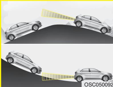
Blind-Spot Safety system may not operate properly when driving on a slope. The function may not detect the vehicle in the next lane or may incorrectly detect the ground or structure.
