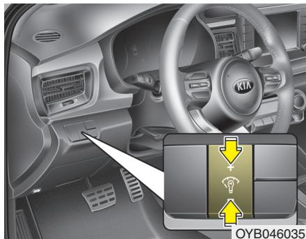
The instrument panel illumination intensity can be adjusted by pressing the control switch with the headlight switch in any position when the ignition switch or ENGINE START/STOP button is in the ON position.
