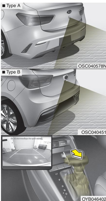
Rear View Monitor will show the area behind the vehicle to assist you when parking or backing up.
