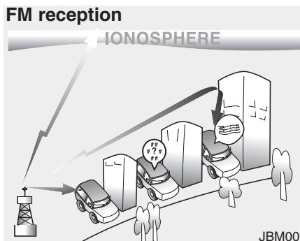
AM and FM radio signals are broadcast from transmitter towers located around your city. They are intercepted by the radio antenna on your vehicle. This signal is then received by the radio and sent to your vehicle speakers.
