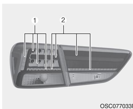
If the stop and tail lamp (LED) (1,2) does not operate, have the vehicle checked by an authorized Kia dealer. The LED lamps cannot be replaced as a single component because it is part of an integrated unit. The LED lamps have to be replaced with the unit.
