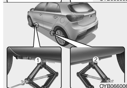
7. Place the jack at the front (1) or rear (2) jacking position closest to the tire you are changing. Place the jack at the designated locations under the frame. The jacking positions are plates welded to the frame with two tabs and a raised dot to index with the jack.
