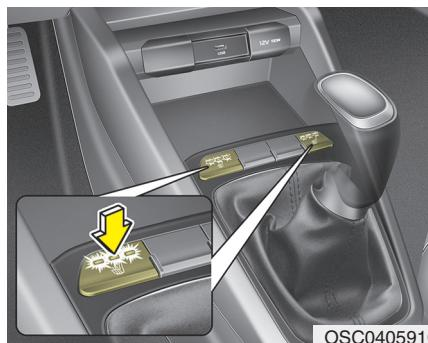
The seat warmer is provided to warm the front seats during cold weather. With the ignition switch in the ON position, push either of the switches to warm the driver's seat or the front passenger's seat.
