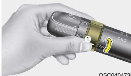
The fog lights will turn on when the fog light switch (1) is turned on after the parklight is turned on.
