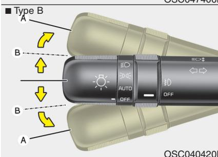
They will self-cancel after a turn is completed. If the indicator continues to flash after a turn, manually return the lever to the OFF position.
