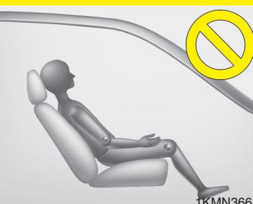
The driver must advise the passenger to keep the seatback in an upright position whenever the vehicle is in motion. If a seat is reclined during an accident, the restraint system's ability to restrain will be greatly reduced.
