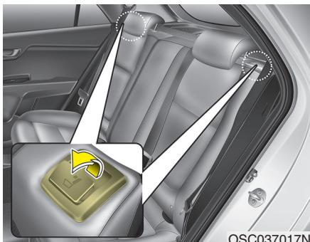
4. Pull the lock release lever and fold the rear seatback forward and down firmly.
