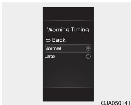
With the ignition switch or ENGINE START/STOP button in the ON position, select 'Driver Assistance' → 'Warning Timing' from the User Settings to change the initial warning activation time for Blind-Spot Safety system.
