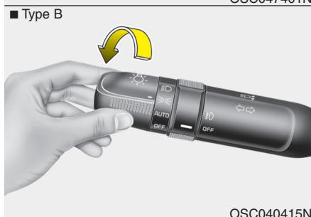
When the light switch is in the parking light position (3rd position), the tail, position, license and instrument panel lights will turn ON.
