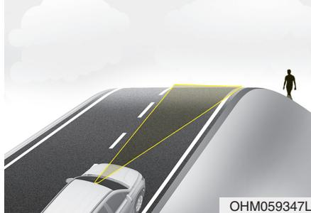
The performance of Forward Collision-Avoidance Assist may be decreased while driving upward or downward on a slope.
