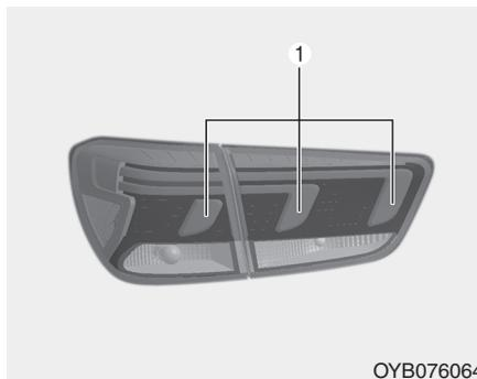
If the stop and tail lamp (LED) (1) does not operate, have the vehicle checked by an authorized Kia dealer. The LED lamps cannot be replaced as a single component because it is part of an integrated unit. The LED lamps have to be replaced with the unit.
