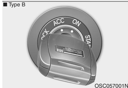
The anti-theft steering column lock is not a substitute for the parking brake. Before leaving the driver's seat, always make sure the shift lever is engaged in 1st gear for the Manual Transmission or P (Park) for the Intelligent Variable Transmission, set the parking brake fully and shut the engine off.
