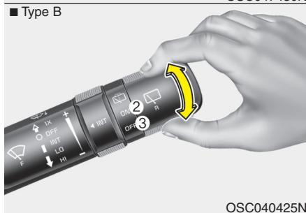
The rear window wiper and washer switch is located at the end of the wiper and washer switch lever. Turn the switch to operate the rear wiper and washer.
