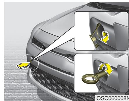
1. Remove the towing hook from the tool case located in the trunk/lift-gate.
