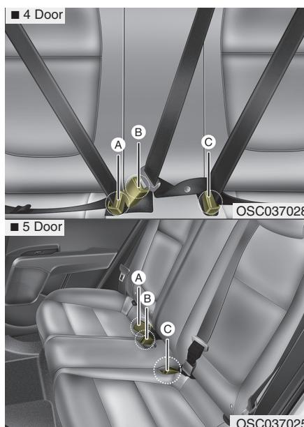
The seat belt should be locked into the buckle on each seat cushion to be properly fastened.
