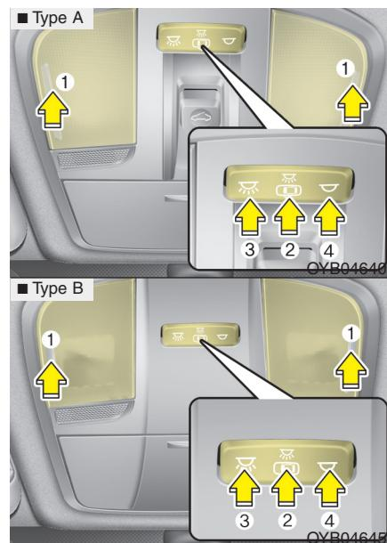
Push the lens (1) to turn the map lamp on or off. This light produces a spot beam for convenient use as a map lamp at night or as a personal lamp for the driver and front passenger.
