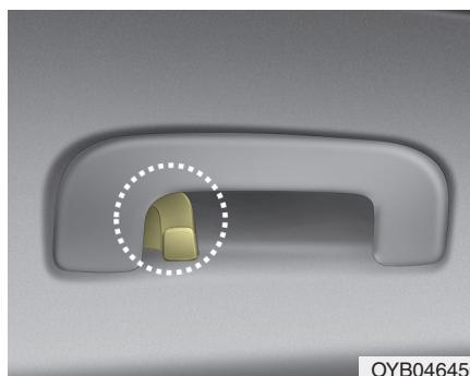
The clothes hanger is located on the roof of the rear seats.
