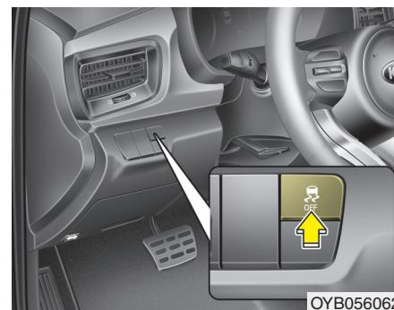
The Electronic Stability Control (ESC) system is designed to stabilize the vehicle during cornering maneuvers. ESC checks where you are steering and where the vehicle is actually going. ESC applies the brakes on individual wheels and intervenes with the engine management system to stabilize the vehicle.
