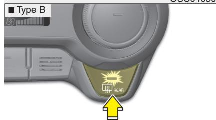
To activate the rear window defroster, press the rear window defroster button located in the center facia switch panel. The indicator on the rear window defroster button illuminates when the defroster is on.
