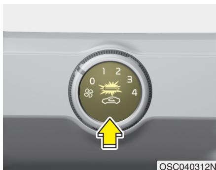
This is used to select outside (fresh) air position or recirculated air position. To change the air intake control position, push the control button.
