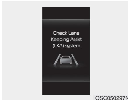
When Lane Keeping Assist is not working properly, the 'Check Lane Keeping Assist (LKA) system' warning message will appear and the yellow (/)\ indicator light will illuminate on the cluster. In this case, have your vehicle inspected by an authorized Kia dealer.
