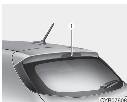
If the high mounted stop lamp (1) does not operate, have the vehicle checked by an authorized Kia dealer. A skilled technician should check or repair the high mounted stop lamp, for it may damage related parts of the vehicle.
