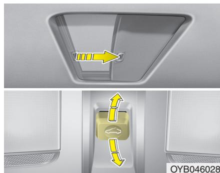
To open the sunroof to the maximum slide open position, press the switch towards the rear of the vehicle once again and hold it until the sunroof slides all the way open.
