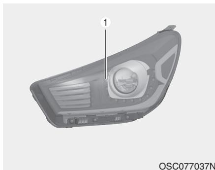
If the position lamp + DRL (LED) (1) does not operate, have the vehicle checked by an authorized Kia dealer. The LED lamps cannot be replaced as a single component because it is part of an integrated unit. The LED lamps have to be replaced with the unit.
