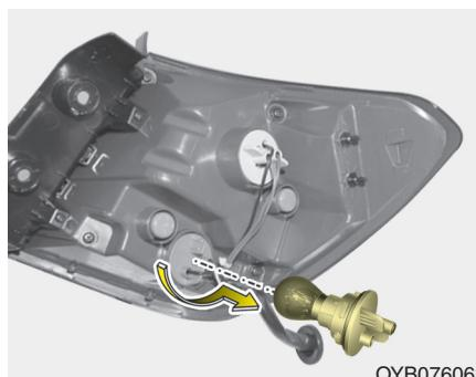
5. Remove the socket from the assembly by turning the socket counterclockwise until the tabs on the socket align with the slots on the assembly.
