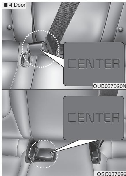
When using the rear center seat belt, the buckle with the "CENTER" mark must be used.
