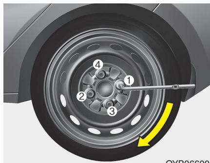
10. To install the wheel, hold it on the studs, put the wheel nuts on the studs and tighten them finger tight. Jiggle the tire to be sure it is completely seated, then tighten the nuts as much as possible with your fingers again.
