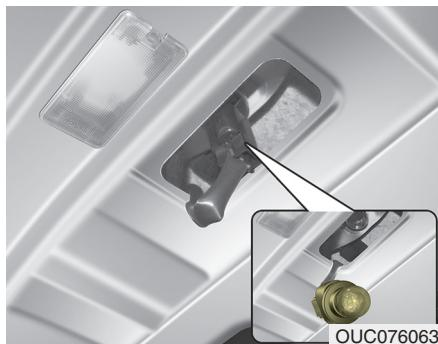
4. Insert a new bulb by inserting it into the bulb-socket.
