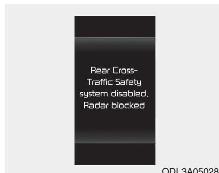
When the rear bumper around the rear-side radar or sensor is covered with foreign matters, such as snow or rain, or installing a trailer or carrier, it can reduce the detecting performance and temporarily limit or disable Rear Cross-Traffic Safety.
