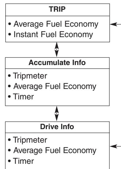
To change the trip mode, scroll the MOVE scroll switch ( $\wedge/\vee$ ) in the trip computer mode.
