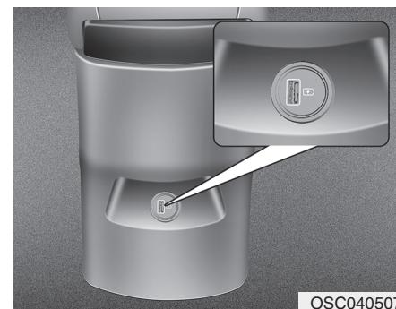
The USB charger is designed to recharge batteries of small size electrical devices using a USB cable. The electrical devices can be recharged when the ignition switch is in ACC/ON/START position.
