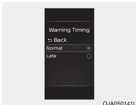
With the ignition switch or ENGINE START/STOP button in the ON position, select 'Driver Assistance → Warning Timing' from the User Settings menu to change the initial warning activation time for Rear Cross-Traffic Safety.
