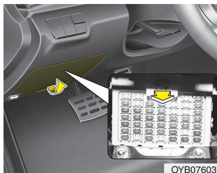
Your vehicle is equipped with the memory fuse to prevent battery discharge if your vehicle is parked without being operated for prolonged periods. Use the following procedures before parking the vehicle for prolonged periods.
