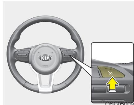
1. Press the Driving Assist (⌚) button on the steering wheel to turn the function on. The (⌚ CRUISE) indicator will illuminate.
