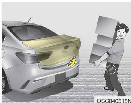
On a vehicle equipped with a smart key, the trunk can be opened with no-touch activation using the Smart Trunk Release system.
