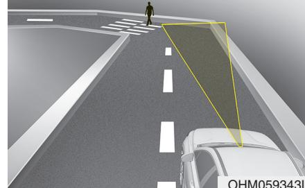
Forward Collision- Avoidance Assist may be limited when driving on a curved road.
