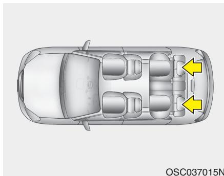
The rear seat is equipped with headrests in left and right side seating positions for the occupant's safety and comfort.
