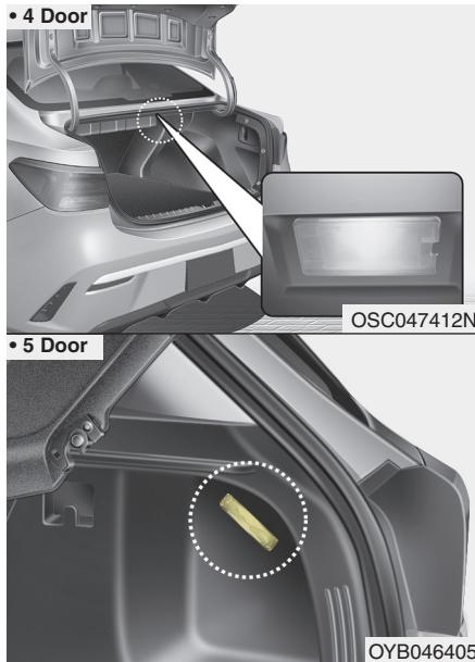
The trunk/liftgate room lamp comes on as long as the trunk/liftgate lid is open. To prevent unnecessary charging system drain, close the trunk/liftgate lid securely after using the trunk/liftgate room lamp.
