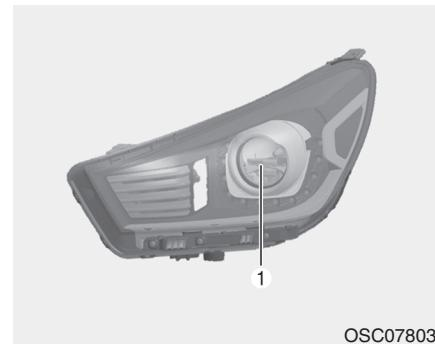
If the headlamp (Low/High beam) (1) does not operate, have the vehicle checked by an authorized Kia dealer.
