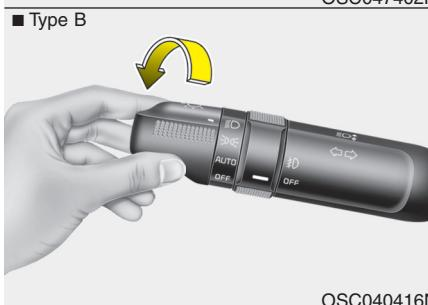
When the light switch is in the headlight position (4th position) the head, tail, position, license and instrument panel lights will turn ON.
