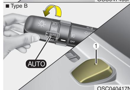
When the light switch is in the AUTO light position, the taillights and headlights will turn ON or OFF automatically depending on the amount of light outside the vehicle.
