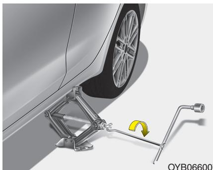
8. Insert the jack handle into the jack and turn it clockwise, raising the vehicle until the tire just clears the ground. This measurement is approximately 30 mm (1 in). Before removing the wheel lug nuts, make sure the vehicle is stable and that there is no chance for movement or slippage.
