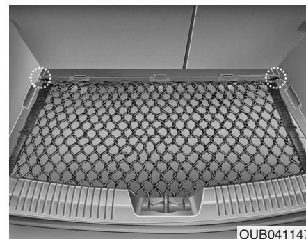
To keep items from shifting in the cargo area, you can use the 4 holders located in the cargo area to attach the luggage net (if equipped). If necessary, we recommend that you contact an authorized Kia dealer.
