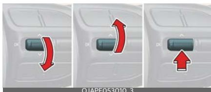
To resume Manual Speed Limit Assist after the function was paused, operate the (+), (-), (OK) switch.
