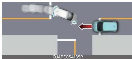
Junction Turning function can help avoid a collision with an oncoming vehicle, powered two-wheeler and cyclist in an adjacent lane when turning left (left-hand drive) or right (right-hand drive) at a crossroad with the turn signal on by applying emergency braking.
