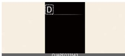
This indicator displays which Automated Manual Transmission shift lever is selected.
