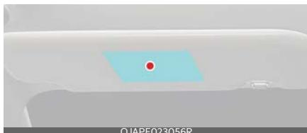
Air bag warning labels are attached to alert the driver and passengers of potential risk of air bag system.
