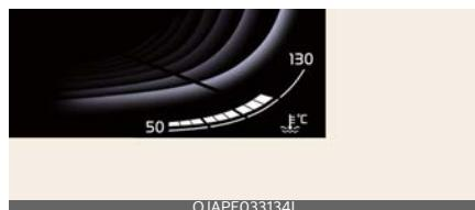
This gauge indicates the temperature of the engine coolant when the ignition switch or ENGINE START/STOP button is ON.
