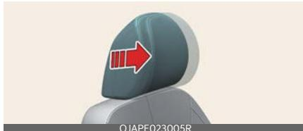
The headrest may be adjusted forward to 4 different positions by pulling the headrest forward to the desired detent. To adjust the headrest to its rearmost position, pull it fully forward to the foremost position and release it. Adjust the headrest so that it properly supports the head and neck.
