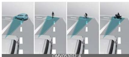
Forward Collision-Avoidance Assist may detect a vehicle, powered two-wheeler, pedestrian or cyclist in the next lane or outside the lane when driving on a curved road.
