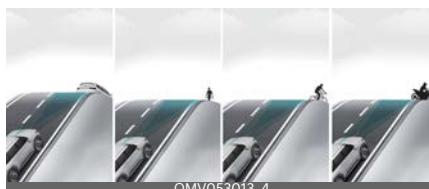
Forward Collision-Avoidance Assist may not detect other vehicle, powered two-wheeler, pedestrians or cyclists in front of you whilst driving uphill or downhill, adversely affecting the performance of the sensors.
