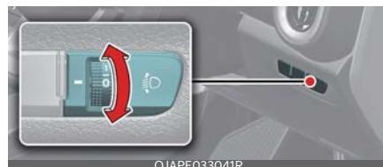
To adjust the headlight beam level according to the number of the passengers and loading weight in the luggage area, turn the beam levelling switch.
