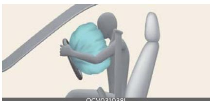
A fully inflated air bag, in combination with a properly worn seat belt, slows the driver's or the passenger's forward
