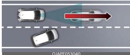
If the vehicle in front abruptly departs, Leading Vehicle Departure Alert may not operate properly.
