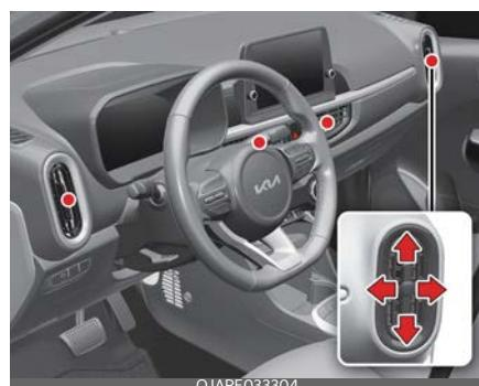
The outlet port can be opened or closed separately using the horizontal thumb-wheel. To close the vent, rotate it down-
