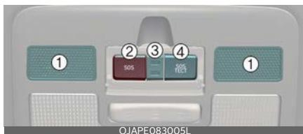
Elements of the system ERA-GLONASS, installed in passenger compartment:
