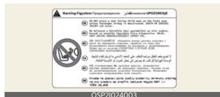
Never place a rear-facing child restraint in the front passenger's seat. If the air bag deploys, it would impact the rear-
