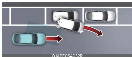
When you are driving forward out of a parking space, if Blind-Spot Collision-Avoidance Assist judges that there is a collision risk with an approaching vehicle in the blind spot, it can help avoid collision by applying the brake.
