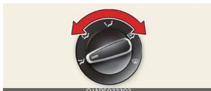
The mode selection knob controls the direction of the air flow through the ventilation system.
