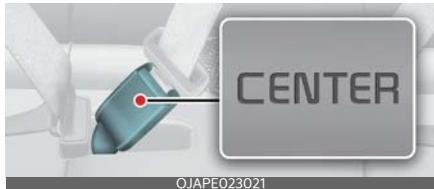
When using the rear centre seat belt, the buckle with the "CENTER" mark must be used.
