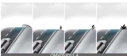
Forward Collision-Avoidance Assist may not detect other vehicles, powered two-wheelers, pedestrians or cyclists in front of you whilst driving uphill or downhill, adversely affecting the performance of the sensors.
