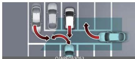
Rear Cross-Traffic Collision-Avoidance Assist may detect vehicles which are parking or pulling out near your vehicle (example, a vehicle leaving beside your vehicle, a vehicle parking
