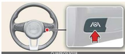
With the vehicle on, shortly press the Lane Driving Assist button located on the steering wheel to turn on Lane Following Assist. The grey or green (Ⓐ) indicator light will appear on the cluster.
