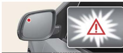
The warning light on the cluster, the outside rear view mirror will appear when the vehicle on both lanes is detected from the rear.
