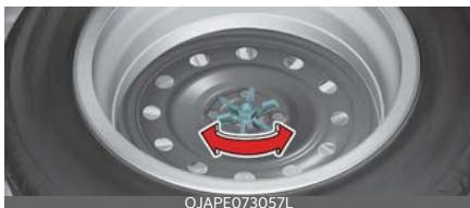
If it is hard to loosen the tyre hold-down wing bolt by hand, you can loosen it easily using the jack handle.
