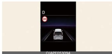
If you exceed the displayed speed limit, the sign will blink and an audible warning will be triggered.
