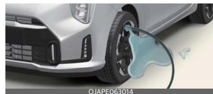
Securely install the sealant filling hose to the valve. If not, sealant may flow backward, possibly clogging the filling hose.
