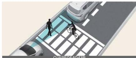
If there is a pedestrian(s) or bicycle(s) in between you and the vehicle in front, Leading Vehicle Departure Alert may not operate properly.
