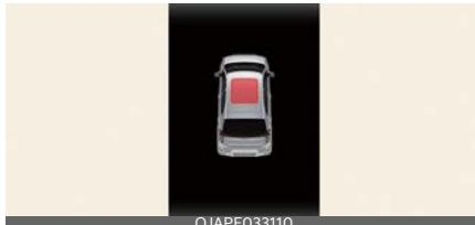
If the driver turns off the engine when the sunroof is not fully closed, the warning chime will sound for several seconds and the sunroof open warning will appear on the cluster LCD display. Close the sunroof securely when leaving your vehicle.
