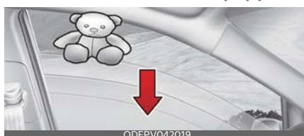
If the upward movement of the window is blocked by an object or part of the body, the window will detect the resistance and will stop upward movement. The window will then lower approximately 30 cm (11.8 in) to allow the object to be cleared.
