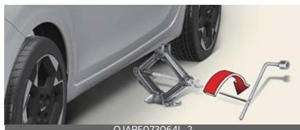
9. Loosen the wheel nuts and remove them with your fingers. Slide the wheel off the studs and lay it flat so it cannot roll away. To put the wheel on the hub, pick up the spare tyre, line up
