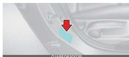
The vehicle certification label attached on the driver's (or front passenger's) side centre pillar gives the vehicle identification number (VIN).
