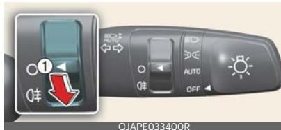
To turn the rear fog lights on, turn the rear fog light switch (1) to the on position when the headlight is turned on.
