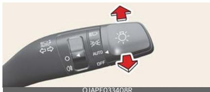
To turn on the high beam headlights, push the lever away from you when the headlight is on. Pull it back for low beams.
