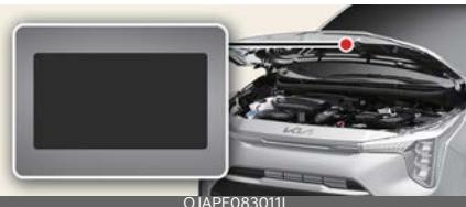
The refrigerant label is located on the underside of the bonnet.
