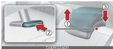
To raise the headrest, pull it up to the desired position (1). To lower the headrest, push and hold the release button (2) on the headrest support and lower the headrest to the desired position (3).
