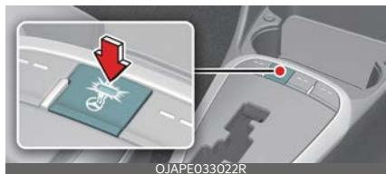
When the ignition switch is in the ON position, pressing the heated steering wheel button warms the steering wheel. The indicator on the button will illuminate.
