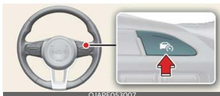
Press the Driving Assist button (OK) to turn Manual Speed Limit Assist off. The Speed Limit indicator (LIMIT) will go off.
