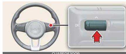
Press the (自然而) switch to temporarily pause the set speed limit. The set speed limit will turn off but the Speed Limit indicator (自然而) will stay on.
