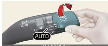
When the light switch is set to AUTO and vehicle is ON position, the light turns ON or OFF depending on the ambient brightness detected by the sensor.
