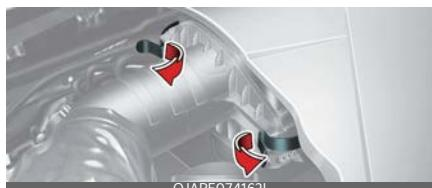
1. Loosen the air cleaner cover attaching clips and remove the air cleaner hose.
