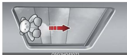
If the sunroof glass senses any obstacle whilst it is closing automatically, it will reverse direction then stop at a certain position.
