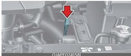
The automatic transmission fluid level should be checked regularly.
