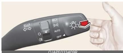
To flash the headlights, pull the lever towards you. It will return to the normal (low beam) position when released. The headlight switch does not need to be on to use this flashing feature.
