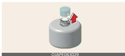
4. Rotate the sealant to mount it with the compressor.
