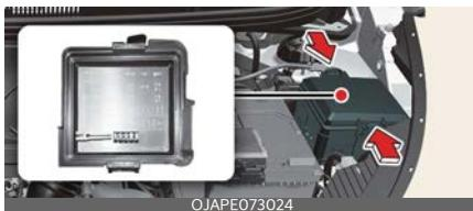
Inside the fuse/relay panel covers, you can find the fuse/relay label describing fuse/relay name and capacity.
