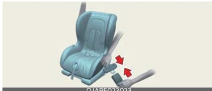
3. Remove as much slack from the belt as possible by pushing down on the Child Restraint System whilst feeding the shoulder belt back into the retractor.
