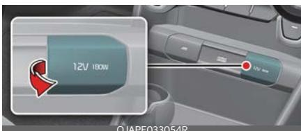
The power outlet is designed to provide power for mobile telephones or other devices designed to operate with vehicle electrical systems. The devices should draw less than 10 amps with the engine running.
