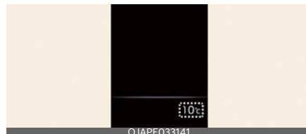
This gauge indicates the current outside air temperatures by 1°C (1°F).
