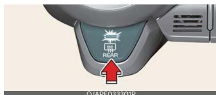
The defroster heats the window to remove frost, fog and thin ice from the rear window, whilst the engine is running.
