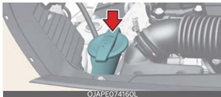
The reservoir is translucent so that you can check the level with a quick visual inspection.
