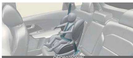
A forward-facing Child Restraint System provides restraint for the child's body with a harness. Keep children in a forward-facing Child Restraint System with a harness until they reach the top height or weight limit allowed by your Child Restraint System's manufacturer.
