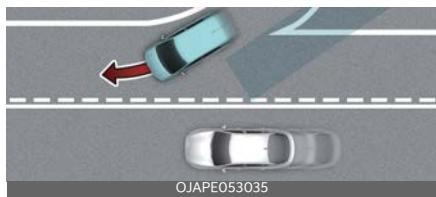
Blind-Spot Collision-Avoidance Assist may not operate properly when driving on a slope. The function may not detect the vehicle in the next lane or may incorrectly detect the ground or structure.
