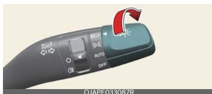
When the light switch is in the headlight position (4<sup>th</sup> position), the head, tail, position, license and instrument panel lights are ON.
