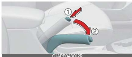
To release the parking brake, first apply the foot brake and pull up the parking brake lever slightly. Secondly depress the release button (1) and lower the parking brake lever (2) whilst holding the button.
