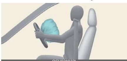
Upon deployment, tear seams molded directly into the pad covers will separate under pressure from the expansion of the air bags. Further opening of the covers then allows full inflation of the air bags.
