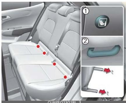
ISOFIX anchorages are located between the seatback and the seat cushion of the rear seat left and right outboard seating positions, indicated by the symbols.
