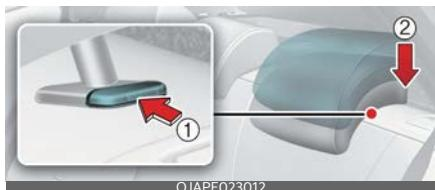
To remove the headrest, raise it as far as it can go then press the release button (1) whilst pulling upward (2).
