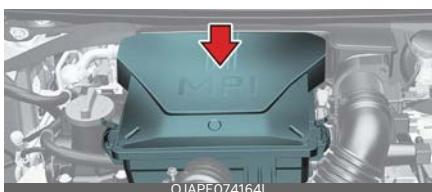
1. Loosen the air cleaner cover attaching clips.
