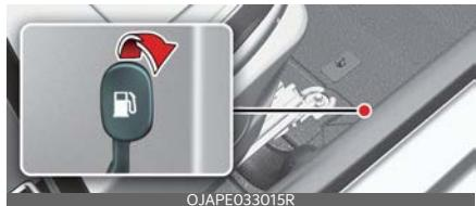
The fuel filler door must be opened from inside the vehicle by pulling up on the fuel-filler lid opener located on the front floor area on the driver's seat.
