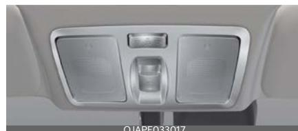
If your vehicle is equipped with a sunroof, you can slide or tilt your sunroof with the sunroof switch located on the overhead console.
