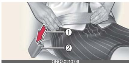
With a 2-point static type seat belt, the length must be adjusted manually so it fits snugly around your body. Fasten the belt and pull on the loose end to tighten.
