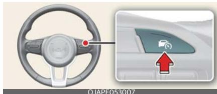
2. Push the (+) switch up or (-) switch down, and release it at the desired speed.
