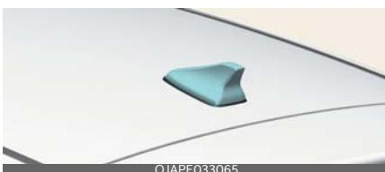
The shark fin antenna will receive the transmit data.
