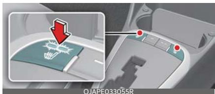
The seat warmer is provided to warm the front seats during cold weather. With the ignition switch in the ON position, push either of the switches to warm the driver's seat or the front passenger's seat.
