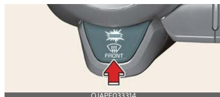
When you select the defrost mode, the following system settings will be made automatically:
