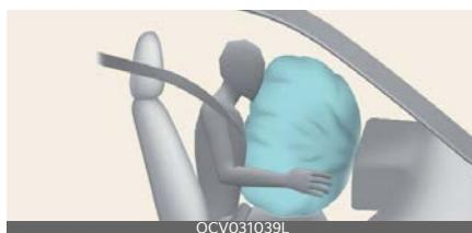
After complete inflation, the air bag immediately starts deflating, enabling the driver to maintain forward visibility and the ability to steer or operate other controls.
