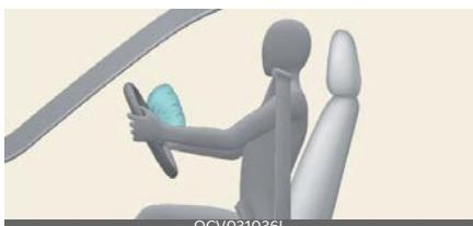
The air bag modules are located both in the centre of the steering wheel and in the front passenger's panel above the glove box. When the SRSCM detects a sufficiently severe impact to the front of the vehicle, it will automatically deploy the front air bags.
