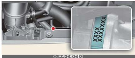
The engine number is stamped on the engine block as shown in the drawing.
