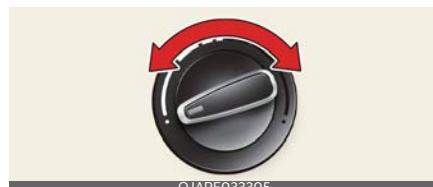
The temperature control knob allows you to control the temperature of the air flowing from the ventilation system. To change the air temperature in the passenger compartment, turn the knob to the right position for warm and hot air or left position for cooler air.
