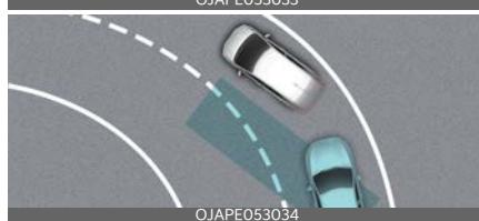
Blind-Spot Collision-Avoidance Assist may not operate properly when driving on a curved road. Blind-Spot Collision-Avoidance Assist may not detect the vehicle in the next lane.
