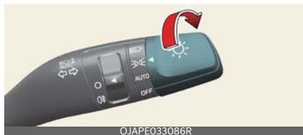
When the light switch is in the parking light position (3<sup>rd</sup> position), the tail position, license and instrument panel lights will turn ON.
