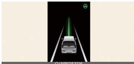
If the vehicle ahead and/or both lane markings are detected and Your driving speed is below 160 km/h (100 mph), the green (Ⓐ) indicator light appears on the cluster, and Lane Following Assist helps centre the vehicle in the lane by assisting the steering wheel.
