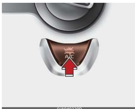
Press the A/C button to turn the air conditioning system on (indicator light will illuminate). Press the button again to turn the air conditioning system off.
