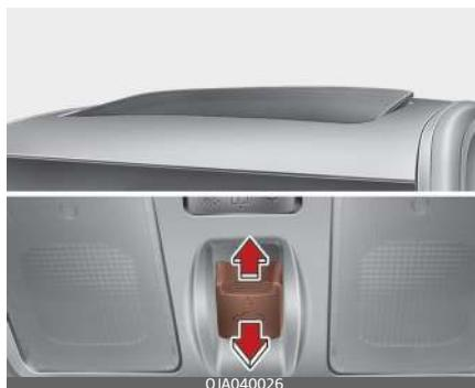
To open the sunroof, push the sunroof control lever upward until the sunroof moves to the desired position.
