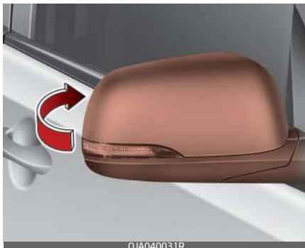
To fold outside rearview mirror, grasp the housing of mirror and then fold it toward the rear of the vehicle.
