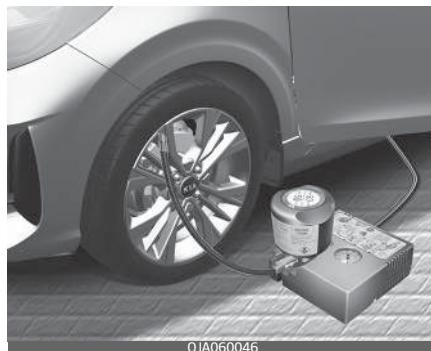
The system of compressor and sealing compound effectively and comfortably seals most punctures in a passenger car tyre caused by nails or similar objects and reinflates the tyre.
