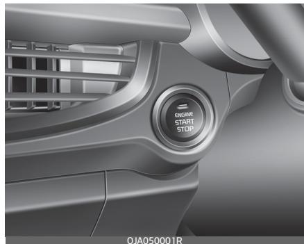
Whenever the front door is opened, the ENGINE START/STOP button will illuminate for your convenience. The light will go off after about 30 seconds when the door is closed. It will also go off immediately when the theft-alarm system is armed.
