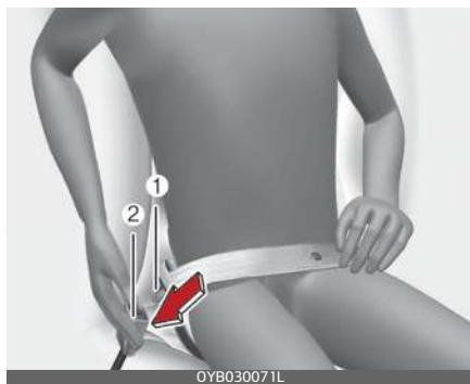
With a 2-point static type seat belt, the length must be adjusted manually so it fits snugly around your body. Fasten the belt and pull on the loose end to tighten.
