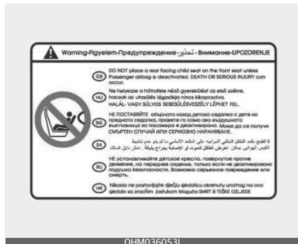
Never place a rear-facing child restraint in the front passenger's seat. If the air bag deploys, it would impact the rear-facing child.
