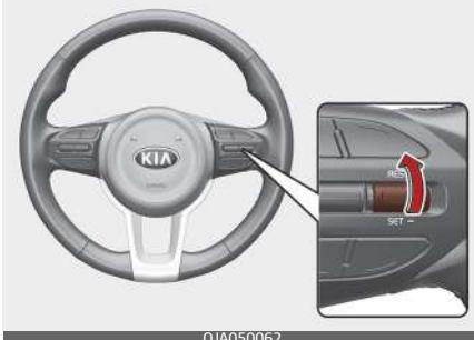
To resume Manual Speed Limit Assist after the function was paused, push the RES+, RES- switch.
