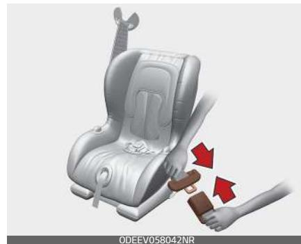
3. Remove as much slack from the belt as possible by pushing down on the Child Restraint System whilst feeding the shoulder belt back into the retractor.
