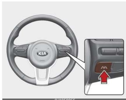
To activate/deactivate LKA, with the ignition switch or ENGINE START/STOP button in the ON position, press and hold the Lane Driving Assist button (/ $\textcircled{A}$ \) located on the steering wheel to turn off Lane Keeping Assist. Press and hold the button again to turn on the function.
