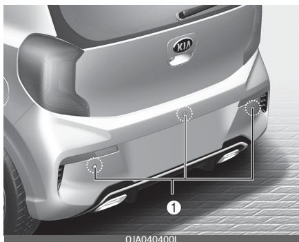
Reverse Parking Distance Warning assists the driver during backward movement of the vehicle by chiming if any object is sensed within a distance of 120 cm (48 in.) behind the vehicle.
