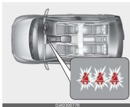
As a reminder to the rear seat belt, the rear seat belt warning lights will illuminate for approximately 6 seconds each time you turn the ignition switch ON regardless of belt fastening.
