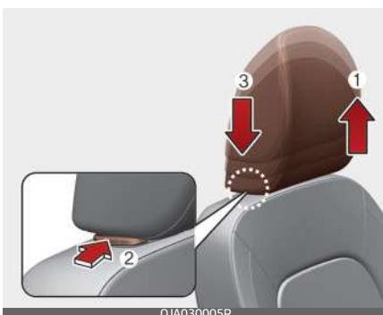
To raise the headrest, pull it up to the desired position (1). To lower the headrest, push and hold the
