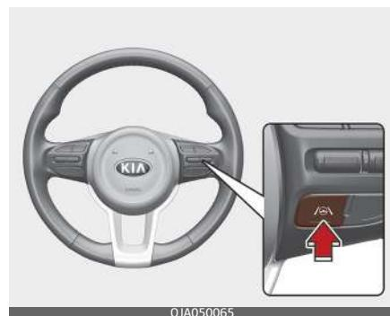
With the ignition switch or the ENGINE START/STOP button in the ON position, press the Lane Driving Assist button located on the steering wheel to turn on Lane Following Assist. The white or green (Ⓐ) indicator light will illuminate on the cluster.
