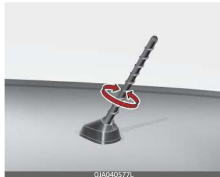
Your car uses a roof antenna to receive both AM and FM broadcast signals. This antenna is a removable type.
