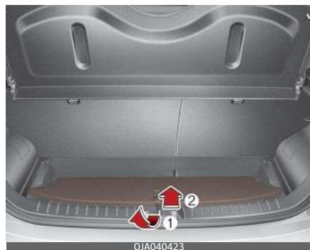
3. Pull the luggage board hinge to the end of sliding slot and it will fall down lower to increase cargo space.
