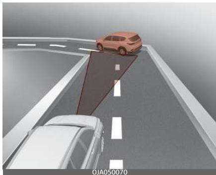
Forward Collision-Avoidance Assist may detect a vehicle in the next lane or outside the lane when driving on a curved road. If this occurs, the unnecessarily alarm the driver and apply the brake.
