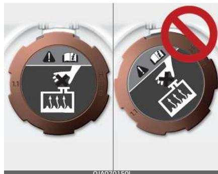
2. Make sure that the tiny protrusions inside the coolant cap should be securely interlocked.
