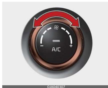
The fan speed can be set to the desired speed by operating the fan speed control knob.
