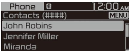
Press the [MENU] button on the control panel to access the following a menu option:
