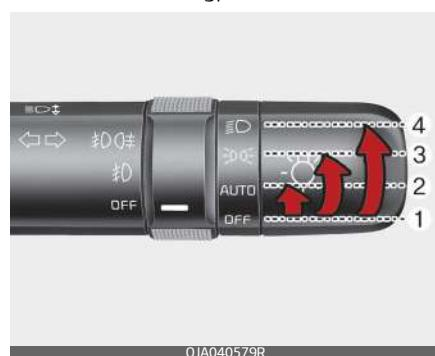
The light switch has a Headlight and a Parking light position.
