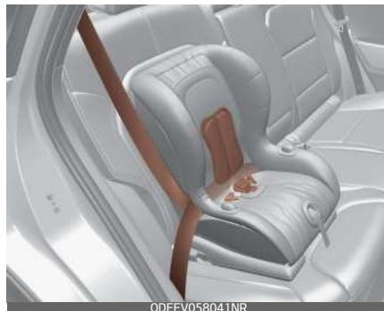
2. Fasten the lap/shoulder belt latch into the buckle. Listen for the distinct "click" sound. Position the release button so that it is easy to access in case of an emergency.
