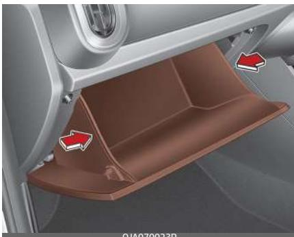
2. Remove the climate control air filter cover whilst pressing the lock on the left side of the cover.
