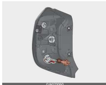
7. Insert a new bulb by inserting it into the socket and rotating it until it locks into place.
