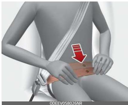
The seat belt should be locked into the buckle on each seat cushion to be properly fastened.
