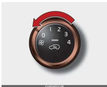
To turn off the blowers, turn the fan speed control knob to the "0" position.
