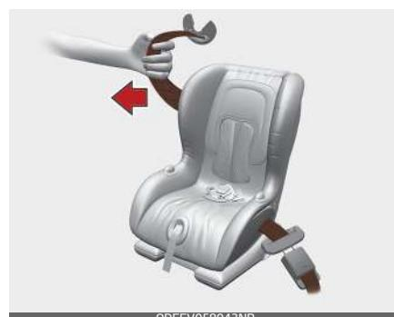
If your Child Restraint System manufacturer recommends the use of a top-tether with the lap/shoulder belt.
