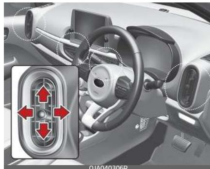
The outlet port can be opened or closed separately using the horizontal thumbwheel. To close the vent, rotate it downward to the maximum position. To open the vent, rotate it upward to the desired position.
