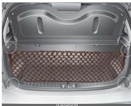
To keep items from shifting in the cargo area, you can use the 2 holders located in the cargo area to attach the luggage net.
