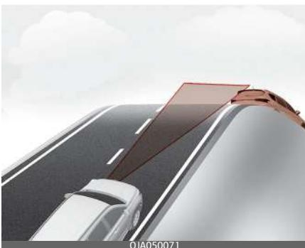
Forward Collision-Avoidance Assist may not detect other vehicles in front of you whilst driving uphill or downhill adversely affecting the performance of the sensors.
