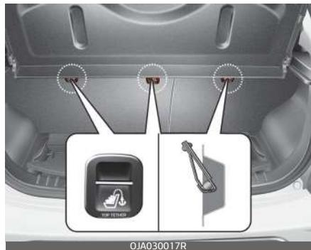
1. Route the Child Restraint System top-tether strap over the seat-back. Placing the top tether strap, please follow the instructions of the Child Restraint System manufacturer.
