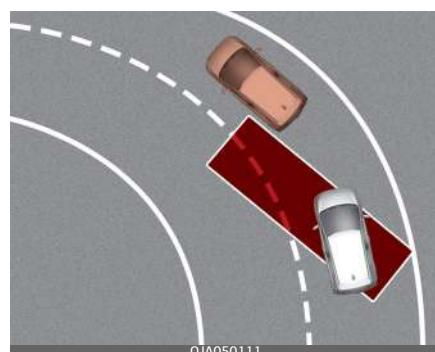
Blind-Spot Safety system may not operate properly when driving on the curved road. The function may recognize the vehicle in the same lane.
