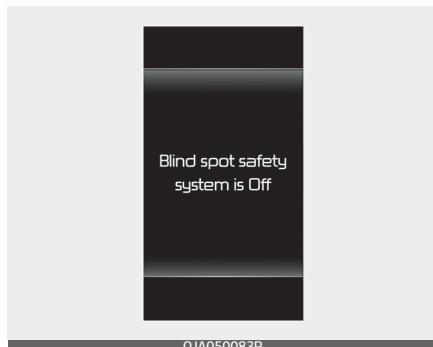
When the engine is restarted with the function off, the 'Blind-spot safety system is Off' message will appear on the cluster.
