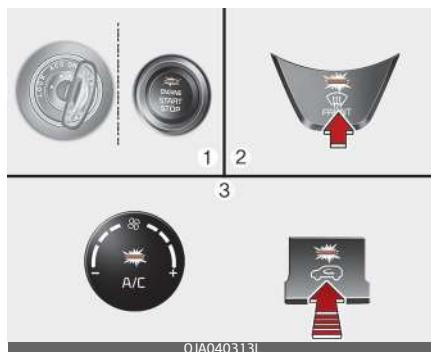
The air intake control button indicator blinks 3 times. It indicates that the defogging logic is cancelled or returned to the programmed status.
