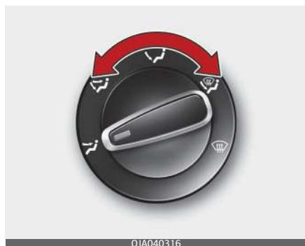
The mode selection knob controls the direction of the air flow through the ventilation system.
