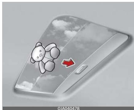
If an object or part of the body is detected whilst the sunroof is closing automatically, it will reverse the direction, and then stop.
