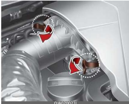
1. Loosen the air cleaner cover attaching clips and remove the air cleaner hose.
