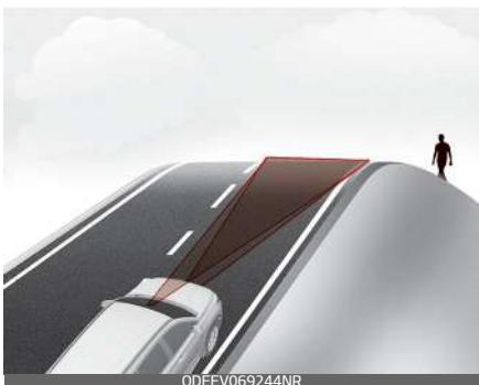
Forward Collision-Avoidance Assist may not detect other vehicles or pedestrians in front of you whilst driving uphill or downhill adversely affecting the performance of the sensors.
