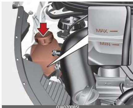
If the coolant level is low, add enough distilled (deionized) or soft water. Bring the level to MAX, but do not overfill.
