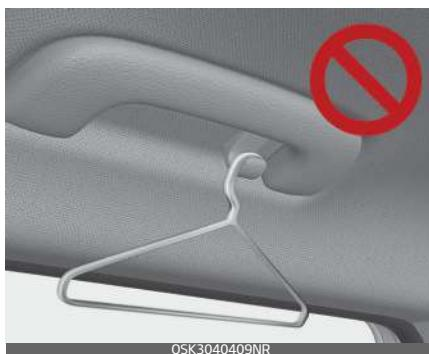
Do not hang other objects such as hangers or hard objects except clothes. Also, do not put heavy, sharp or breakable objects in the clothe pockets. In an accident or when the curtain air bag is inflated, it may cause vehicle damage or personal injury.
