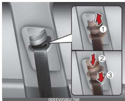
Release the button to lock the anchor into position. Try sliding the height adjuster to make sure that it has locked into position.
